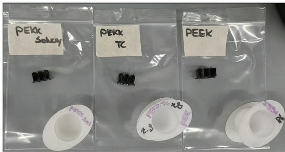
Figure 3.2: Photograph of UD samples in sample holder before embedding
