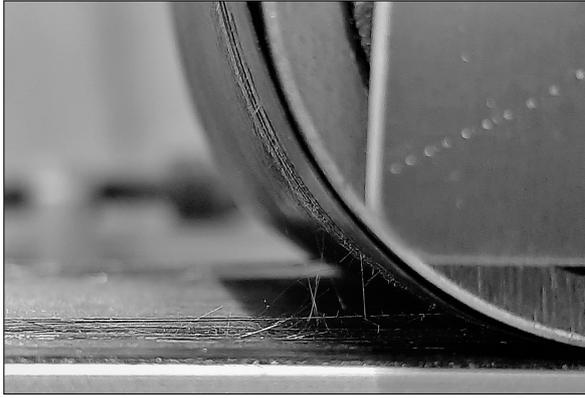
Figure 4.11: Photograph showing the presence of fibre bridging during the MP test at the front side of the mandrel
