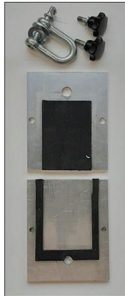
Figure 4.5: Photograph of UD tape fixture
