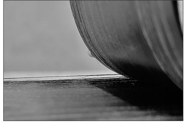
Figure 4.12: Photo showing the presence of fibre pull-out during the MP test at the back side of the mandrel
