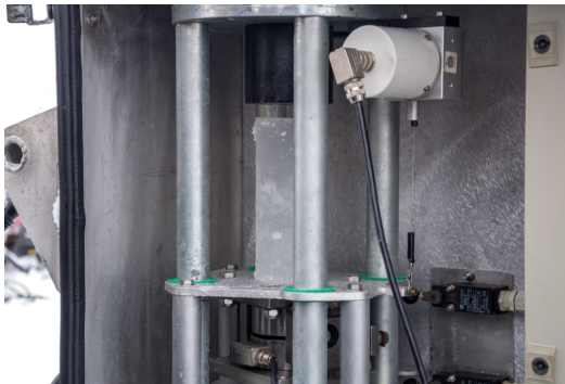
Figure 2.7: Uni-axial compression test on sea ice near Svea, Svalbard
