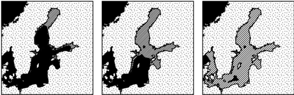
Figure 1.1: Ice cover in the Baltic Sea. From left to right: a mild, an average, and an extreme winter (ISO 19906, 2010)
