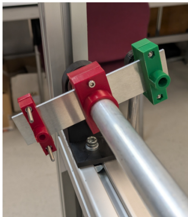
Figure A.8: Iteration 3: aluminum plate joint detail (left) and complete setup mounted on extrusion profiles (right).
