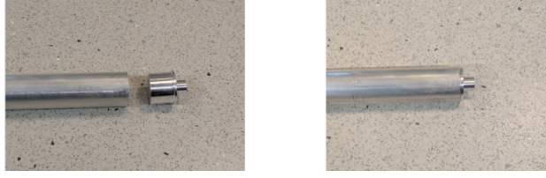
Figure A.17: Hollow torsion rod tube with solid aluminum insert prior to bonding (left). Assembled torsion rod with insert seated in the steel roller bearing (right).
