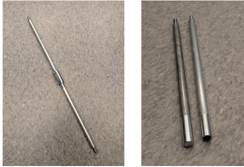
Figure A.15: Assembled pushrod with shaft coupling (left). Solid and hollow pushrod variants shown for comparison (right); the hollow variant was selected for the final prototype.
