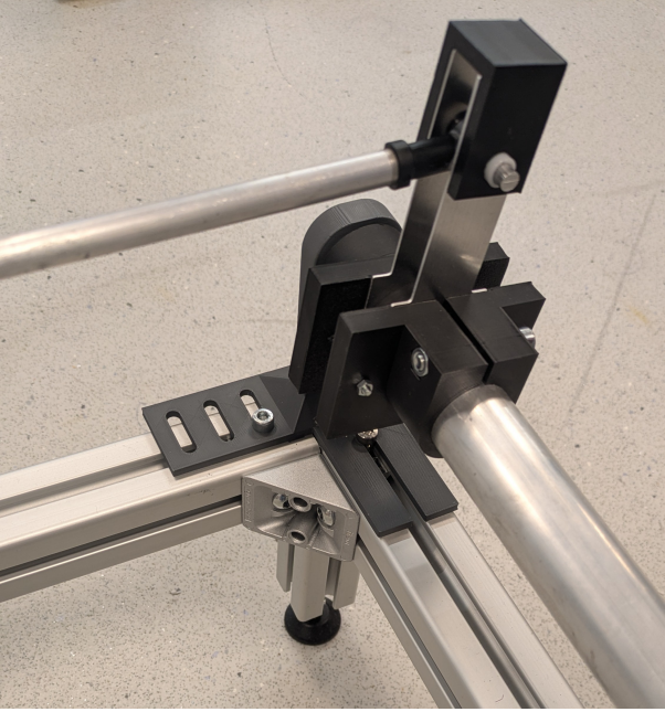
Fig. 6: 3D-printed bearing housing supporting the torsion rod. The housing is fastened to the aluminum extrusion frame with steel bolts.
