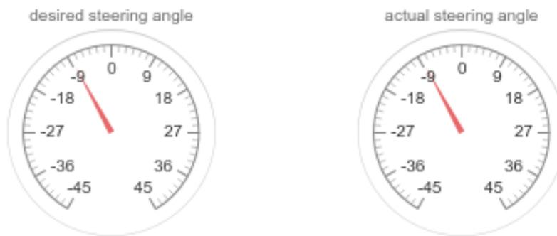
**Figure 4-6:** Driver instructions in 2D world simulation. (Left: Steering instruction  $\delta_d$ . Right: Steering input from driver  $\delta$ .)
