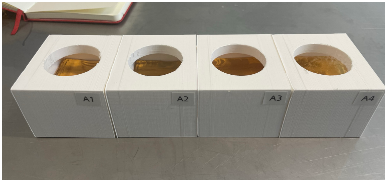
Figure 89: Four prototypes to determine the best fitting part for the cervix and vagina wall toughness.
