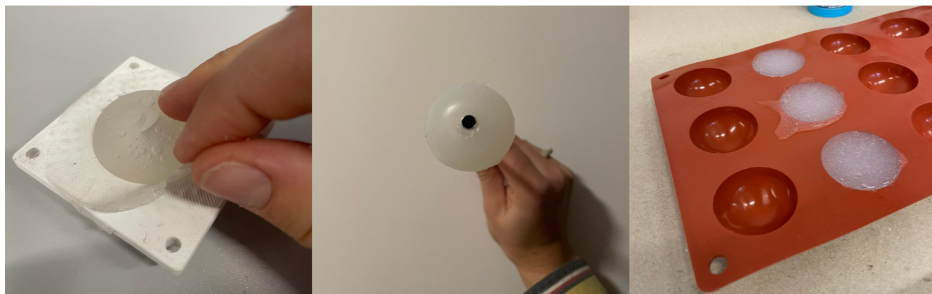
Figure 92: First casting trial and Dragon Skin models without possibility of fixing on outer part.
