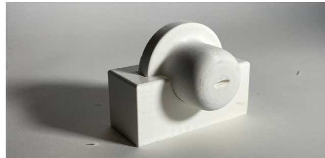
Figure 34: 3D printed cervix model, with the best potential for the demonstration device.
