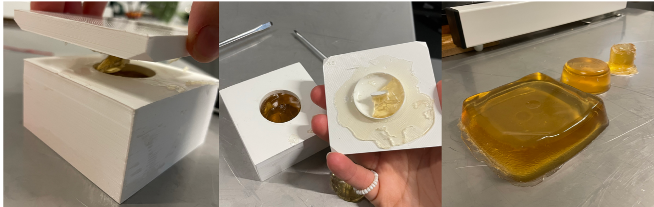
Figure 88: Two molded cervix design (poor unloading material), with other working cervix designs.
