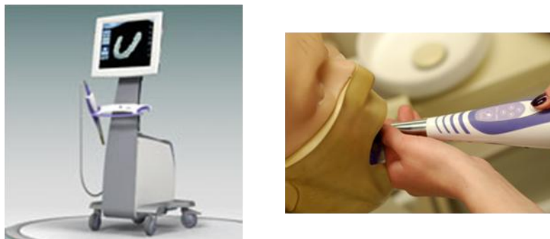
Figure 2 3M Lava™ Chairside Oral Scanner (left) and an oral scanning with 3M oral scanner on a phantom head
