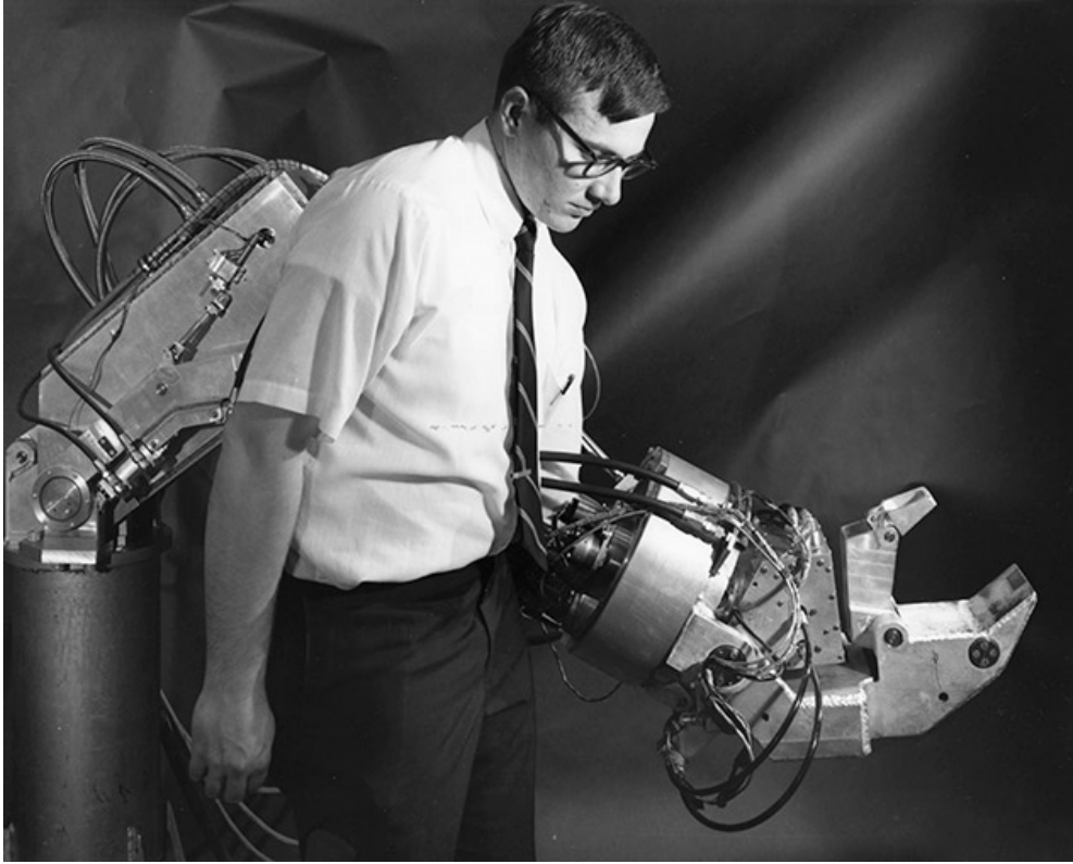
Figure 2.3: Arm module of the Hardiman powered exoskeleton (Croshaw, 1969), representing the role of an orthosis to augment human strength.
