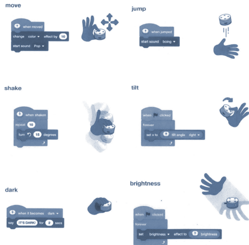
Fig. (3.5.2) Scratchbit mini-card examples showing home custom gestures of the blended learning object could be encoded
