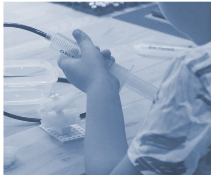
Fig. (3.1.4 c) It was still difficult to hand hold the syringes thus creating a need for a separate syringe pumping unit as shown
