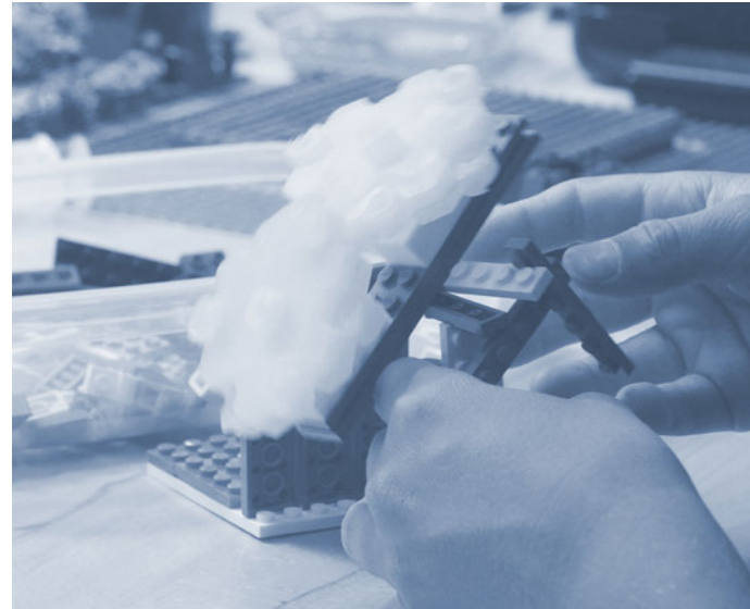
Fig. (3.1.4 a) Using the LEGO based connectors to integrate into the LEGO ecosystem with the soft actuator blocks
