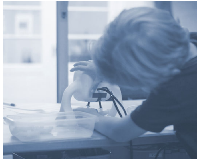
Fig. (3.1.6 b) Customising the body movement by connecting the soft modular blocks to bending restrictors
