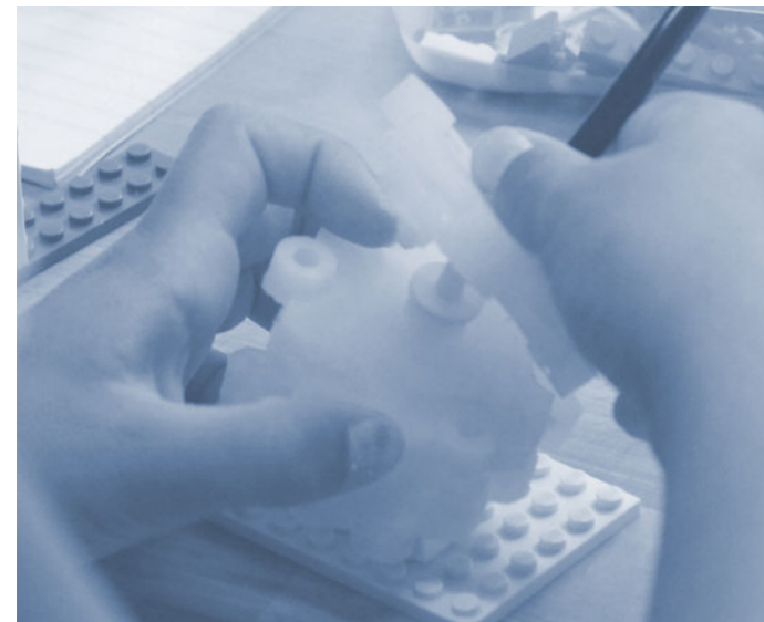
Fig. (3.1.4 b) The interconnectors were much more easier to combine the soft actuator blocks together
