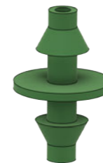
Fig. (D.4 b) Final selected interconnector making it both easy to pull, push and also being airtight at the same time.
