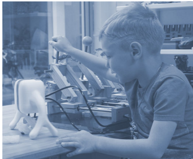
Fig. (3.1.6 d) The vinyl tube length was causing interference in the motion of the Silly Stompers which could be improvised
