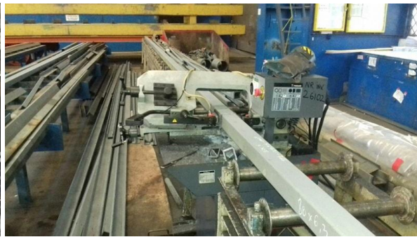
(b) Cutting machine S1a-L1- sawing-machine
