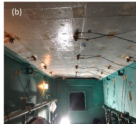
Fig. 13. (a) Tested highway bridge, (b) sensor arrangement for the measurement before repair.
