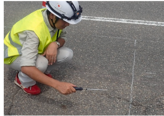
Fig. 11. (a) Analysis model for AE tomography, (b) steel-ball tapping (Okude et al., 2018).
