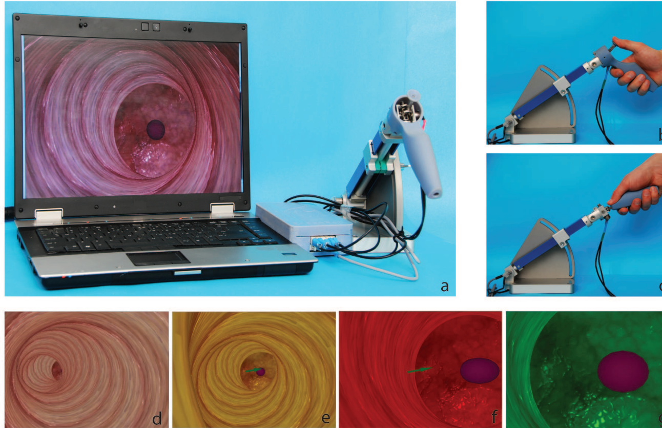
Figure 5.3: Endo-PaC hardware and software units. a) the Endo-PaC setup, b) thumb control, c) wrist control, screenshots of the animation program in case of d) normal e) warning for near collision, f) collision, g) success. The green arrow appears only in the case of near collision or collision. The direction and length of green arrow is proportional to the position of the warning/collision and deviation to the tunnel central line.
