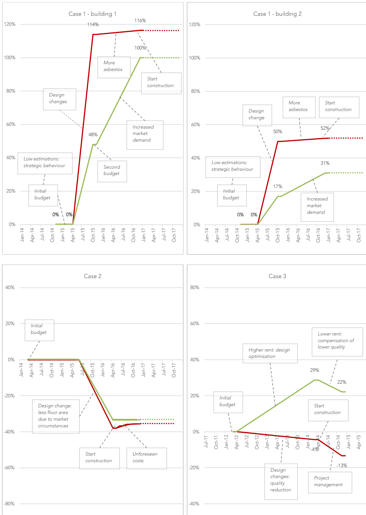
Figure 1: Cross-case analysis, classified on the development duration, key moments in the process and the main reasons for deviations in relation to the development of construction costs (red) and rental income per year (green)
