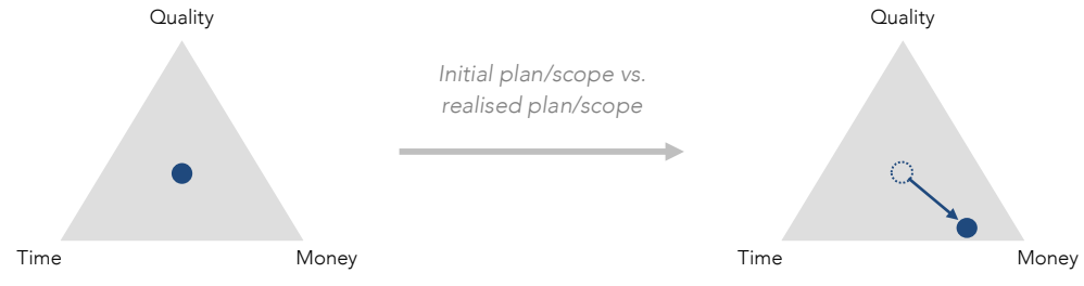
Figure 33: Change in scope/plan decreased the quality and total GFA, but came with lower costs (schematic)
