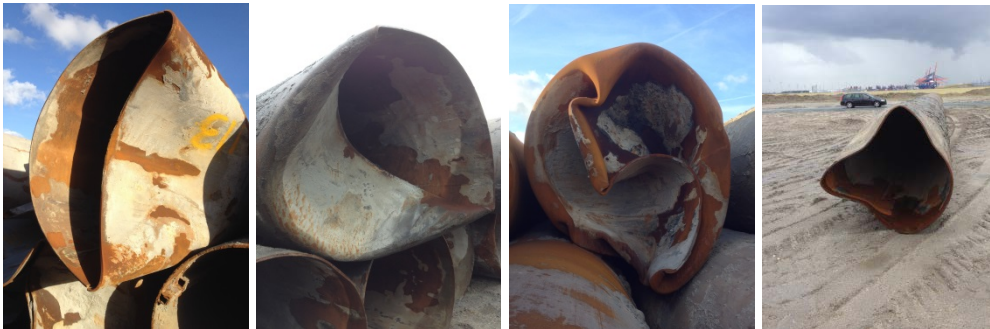
Figure 8: Pile toe damages
