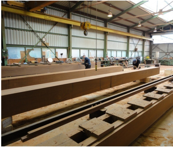
Figure 17: Work done by hand on posts
