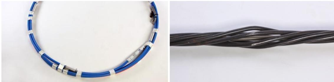
Figure 70: MPBX (left) and SMART Cable (right). (Mine Design Technologies, 2013)
