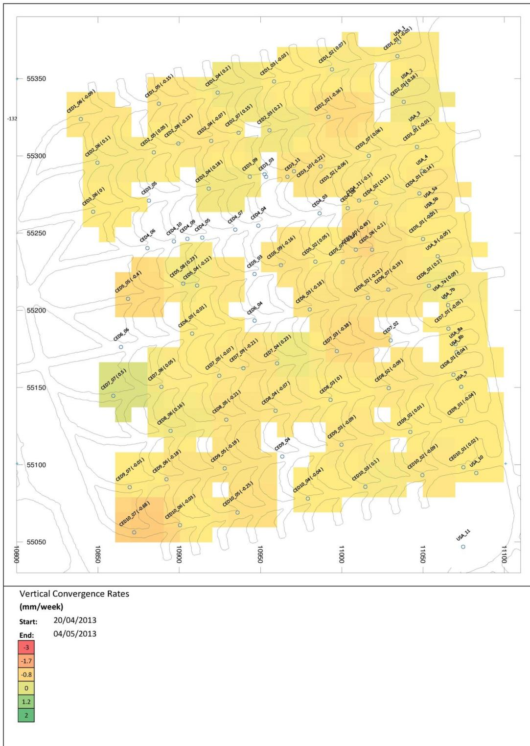
Figure 79: Example of an Extraction Level plan with convergence stations and colour coding to indicate weekly convergence rates.
