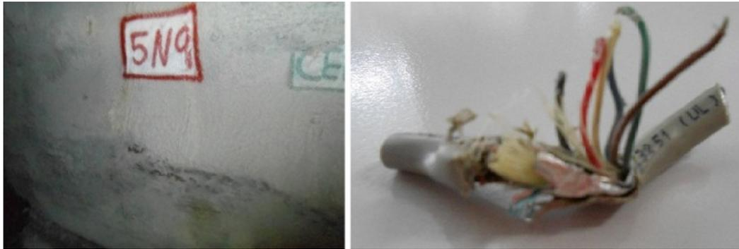
Figure 72: Scrape marks of an LHD on the camelback of the pillar next to drawpoint 5N9 (left) and an example of a resulting breakage in the leadwires (right). This particular section of leadwire was taken at station EXT-02S03-HM.
