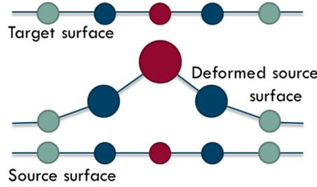
**FIGURE 33.2** Schematic representation of elasticity. If one vertex, in this case, the *red dot* (gray in print version) is transformed; the neighboring vertices are forced to move along with this vertex. The closest neighbors (*blue dots*) (dark gray in print version) are the stiffest and move more than the distant neighbors (*green dots*) (light gray in print version).
