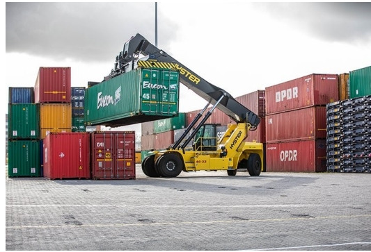
Figure 4.4: A reach stacker stacking containers (Hyster, 2022)
