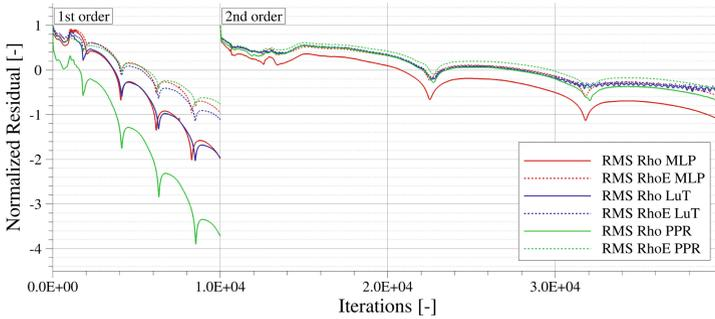
**Fig. 5.** Normalized density and energy residuals for the 1st and 2nd order simulations performed with the three investigated fluid models. The case featuring the PPR EoS reached the lowest absolute density residual.
