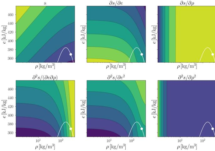
**Fig. 1.** Trends of the entropy potential, its first and its second-order derivatives with respect to density and internal energy. The white line identifies the saturation curve, while the white dot corresponds to the critical point. The range of density has been extended up to  $405 \text{ kg/m}^3$  for visualization purposes.
