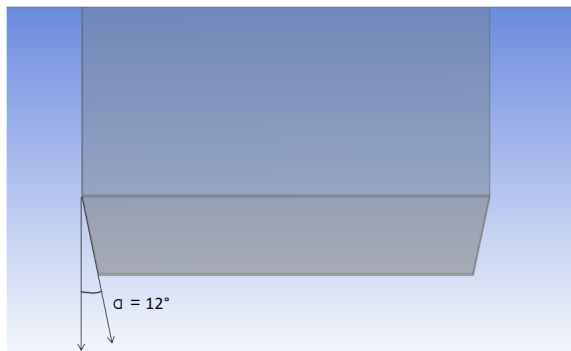
Figure 3.46: Top panel of the attached boat-tail (top view)
