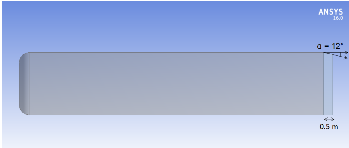
Figure 3.45: Modified GETS model with the boat-tail attached (side view)
