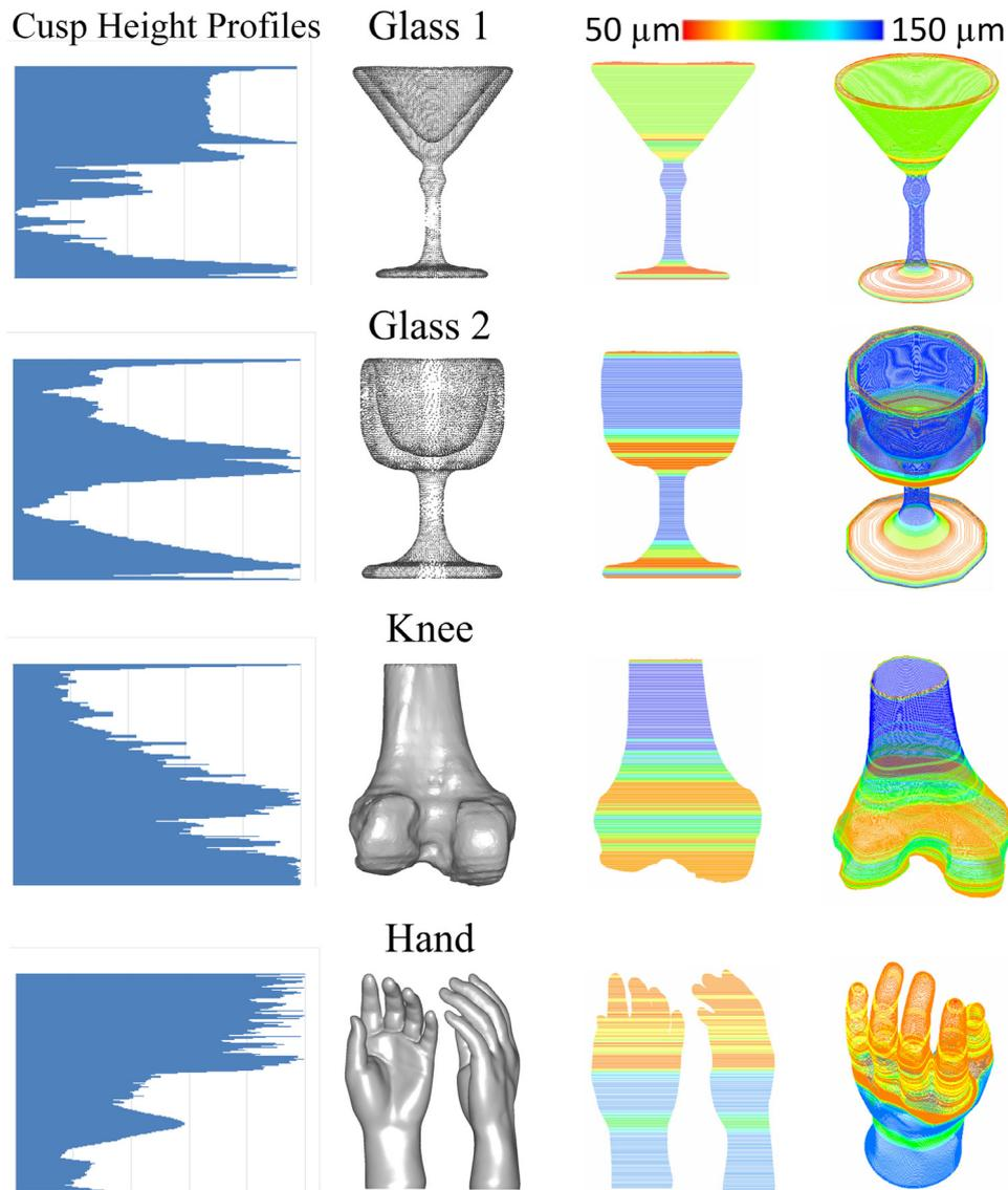
Fig. 9. Adaptive slicing results of various models.
