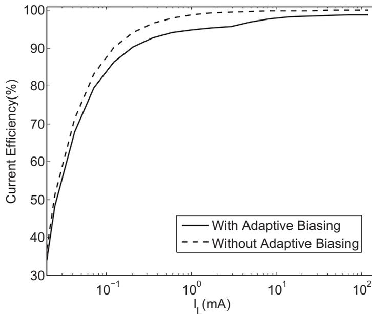
Figure 4.3: Current efficiency ( $V_{BAT}=12\text{V}$ , typical process corner, temp= $27^\circ\text{C}$ ).
