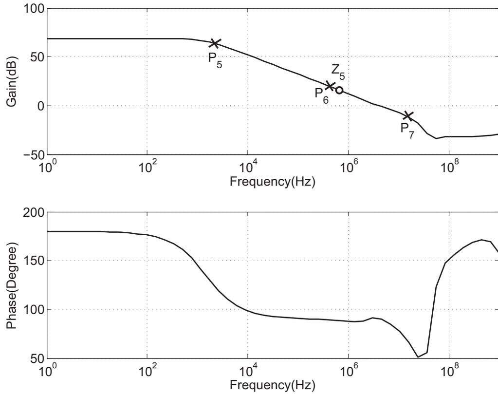
Figure 3.20: Current sensing loop bode plot at  $I_L=120\text{mA}$ .
