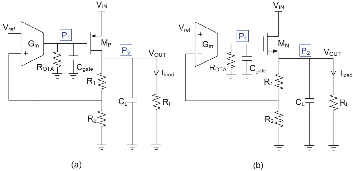
Figure 2.11: A simple topology of (a) PMOS regulator (b) NMOS regulator.
