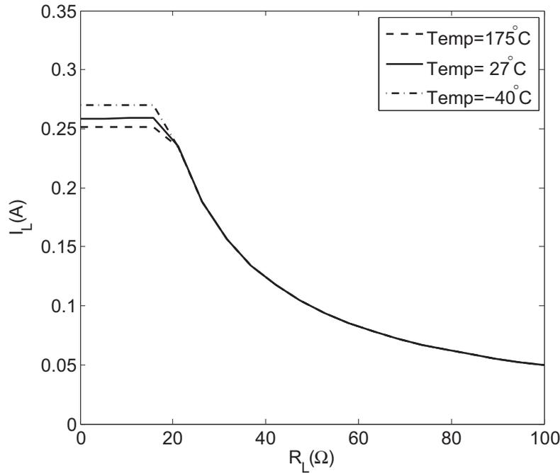
Figure 4.17:  $I_L$  versus  $R_L$  ( $V_{BAT}=12V$ , typical process corner).
