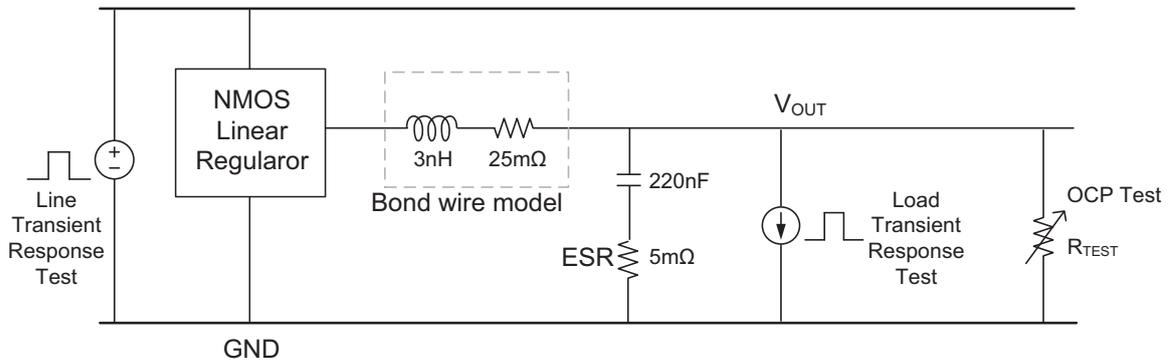
Figure D.1: Test-benches.
