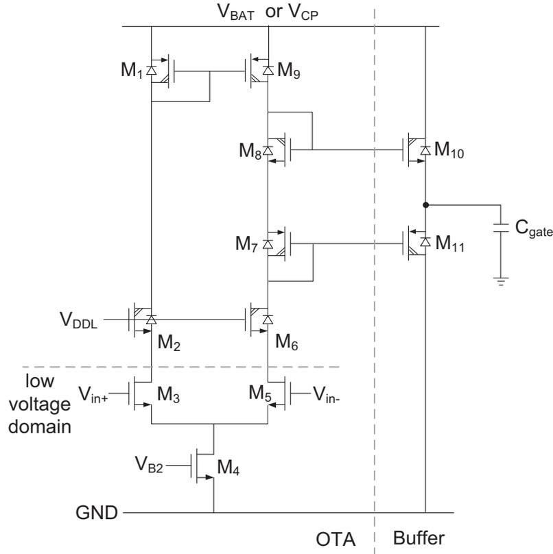
Figure 3.3: High voltage operational amplifier with cascode low voltage input pair.
