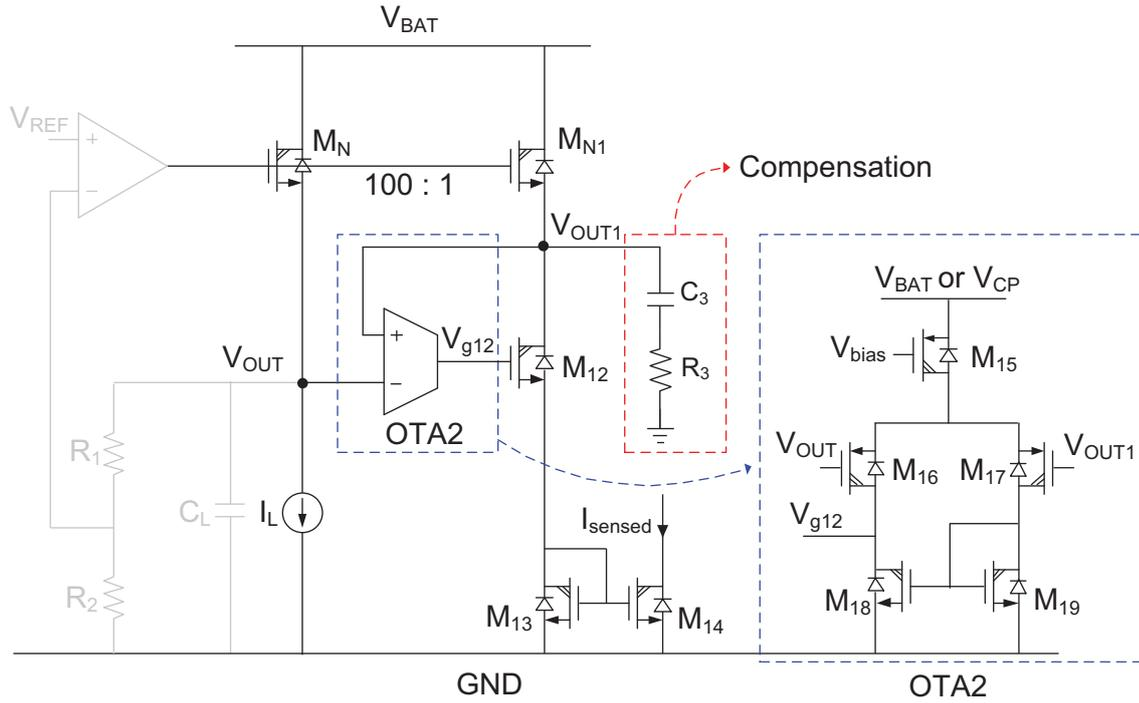
Figure 3.17: Current sensing scheme with regulated source node voltage.
