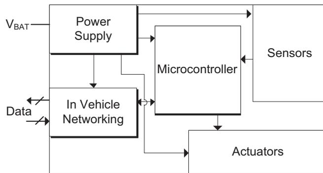
Figure 1.2: A typical ECU diagram.
