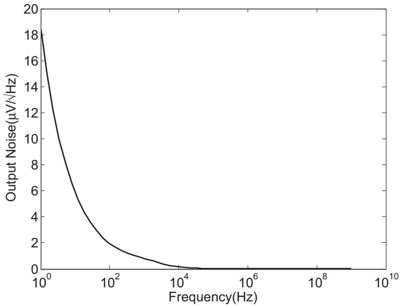
Figure 4.16: Output noise ( $I_L=20mA$ , typical process corner,  $27^\circ C$ ).
