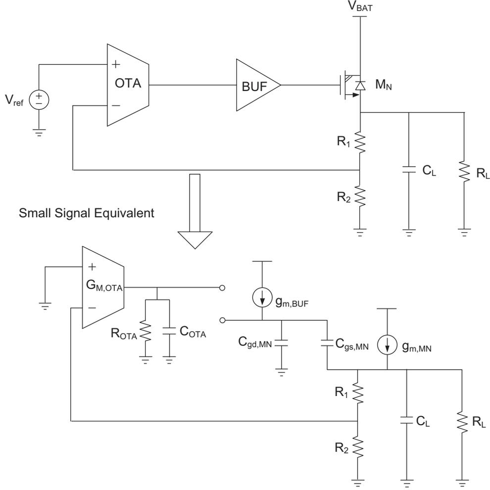
Figure 3.4: Small signal equivalent of NMOS linear regulator.
