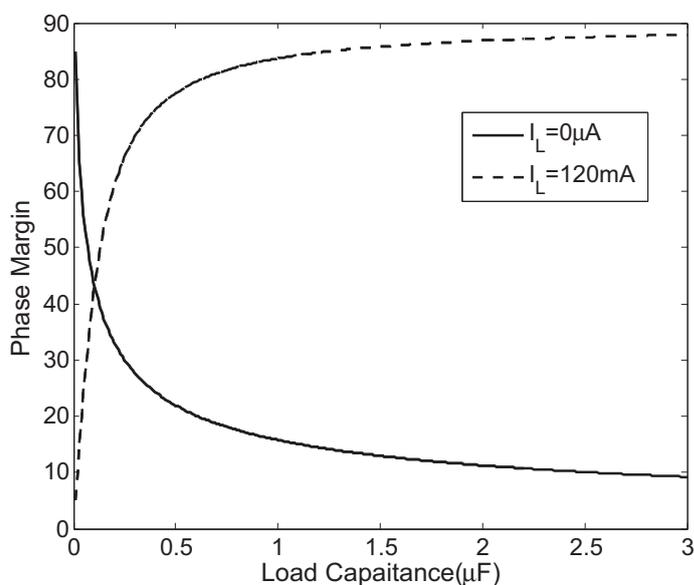
Figure 5.1: Phase margin among output capacitor sizing range.
