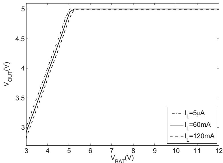
Figure 4.1:  $V_{OUT}$  versus  $V_{BAT}$  ( $V_{CP}=10V$ , typical process corner, temp= $27^{\circ}C$ ).
