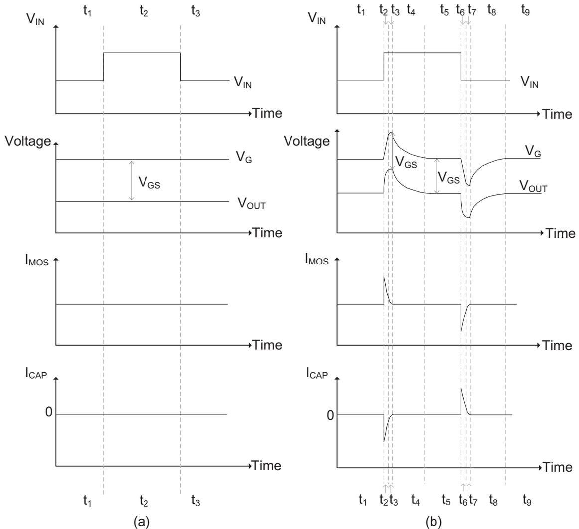
Figure 2.5: One possible NMOS linear regulator line transient response (a) with infinite bandwidth (b) with finite bandwidth.
