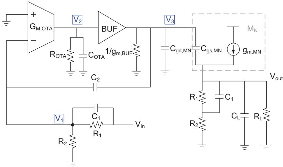
Figure B.1: Signal signal model for the whole loop.
