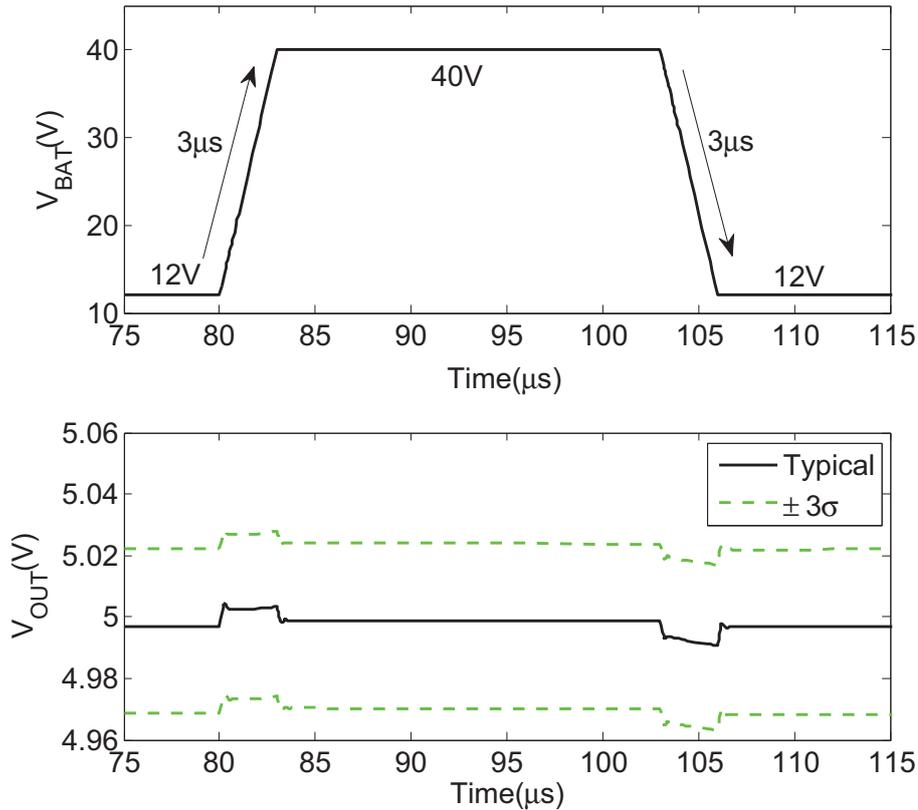
Figure 4.11: High battery line transient response ( $I_L=120\text{mA}$ ,  $-40^\circ\text{C}\sim 175^\circ\text{C}$ ).
