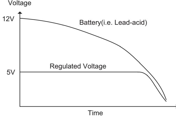
Figure 2.2: Lead-acid discharge curves under a constant load current.
