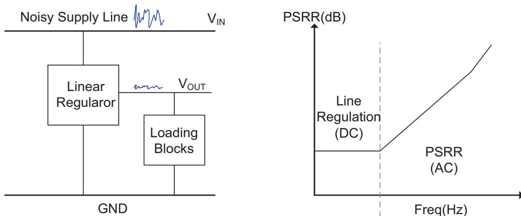
Figure 2.8: (a) Power supply rejection on linear regulator (b) typical bode plot of PSRR.
