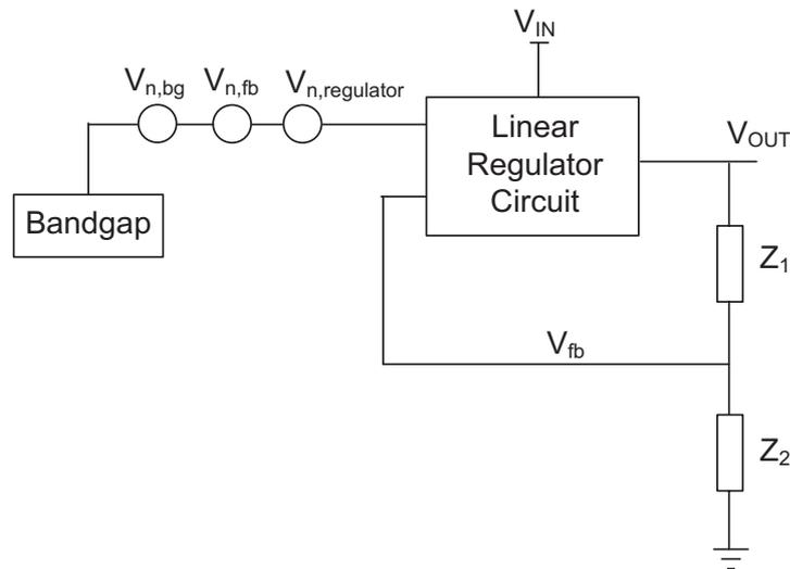
Figure 2.9: Equivalent input noise of linear regulator.
