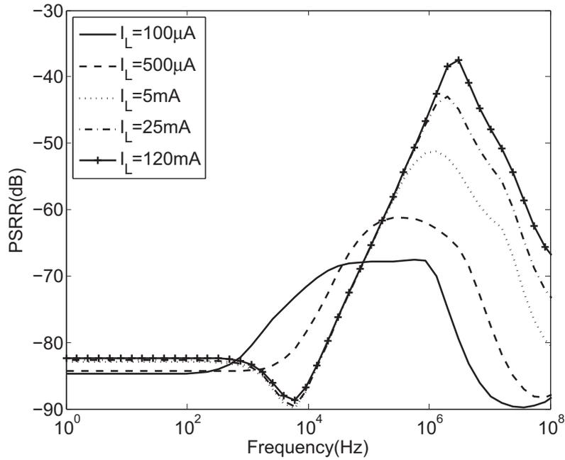
Figure 4.15: PSRR over  $I_L$  ( $V_{BAT}=12V$ , typical process corner,  $27^\circ C$ ).
