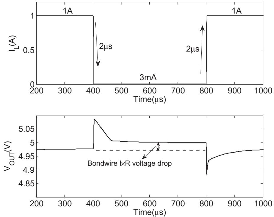
Figure 5.5: A 1A linear regulator load transient response.
