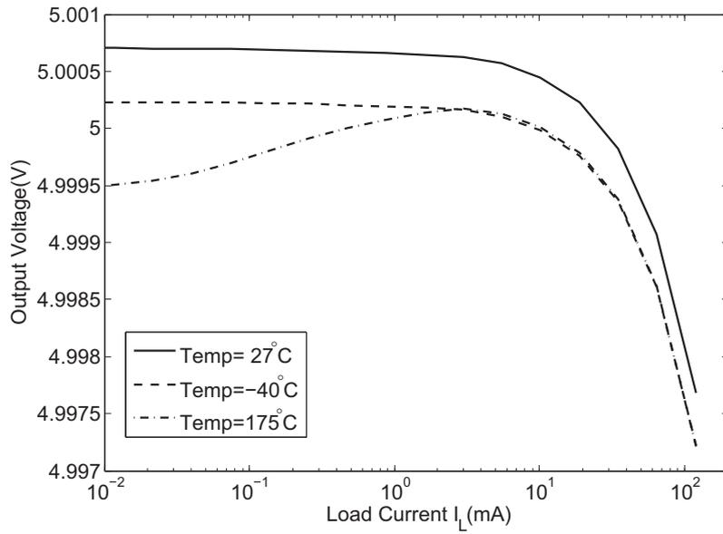
Figure 4.5: Static load regulation ( $V_{BAT}=12V$ , typical process corner).
