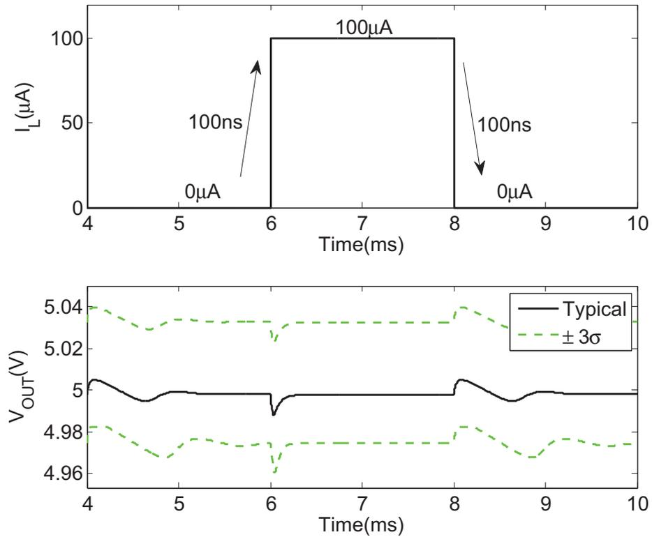
Figure 4.13: Low current load transient response ( $V_{\text{BAT}}=12\text{V}$ ,  $-40^\circ\text{C}\sim 175^\circ\text{C}$ ).
