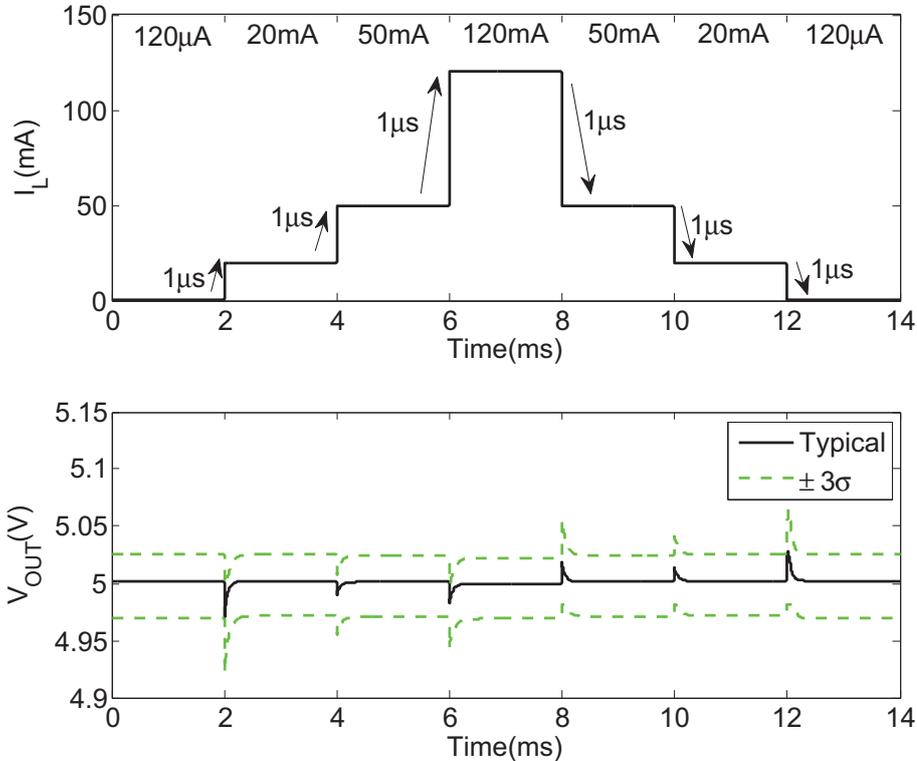
Figure 4.14: Staircase load transient response ( $V_{BAT}=12V, -40^{\circ}C \sim 175^{\circ}C$ ).
