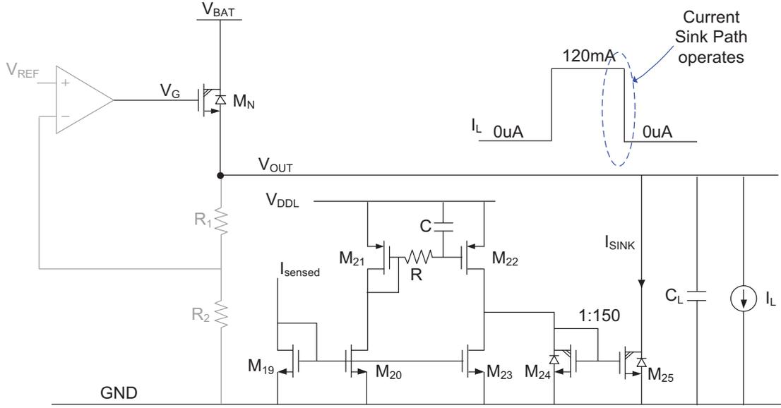
Figure E.2: Current sink path circuit.
