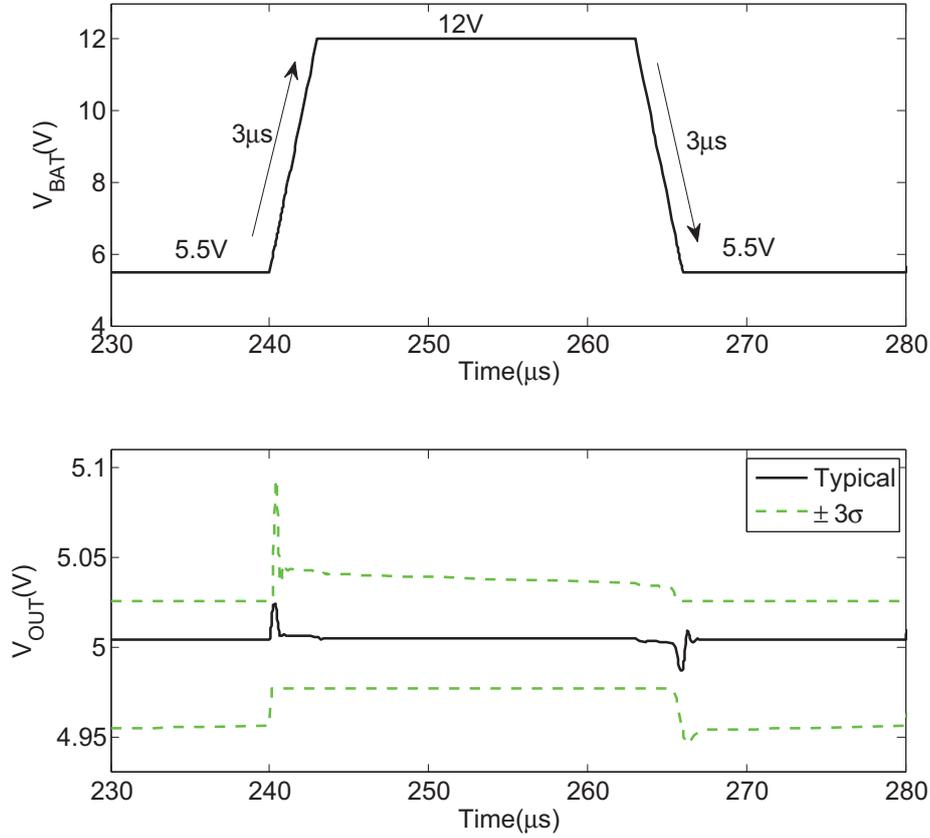
Figure 4.10: Low battery line transient response ( $I_L=120\text{mA}$ ,  $-40^{\circ}\text{C}\sim 175^{\circ}\text{C}$ ).
