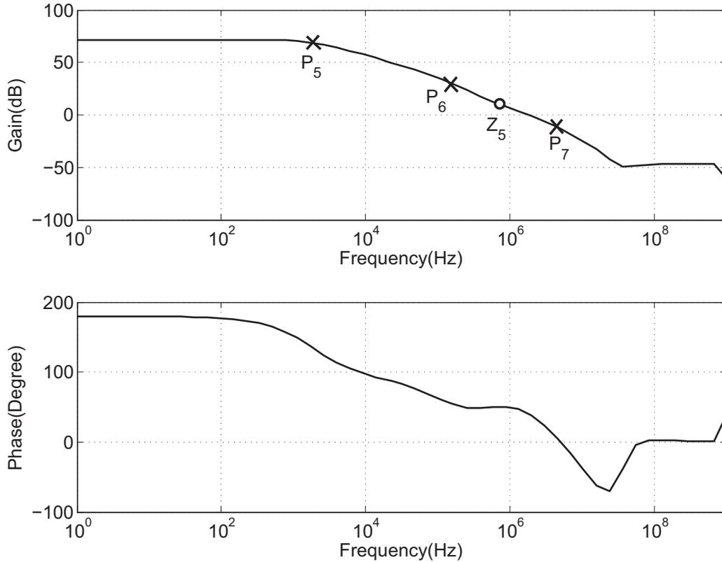
Figure 3.19: Current sensing loop bode plot at  $I_L = 0\mu A$ .
