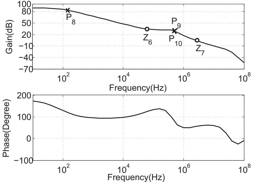
Figure 3.30: Current limitation loop bode plot ( $R_L=10\Omega$ ).
