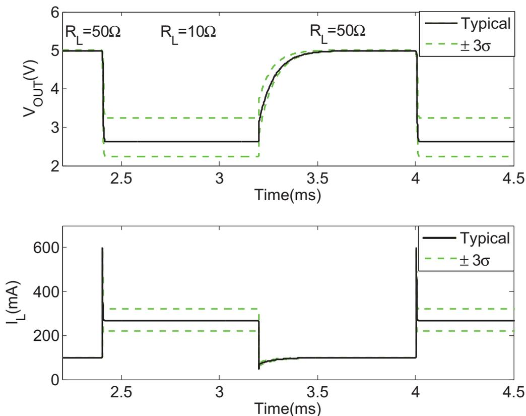
Figure 4.18: Over-current protection transient behavior ( $V_{BAT}=12V, -40^{\circ}C \sim 175^{\circ}C$ ).
