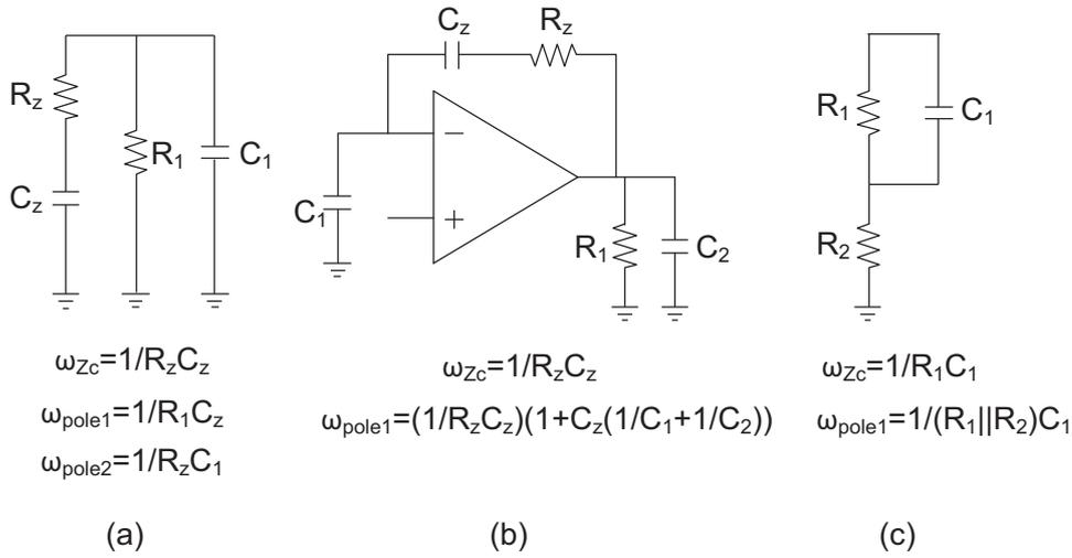
Figure 3.8: Adding a zero and its associated pole.
