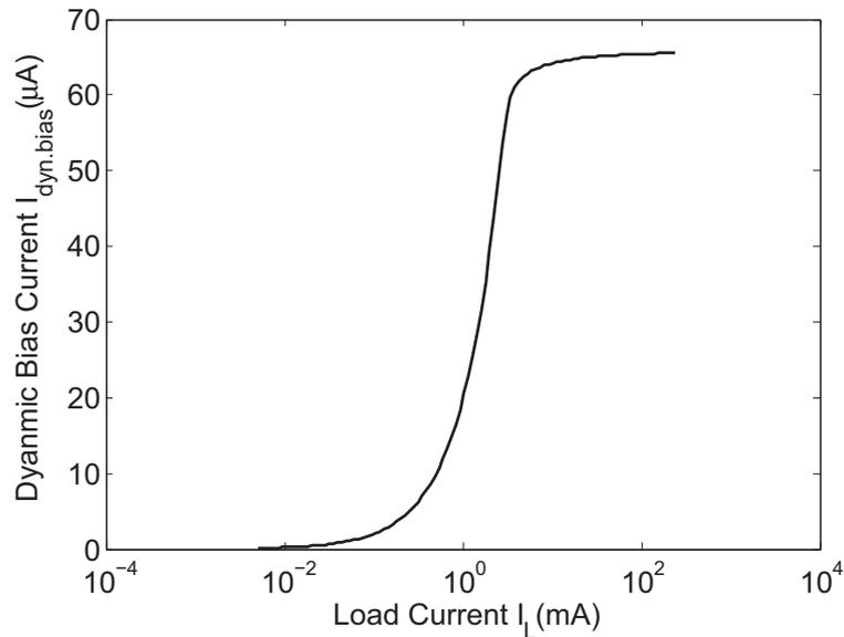
Figure 3.23: Adaptive biasing current versus load current  $I_L$ .
