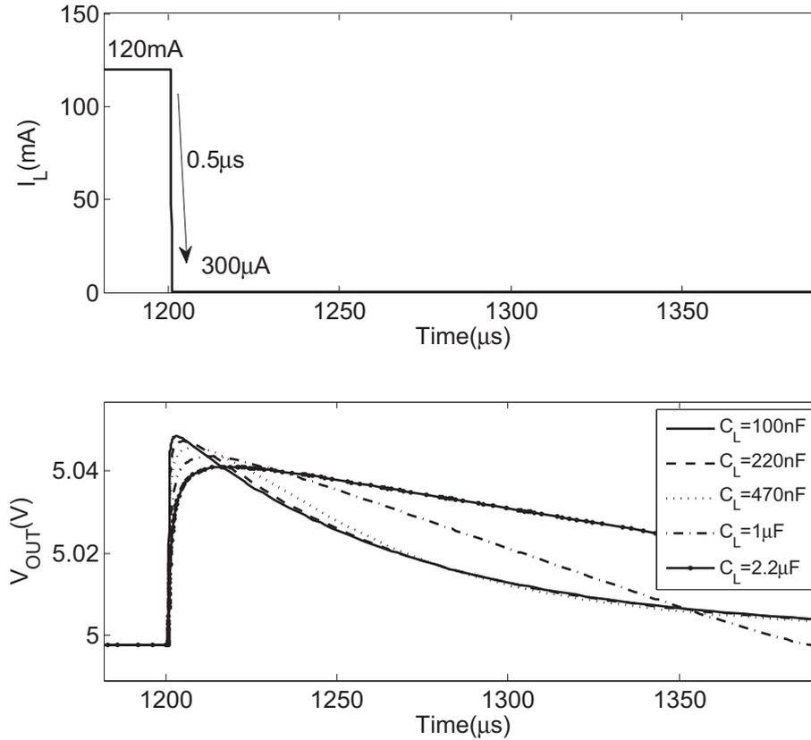
Figure 5.4: Load transient response ( $I_L$  decreasing) with different  $C_L$ .
