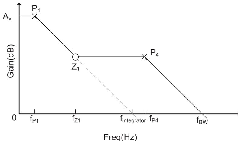
Figure 3.15: Stability analysis at high load current.
