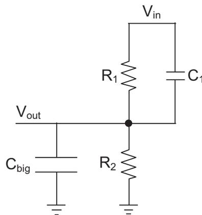
Figure 3.9: Adding a zero while merging the associated pole with dominate pole.
