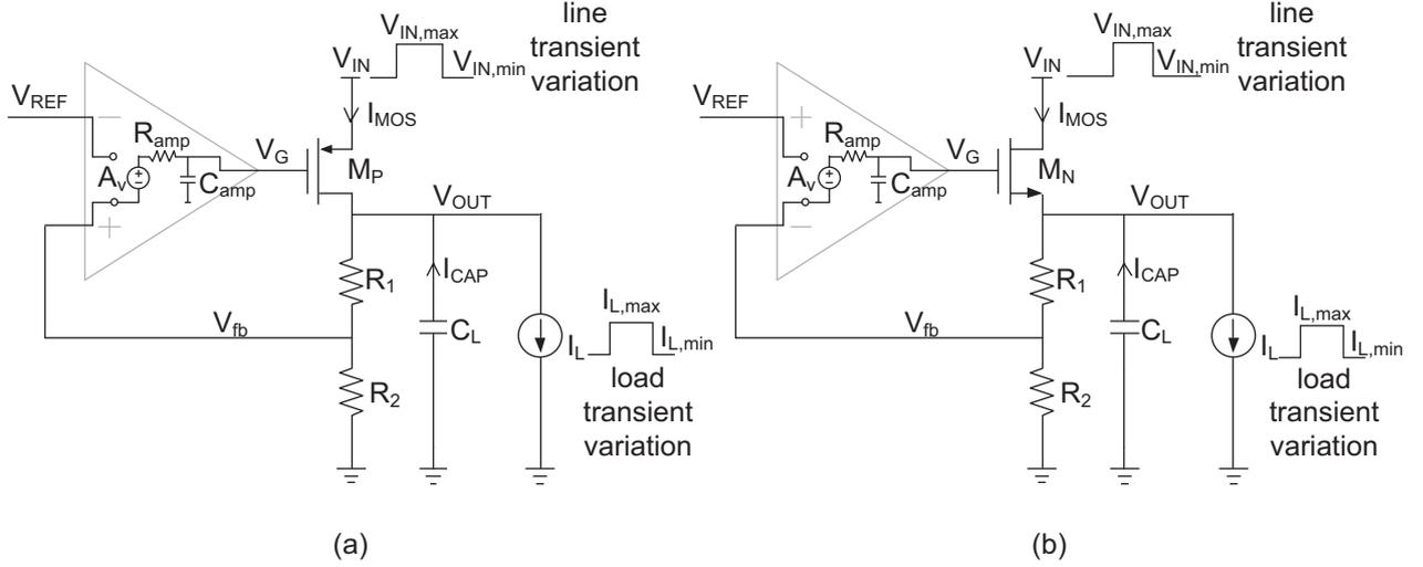
Figure 2.3: Transient response of (a) PMOS regulator (b) NMOS regulator.
