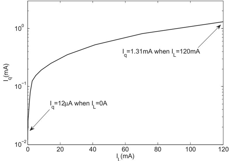
Figure 4.2:  $I_q$  versus  $I_L$  ( $V_{BAT}=12\text{V}$ , typical process corner, temp= $27^\circ\text{C}$ ).
