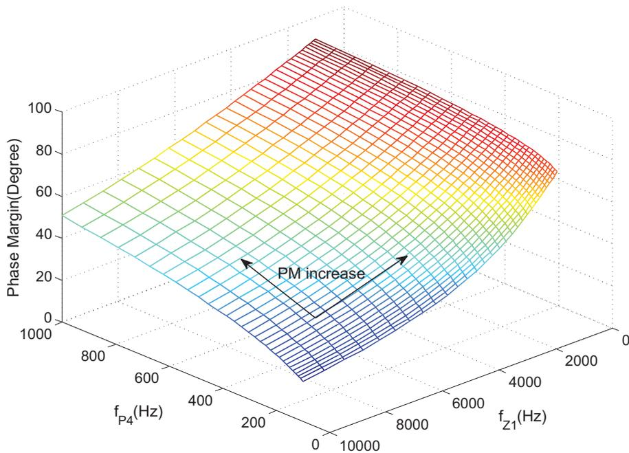
Figure 3.13: Phase margin analysis at  $I_L=0\mu\text{A}$ .
