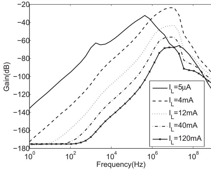
Figure 3.24: Adaptive biasing loop gain plot.
