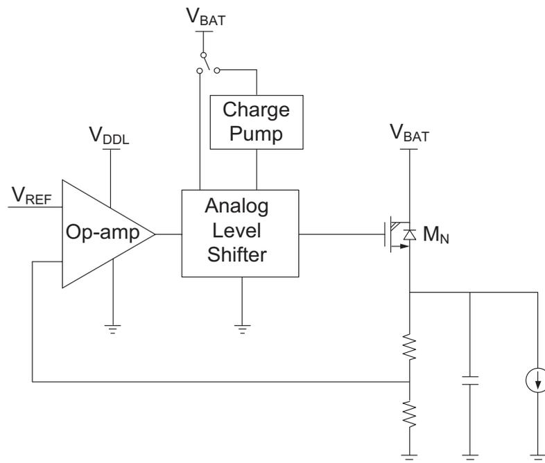
Figure 3.2: NMOS linear regulator topology.
