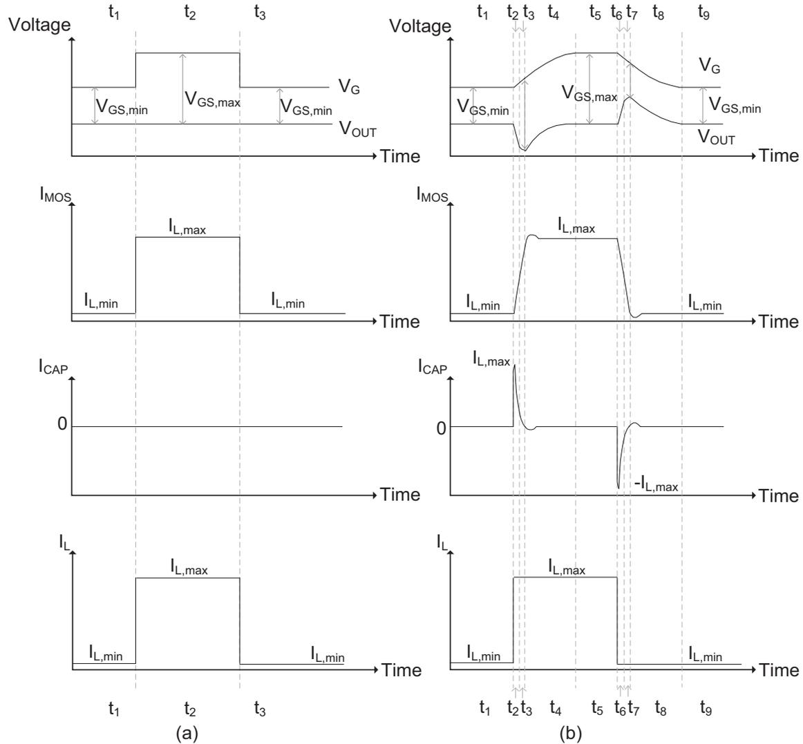
Figure 2.7: One possible NMOS linear regulator load transient response (a) with infinite bandwidth (b) with finite bandwidth.
