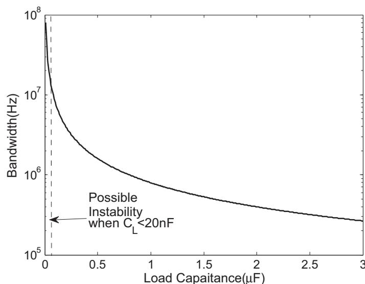
Figure 5.2: Bandwidth at high current load over  $C_L$ .
