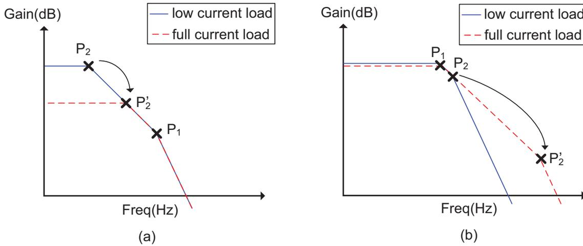
Figure 2.12: Bode plot of (a) PMOS regulator (b) NMOS regulator.
