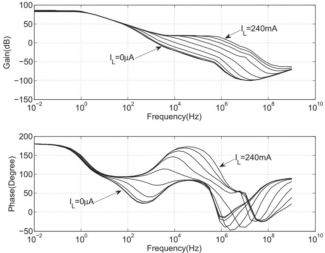
Figure 4.7: Bode plot over different  $I_L$ .
