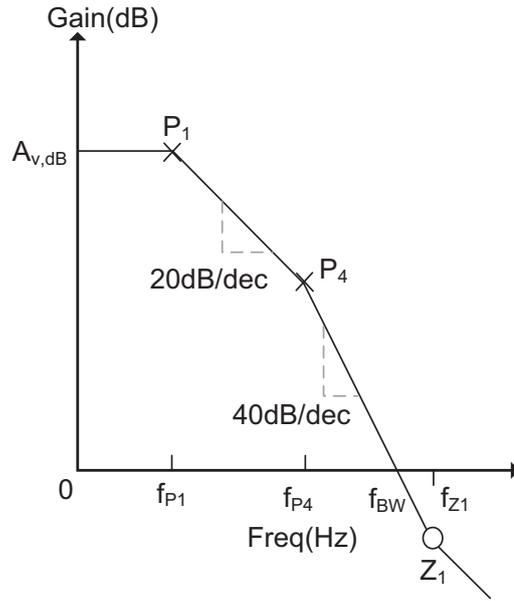
Figure 3.12: Simplified bode plot analysis at  $I_L=0\mu\text{A}$ .
