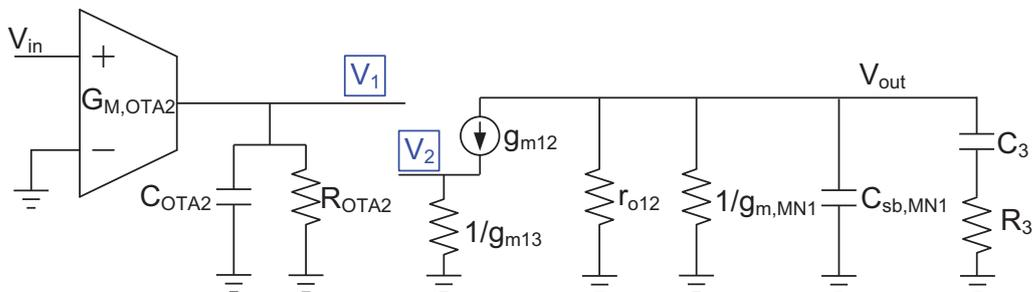
Figure 3.18: Small signal equivalent of current sensing loop.
