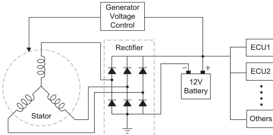
Figure 1.1: A simplified automotive power management system.
