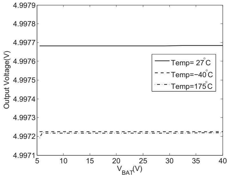
Figure 4.4: Static line regulation ( $I_L=120\text{mA}$ , typical process corner).
