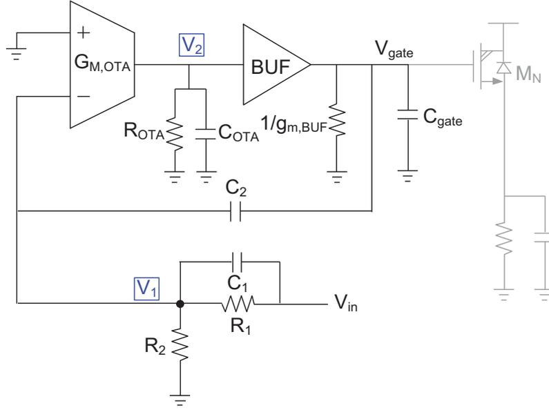
Figure 3.10: Integrator configuration with  $C_2$ .
