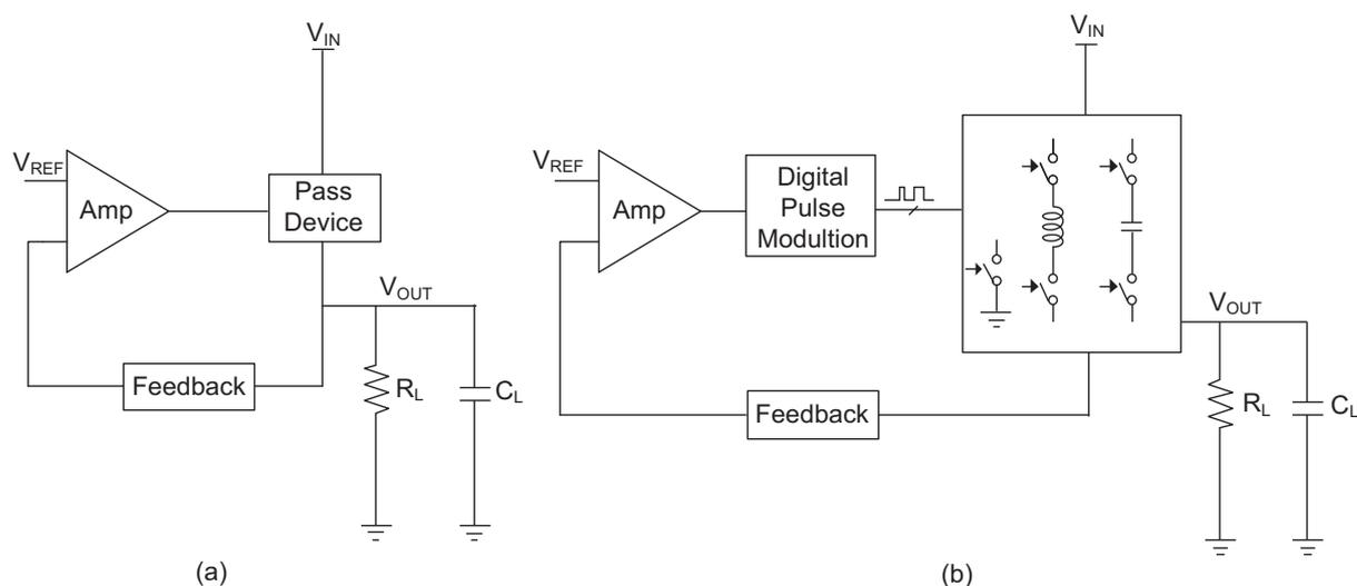
Figure 1.3: DC voltage converter topology (a) linear regulator and (b) switching regulator.
