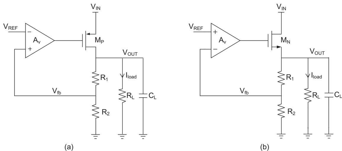
Figure 2.1: Basic linear regulator topology with (a) PMOS as pass device (b) NMOS as pass device.
