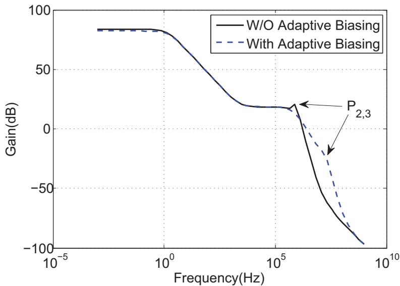
Figure 3.25: Linear regulator high current load bode plot with adaptive biasing
