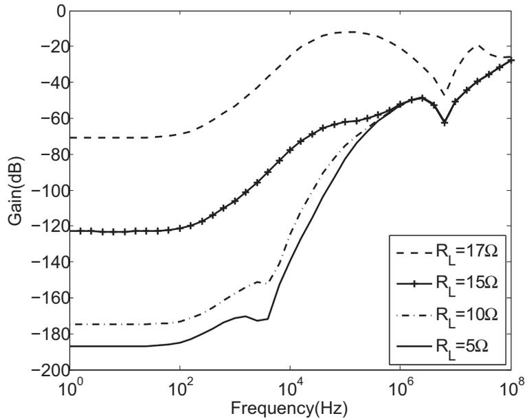
Figure 3.32: Main voltage regulation loop gain plot over  $R_L$ .
