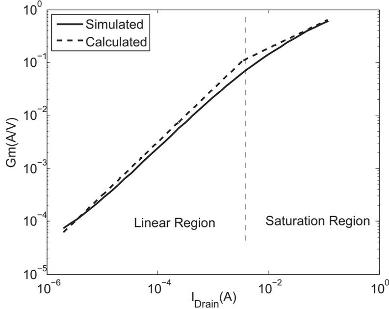
Figure 3.5: Transconductance of NMOS power transistor.
