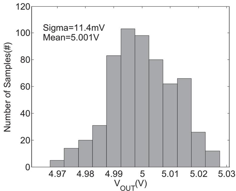
Figure 4.6: Output voltage spread ( $V_{BAT}=12V, I_L=0, -40^\circ C \sim 175^\circ C$ ).
