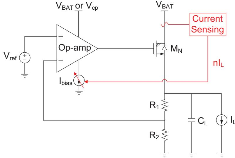
Figure 3.16: Illustration of adaptive biasing idea.
