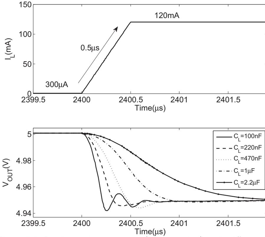
Figure 5.3: Load transient response ( $I_L$  increasing) with different  $C_L$ .
