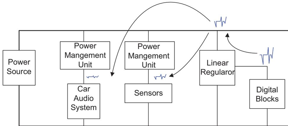
Figure 2.10: EMI example in automotive environment.
