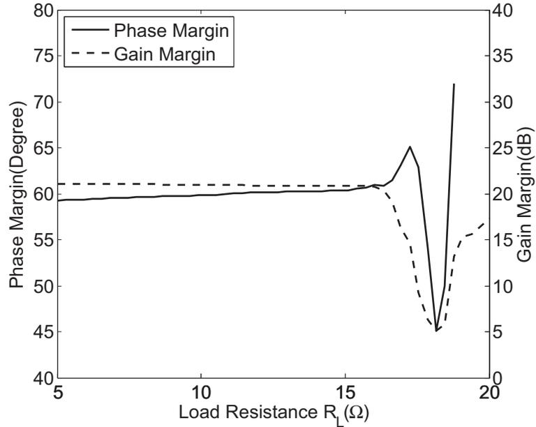
Figure 3.31: Current limitation stability over  $R_L$ .
