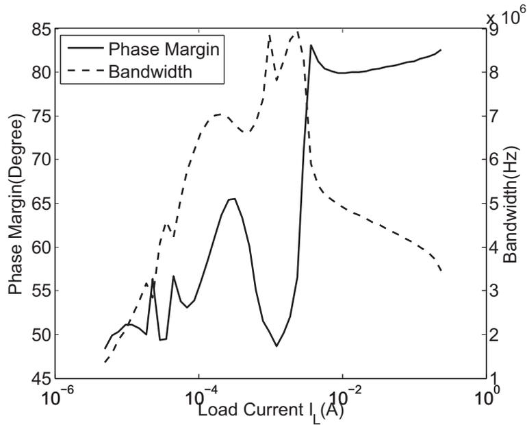
Figure 3.21: Phase margin and bandwidth versus load current for current sensing loop.
