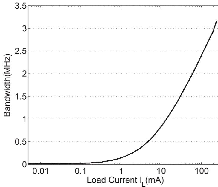
Figure 4.9: Bandwidth versus  $I_L$ .
