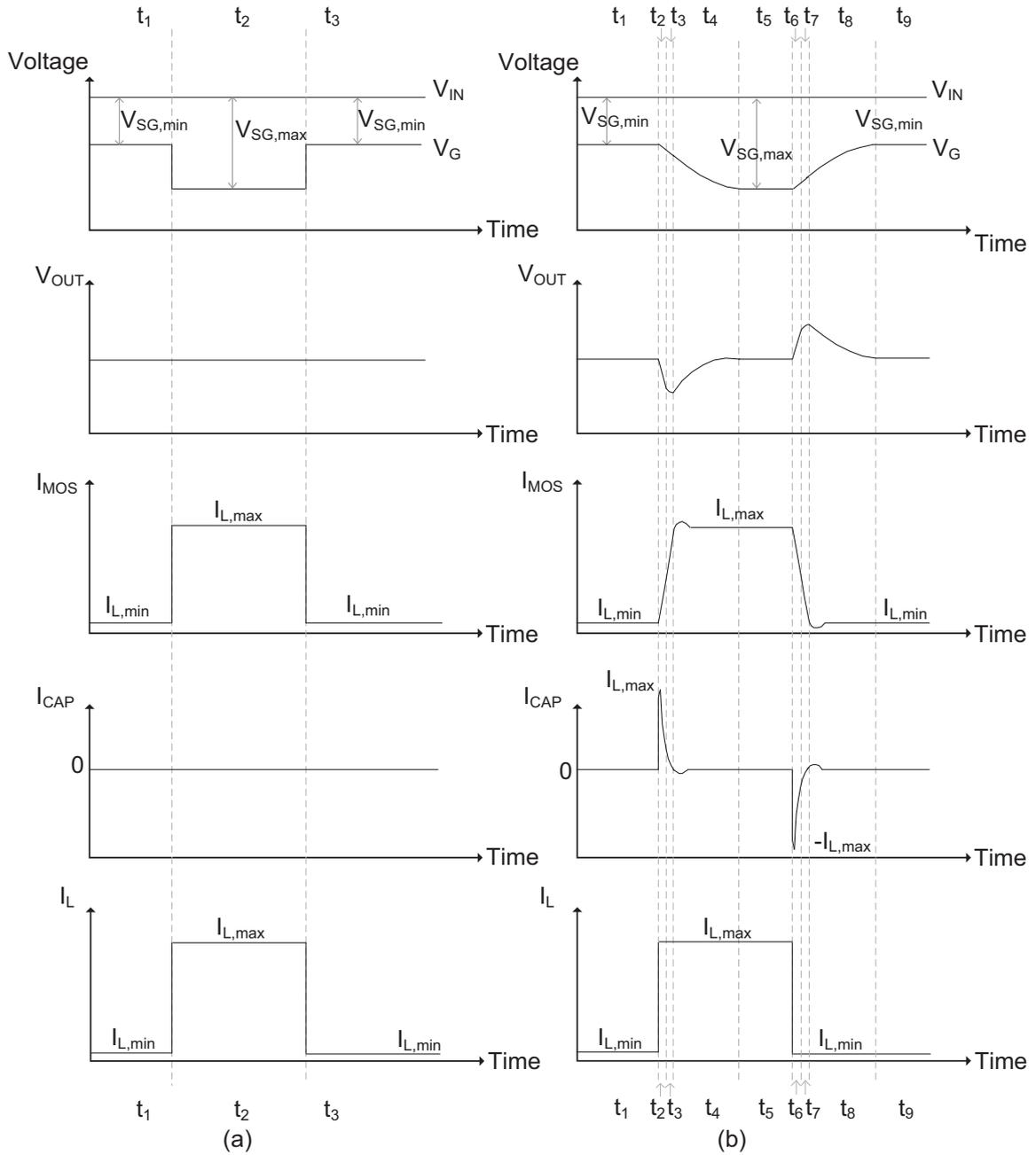
Figure 2.6: One possible PMOS linear regulator load transient response (a) with infinite bandwidth (b) with finite bandwidth.
