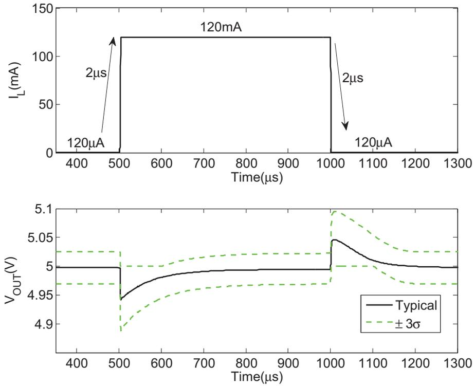
Figure 4.12: Load transient response ( $V_{\text{BAT}}=12\text{V}$ ,  $-40^\circ\text{C}\sim 175^\circ\text{C}$ ).
