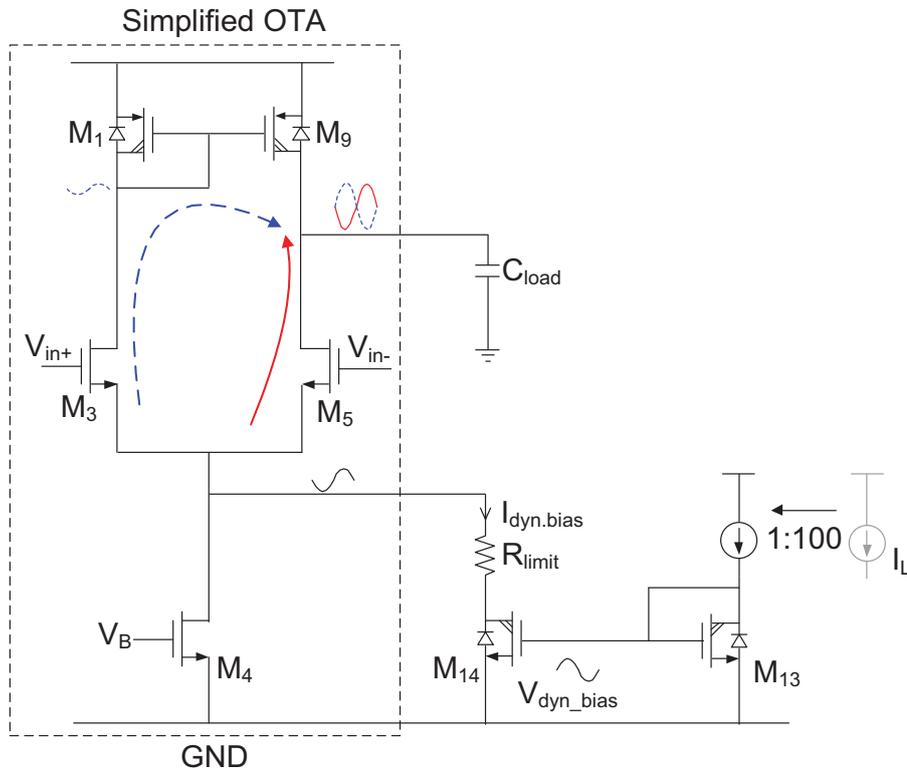
Figure 3.22: Adaptive biasing on the main voltage feedback loop stability analysis.
