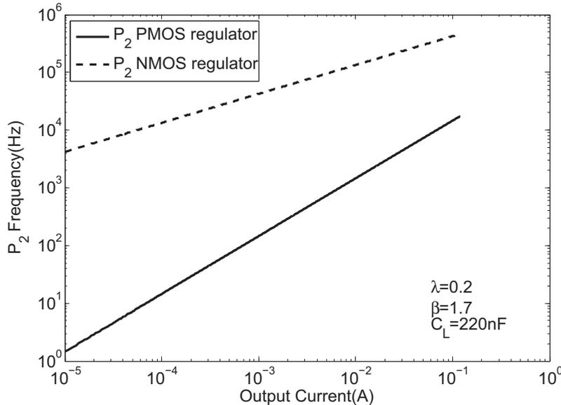
Figure 2.13:  $P_2$  movement over load current.
