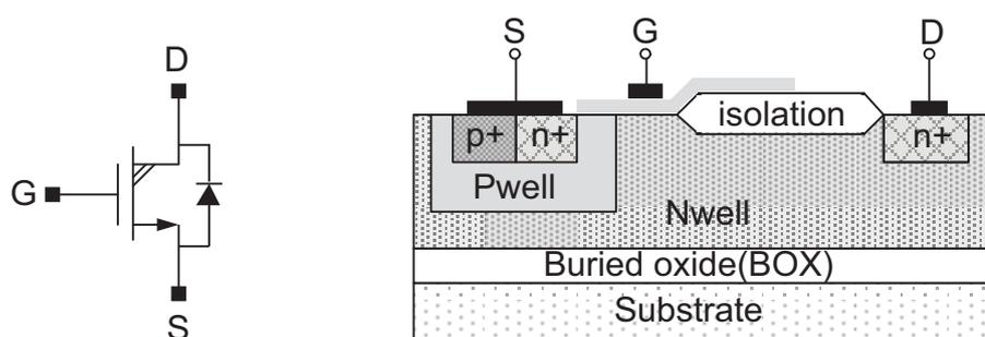
Figure 3.1: Power MOS symbol and the cross section view.
