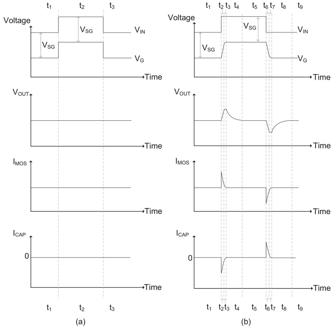
Figure 2.4: One possible PMOS linear regulator line transient response (a) with infinite bandwidth (b) with finite bandwidth.
