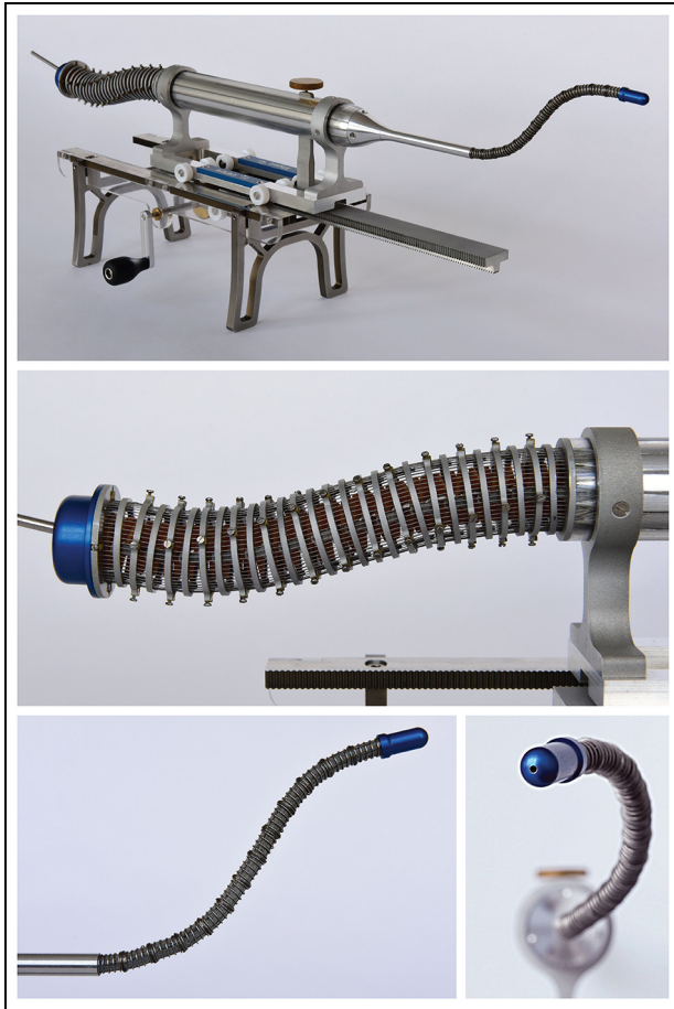
Figure 6. Proof-of-concept prototype; the MemoFlex. All parts were fabricated out of aluminium, except for the wheels (nylon), gear rack (stainless steel) and gears (brass). The outside of the shaft is transparent to allow visual feedback of the cables during their assembly.
