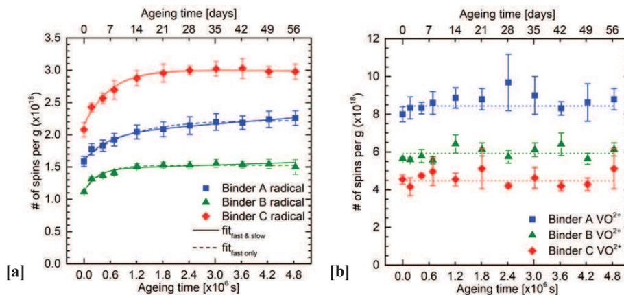
201 Figure 5: Evolution of the carbon-centred radical and the used radical fitting, based on a dual-sequential or a fast reaction model [a] and  $\text{VO}^{2+}$  centres
