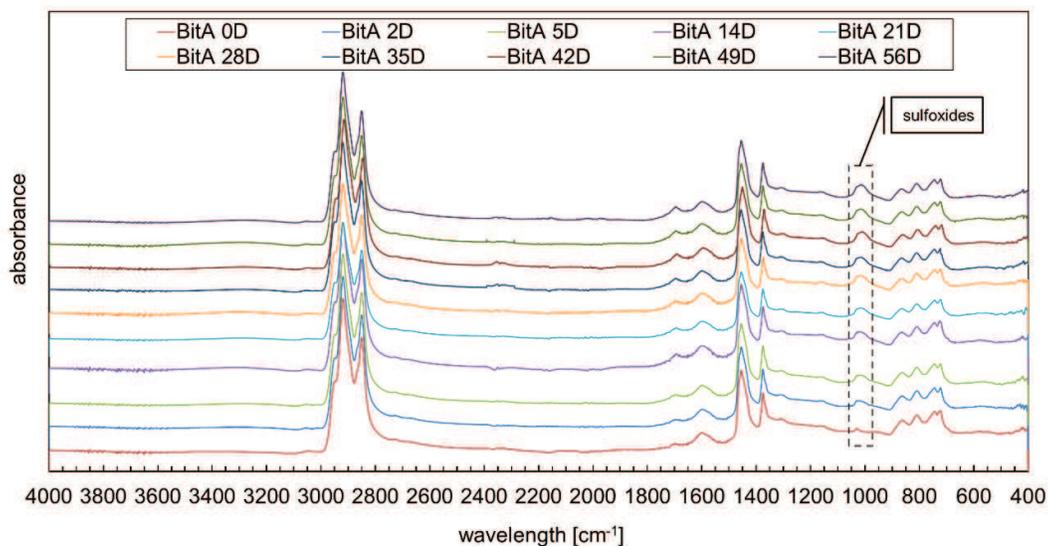
115 Figure 2: Evolution with ageing time (0-56 days) for exemplary FTIR spectra of bitumen A.
