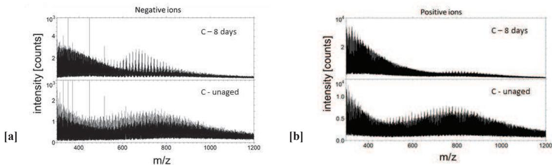
271 Figure 10: High mass range of negative [a] and positive ion spectra of bitumen C before and after M-TFOT ageing for 8 days [b].
