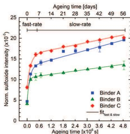
186 Figure 4: Evolution of the FTIR normalised sulfoxide intensity over ageing time and the fitting used, based on a dual-sequential model [4,12].
