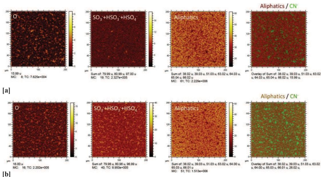
309 Figure 13: High-resolution TOF-SIMS images of selected negative fragment ions on the surface of bitumen C before [a] and after ageing [b].
