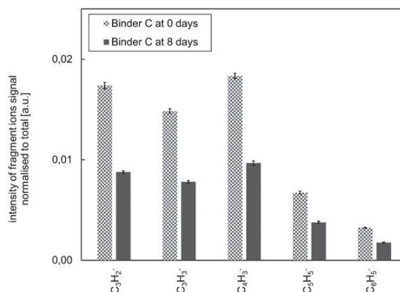
Figure 9: Negative ions of binder C assigned to aliphatic
