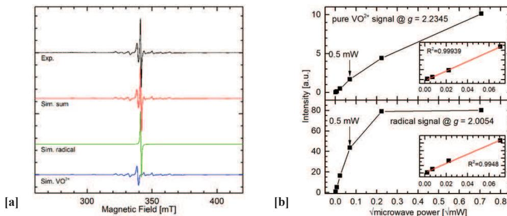
146 Figure 3: Room temperature cw X-band EPR spectra of binder A with its simulations [a] and its signal intensity contrasted with square root of
