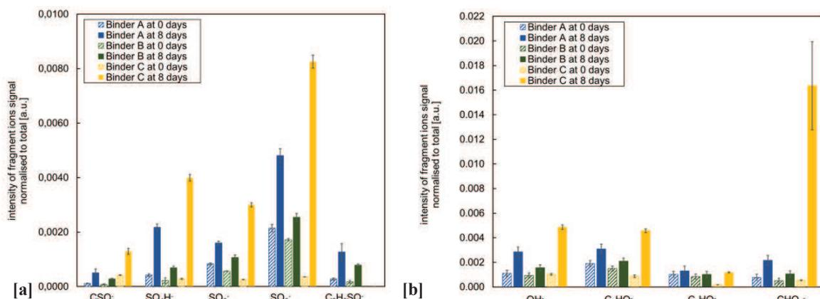
269 Figure 7: Intensity of  $\text{SO}_x$ -containing [a] and  $\text{HO}_x$ -containing compounds via TOF-SIMS for all three binders [b]. Mean values from three
