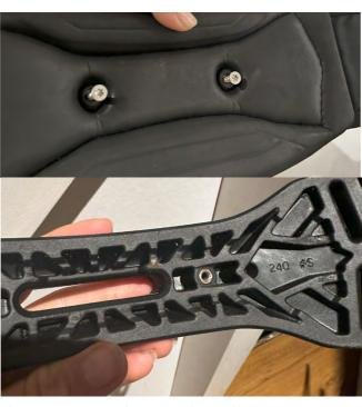
Figure 109: Screws used to connect the spreaderbar's components
