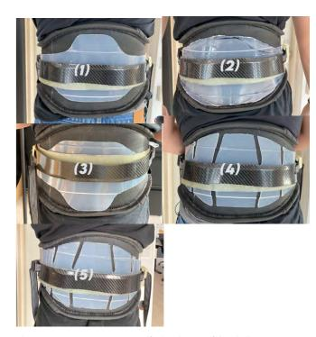
Figure 100: 1:1 Prototype to verify the shapes of the shell
