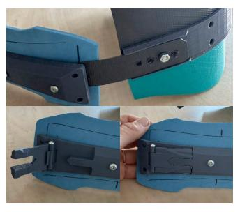
Figure 107: First prototype of the lever system with singular inner hook
