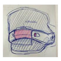
CONCEPT 6: HARNESS ADAPTABLE IN TORSO WIDTH THROUGH MODULAR PARTS
