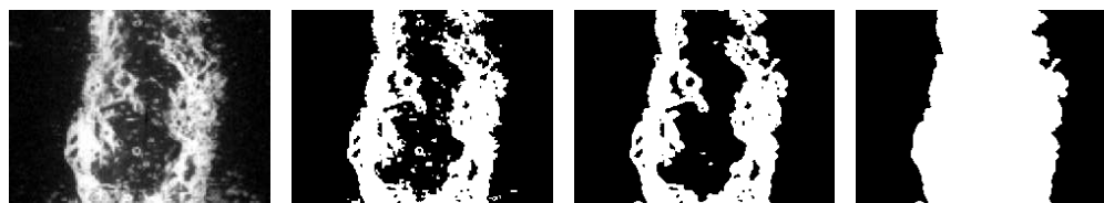
Figure 9. Image processing steps performed by the MATLAB code. From left to right: raw image obtained by the high-speed camera, binary image, image after the moving average filter, and final image with holes filled.
