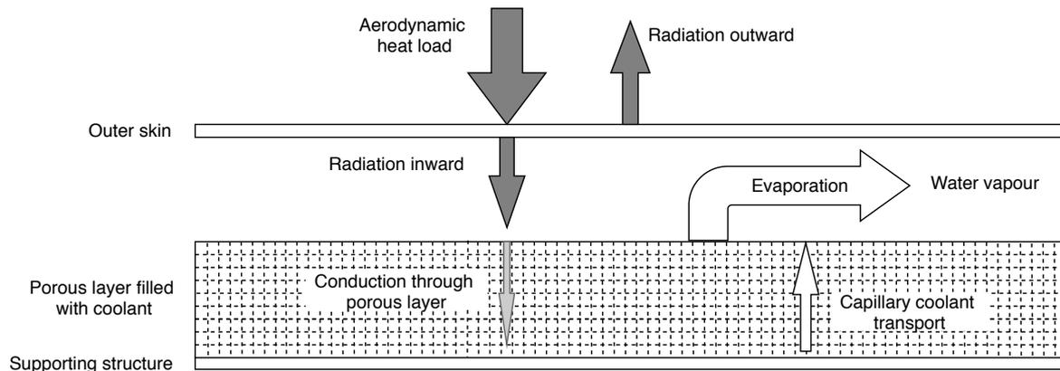
Figure 3-1: Schematic representation of energy flow in Enhanced radiation cooled TPS.
