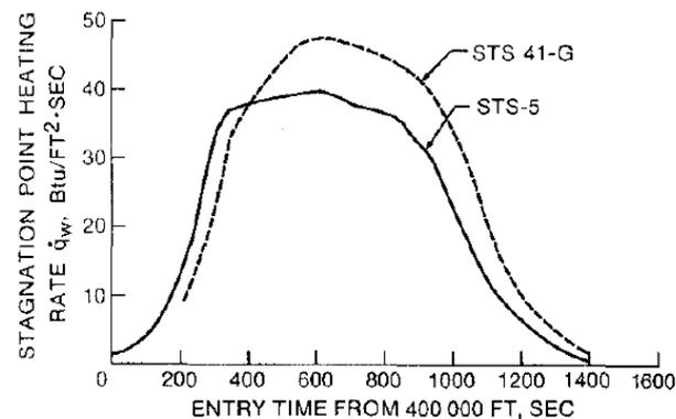
Figure 2-4: STS Stagnation-point heat flux during re-entry (Curry et al., 1986).
