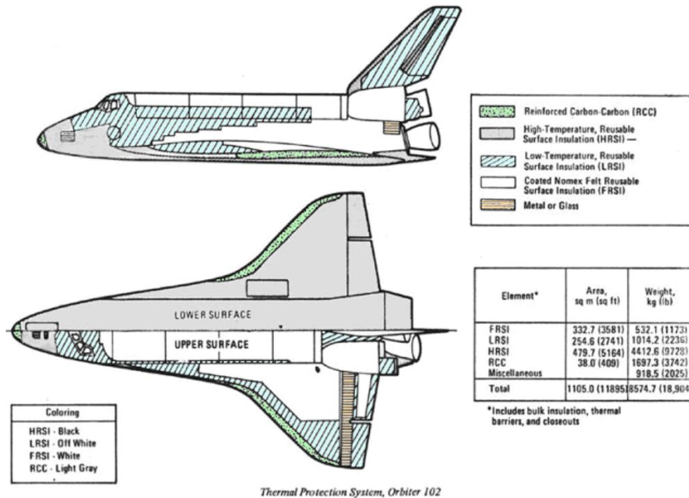
Figure 2-5: STS thermal protection systems (NASA).
