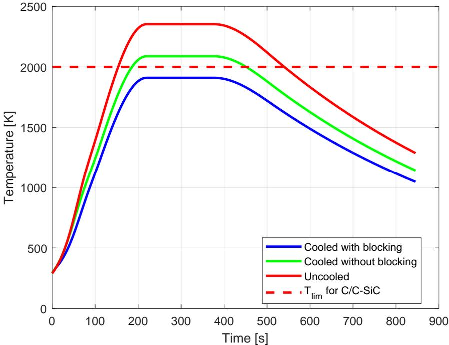
Figure 5-7: Variation of skin temperature as a function of time (C/C-SiC, cooled with blocking, 5mm gap).
