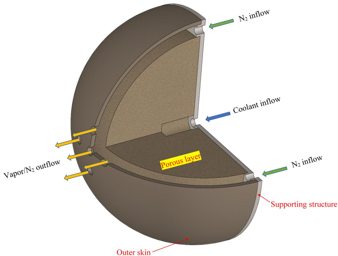
Figure 5-14: 3D view of the nose with a modified enhanced radiation cooled TPS.
