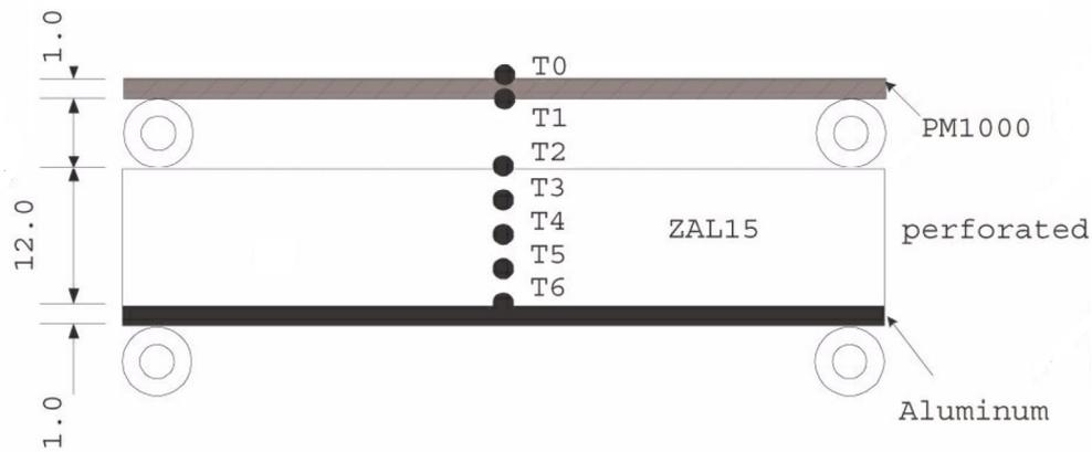
Figure 4-6: Location of thermocouples in the test setup Buursink (2005).
