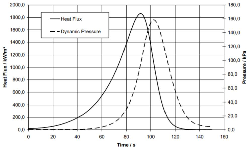
Figure 2-8: Heat flux and dynamic pressure variation for the EXPERT vehicle nose over time (Reimer et al., 2009).
