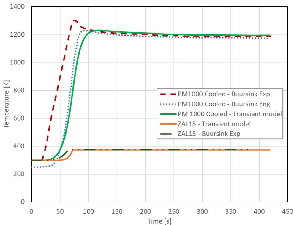
Figure 4-7: Verification of transient model (cooled) using experimental and analytical data given by Buursink (2005).
