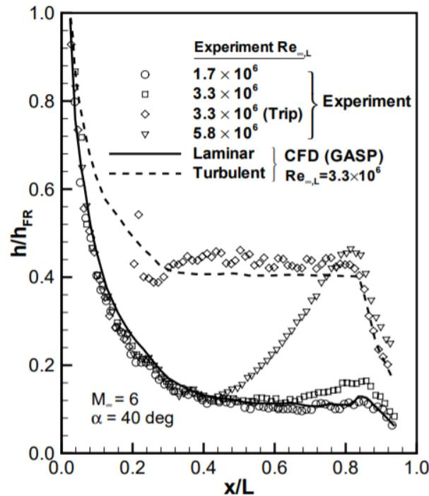
Figure 2-6: Predicted and measured heating for the X-33 vehicle along the windward centreline (Hollis et al., 2001).
