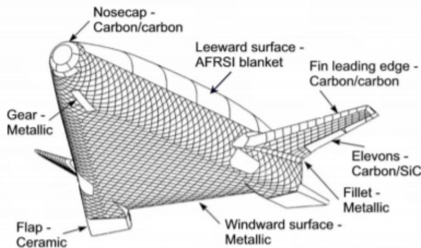
Figure 2-7: TPS material design for the X-33 (Hollis et al., 2001).
