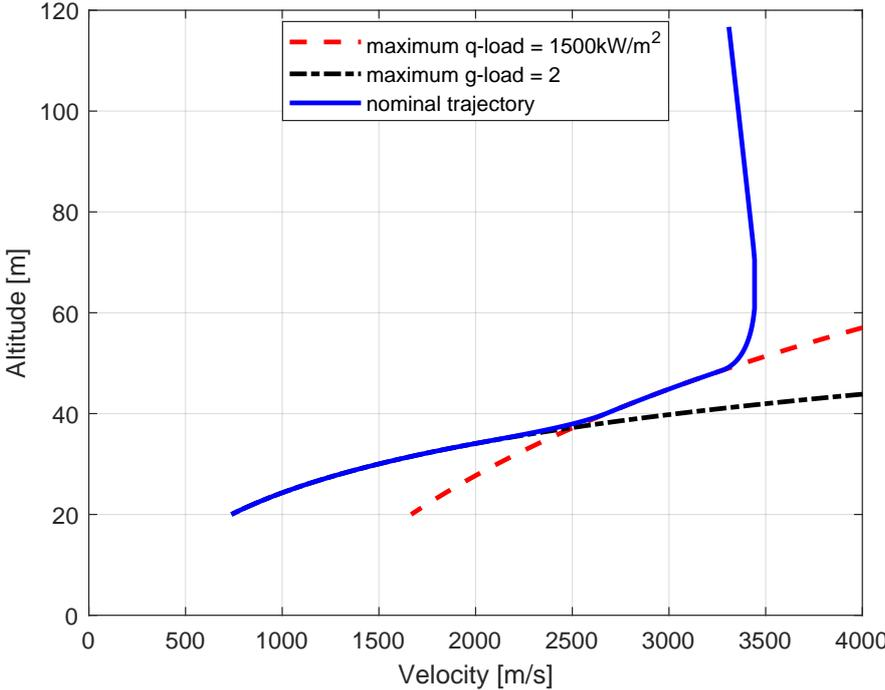
Figure 2-23: Altitude-velocity profile for nominal trajectory.
