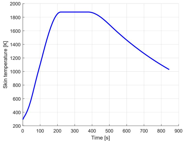
Figure 5-12: Variation of skin temperature as a function of time (C/C-SiC, cooled with blocking).
