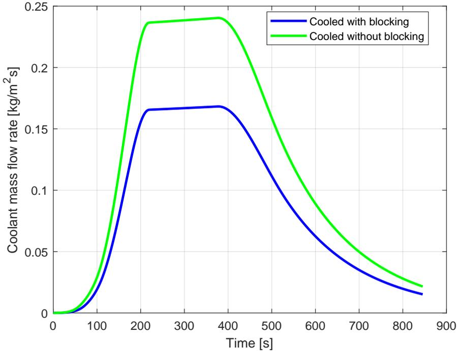
Figure 5-8: Variation of coolant mass flow rate as a function of time (C/C-SiC, cooled with blocking, 5mm gap).
