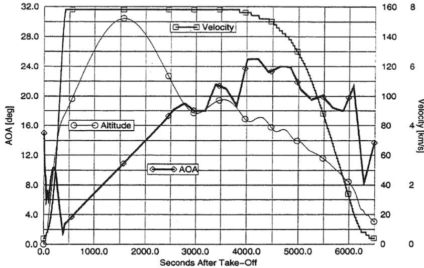
Figure 2-19: Nominal trajectory for FSS-15 (OAE) (Vollmer, 1992).
