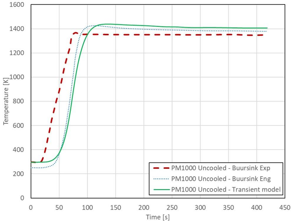
Figure 4-8: Verification of transient model (uncooled) using experimental and analytical data given by Buursink (2005).
