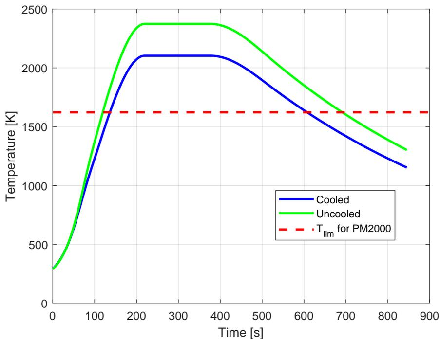
Figure 5-2: Variation of skin temperature as a function of time (PM2000, cooled and uncooled).
