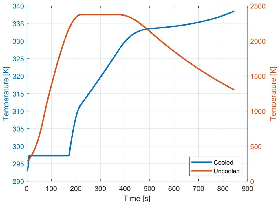
Figure 5-3: Variation of porous layer temperature (outermost surface) as a function of time (PM2000, cooled and uncooled).
