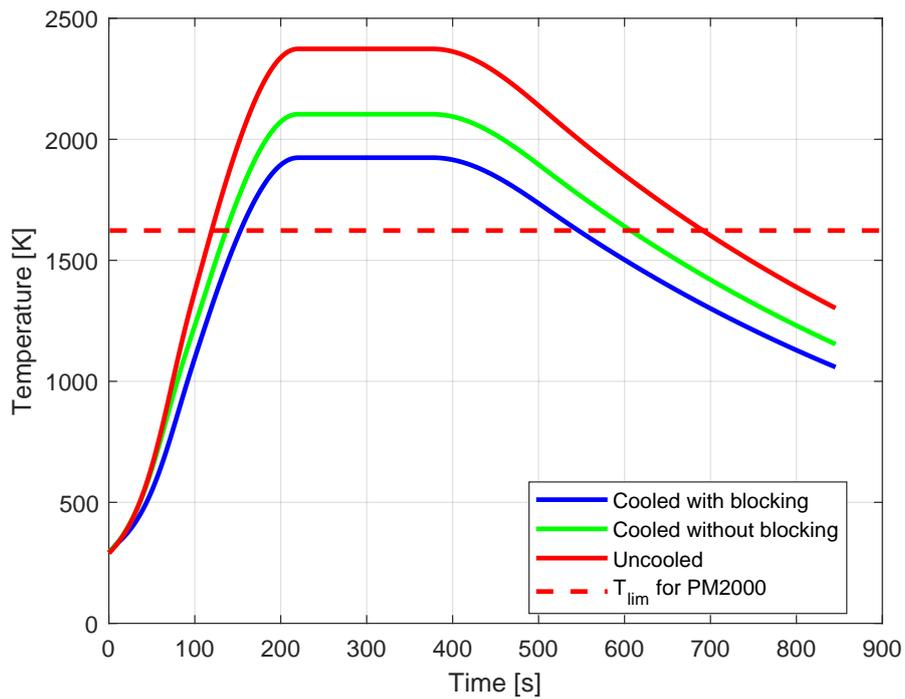
Figure 5-5: Variation of skin temperature as a function of time (PM2000, cooled, with and without blocking).
