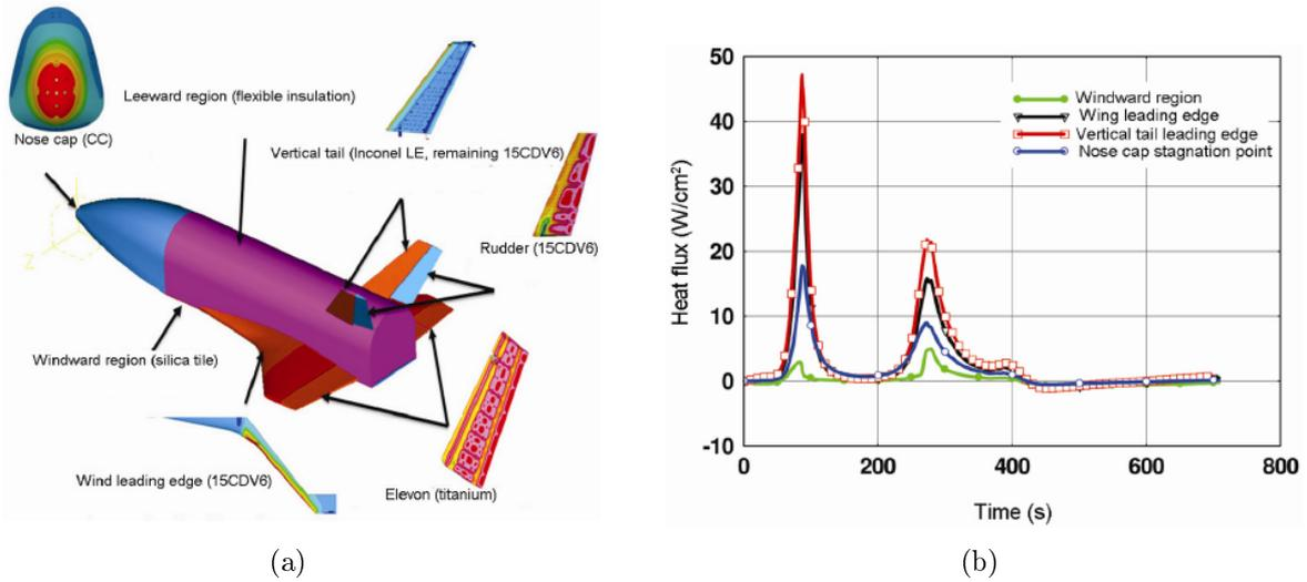
Figure 2-16: (a) Various structures and (b) Cold wall heat flux estimated at various locations of RLV-TD (Sivamurugan et al., 2018).
