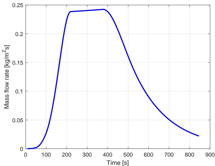
Figure 5-4: Variation of coolant mass flow rate as a function of time (PM2000, cooled).
