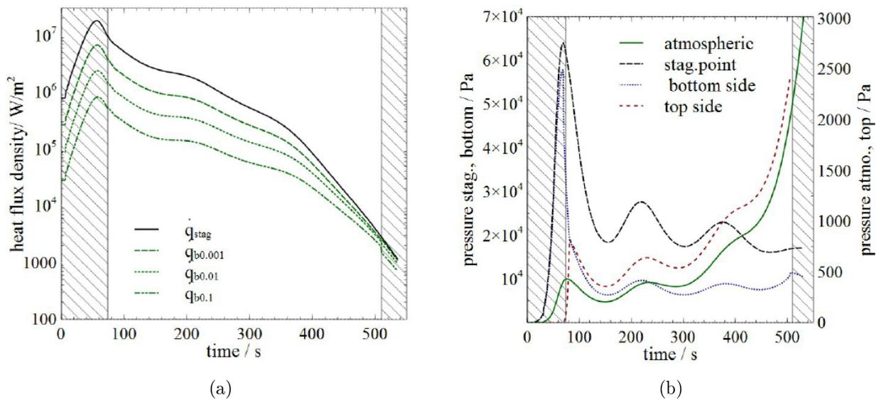
Figure 2-12: (a) Heat flux predicted for stagnation point and bottom side and (b) Pressure distribution and atmospheric pressure variation for SHEFEX III (Dittert et al., 2015).
