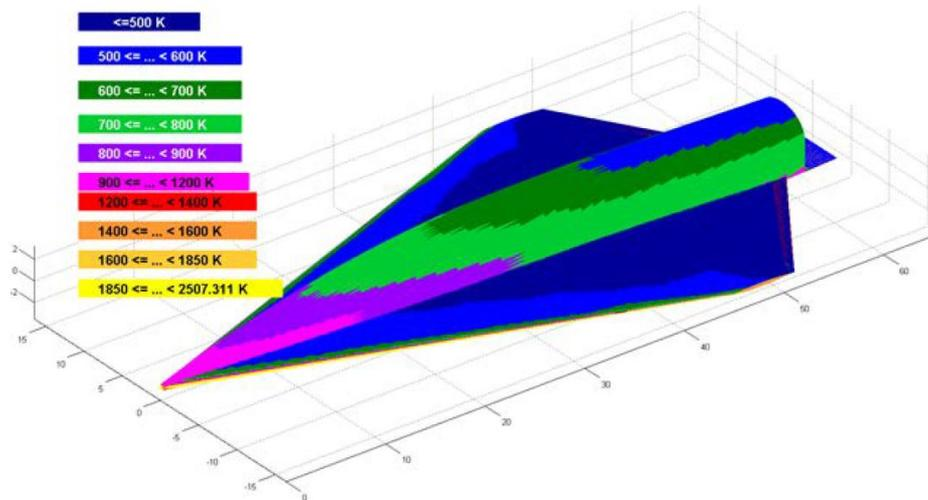
Figure 2-14: Overall maximum surface temperature areas reached on the upper side of SpaceLiner (Sippel, 2015).
