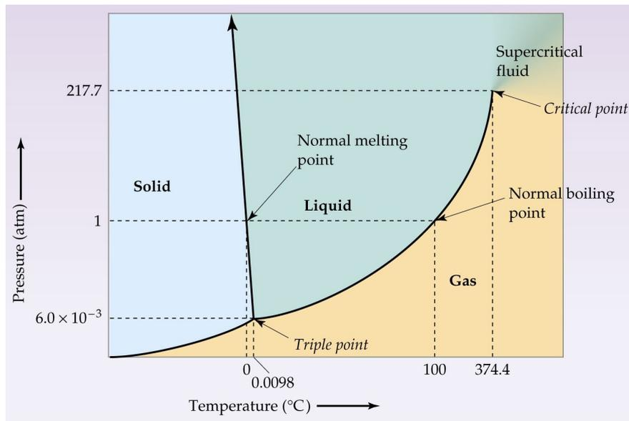
Figure 3-2: A phase diagram of water (McMurry and Fay, 2004).
