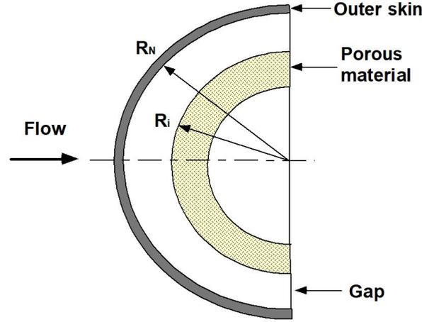
Figure 4-1: Configuration of Enhanced radiation cooling.
