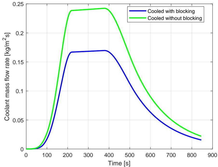
Figure 5-6: Variation of coolant mass flow rate as a function of time (PM2000, cooled, with and without blocking).
