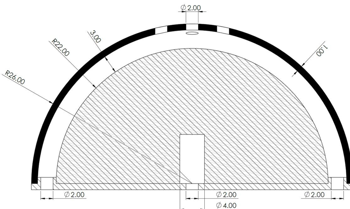
Figure 5-15: 2D view of the nose with a modified enhanced radiation cooled TPS (dimensions in mm).
