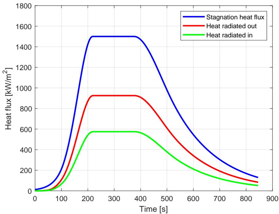
Figure 5-1: Distribution of heat flux (PM2000, cooled).
