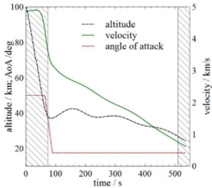
Figure 2-11: SHEFEX III trajectory design (Dittert et al., 2015).
