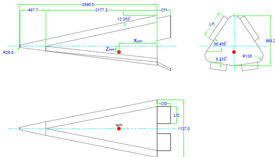
Figure 2-21: Hyperion-II design 5 geometry, as drawn by Dijkstra (2012).
