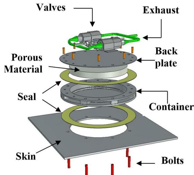
Figure 2-10: Enhanced radiation cooling experiment fitted on-board the EXPERT vehicle (Sudmeijer, 2005).
