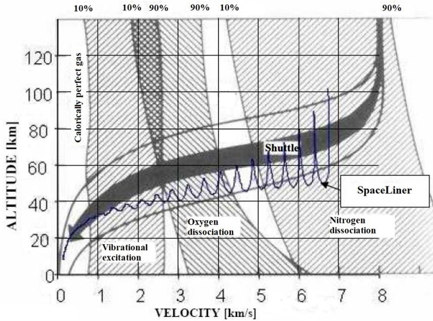
Figure 2-13: SpaceLiner skip trajectory vs. Shuttle re-entry (van Foreest et al., 2007).
