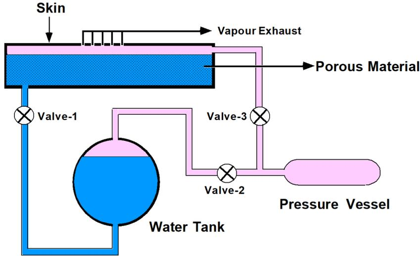
Figure 5-10: Schematic representation of the proposed cooling system.
