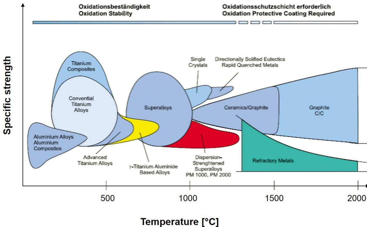
Figure 3-3: Comparison of different types of materials based on their operating temperature and strength (Buursink, 2005).
