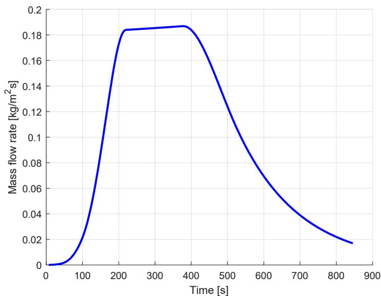
Figure 5-13: Variation of coolant mass flow rate as a function of time (C/C-SiC, cooled with blocking).
