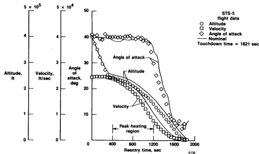
Figure 2-3: STS re-entry flight parameters (Gong et al., 1987).
