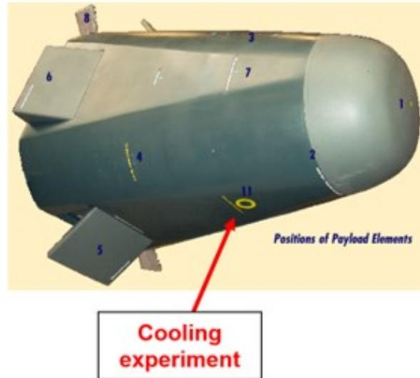
Figure 2-9: Location of the active cooling experiment on the vehicle (Sudmeijer, 2005).
