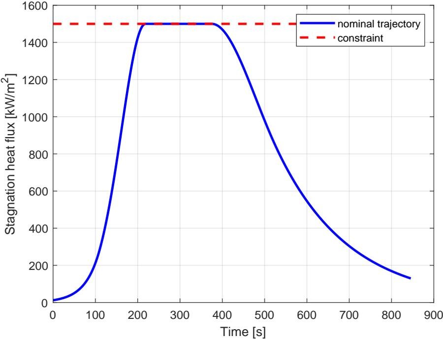
Figure 2-24: Stagnation heat flux profile for nominal trajectory (Nose radius ( $R_N$ ) = 26 mm).
