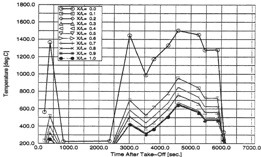
Figure 2-20: Temperature profile on windward centreline of FSS-15 (OAE) (Vollmer, 1992).
