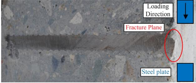
(b) Rebar shape inside concrete block
