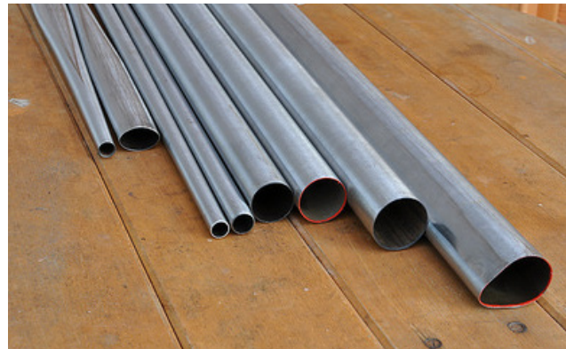
Figure 34 Extruded bicycle tubes
