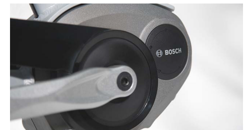
Figure 28 From top to bottom; a. Bafang front-wheel motor Ebike4Delivery, b. Bafang mid-motor, c. Bosch mid-motor
