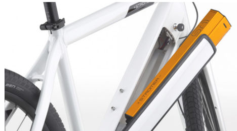
Figure 29 From top to bottom; Integrated and removable battery in frame a. Ebike4Delivery, b. Sparta, and c. Stromer
