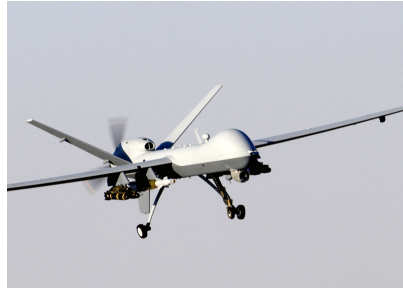
Figure 2.11: MQ-9 Reaper UAV equipped with SAR (Courtesy of U.S. Air Force)
