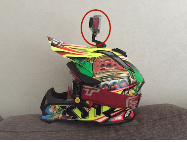
Fig. 2. Placement of the action camera on top of the helmet. The top mount provides a complete view of the rider's movements.
