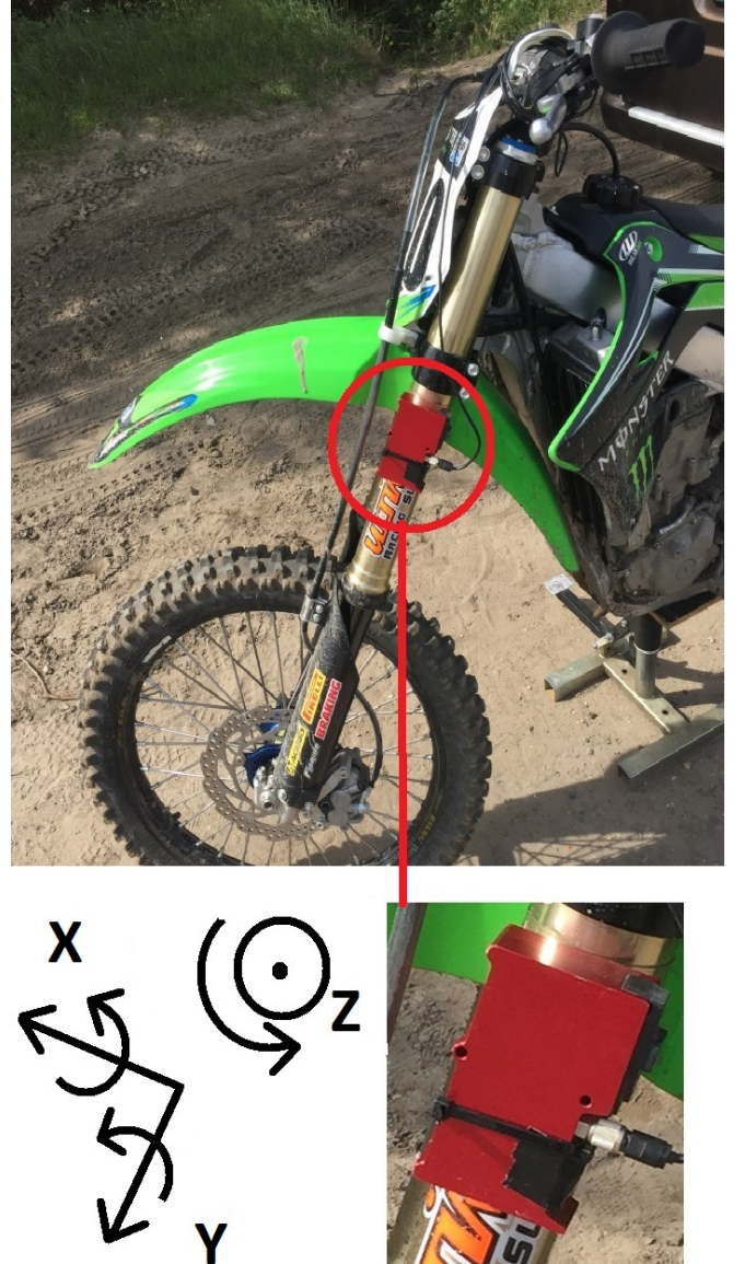
Fig. 1. Placement of the sensor on the motorcycle including the references axis orientation.
