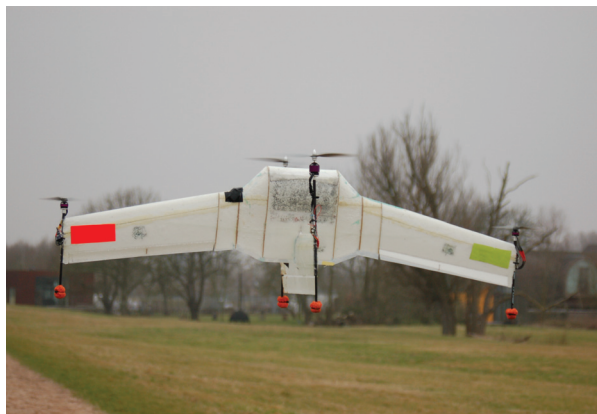
Figure 8: A hovering ATMOV to plant a calibration sensor. When flying larger distances, the wing is rotated 90^\circ .
