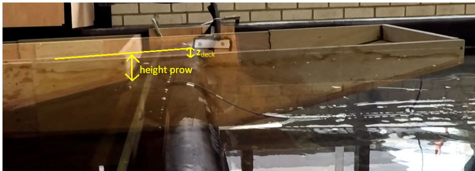
Figure 6.14: displacement measurement ship on weir
