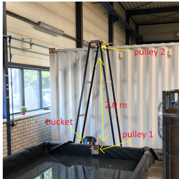
Figure 6.6: tower for fall height
