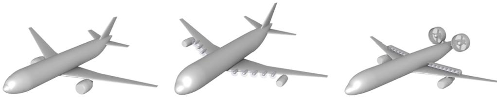
Figure B.3: Example illustration of selected hybrid electric aircraft concepts generated with the *Initiator* [7]
