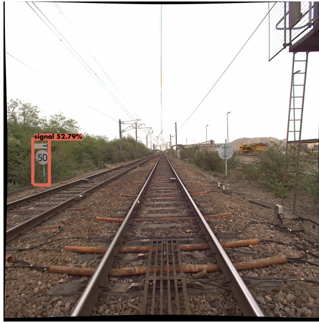
Figure 5.1: False positive (FP) detection of the 2D detector - Confusing a speed limit sign as signal. This lowered the precision of the 2D detector (see Table 4.1). Although the sign appeared in multiple 2D images/frames, only in one frame the 2D detector captured it as a signal.
