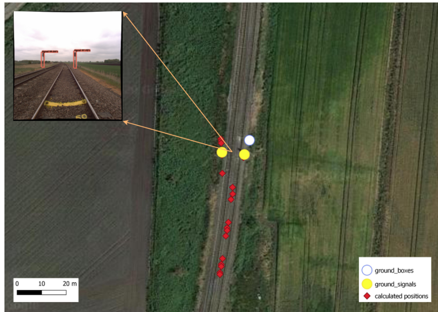
Figure 5.4: Wrong triangulations (red). The model mixed the 2 detected signals as one.
