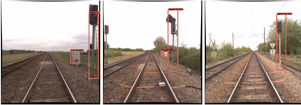
Figure 4.2: Not sufficient performance of the 2D detector regarding the height borders of the bounding boxes.
