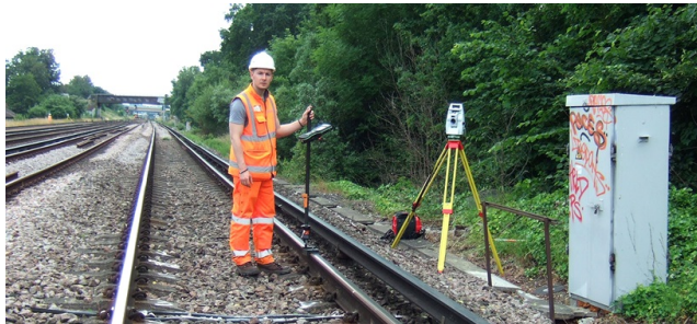
Figure 1.1: Monitoring the railway infrastructure by means of GNSS and leveling. The acquisition of the geo-data made by the physical presence of an inspector (Figure taken from [1]).
