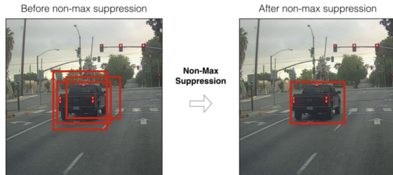
Figure 2.5: Choosing the best bounding box using the non-maximum suppression technique (Figure taken from [6]).
