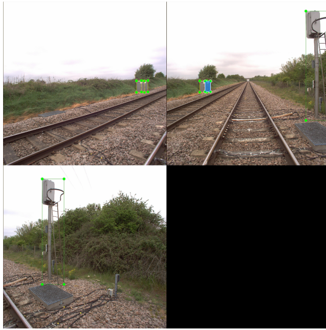
Figure 3.5: Creation of training data - Labeling procedure on raw input data. Top-left: labeled equipment box; Bottom-left: labeled signal; On top right, both objects classes are present.
