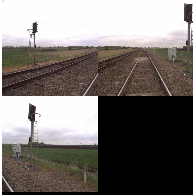
Figure 3.2: Raw 2D imagery data. A tessellation of raw images of the 3 cameras mounted on Fugro's MMS RILA. The dimensions of every individual 2D video frame are 2016x2016 pixels.
