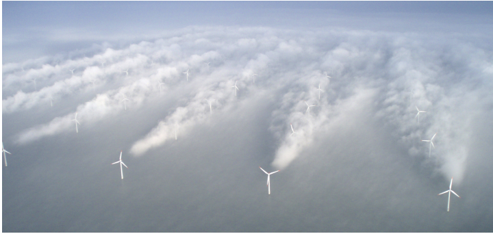
Figure 1.1: Aerial view from the Southeast of wake clouds at Horns Rev on February 12, 2008 (© Vattenfall, Horns Rev 1 owned by Vattenfall. Photographer Christian Steiness)
