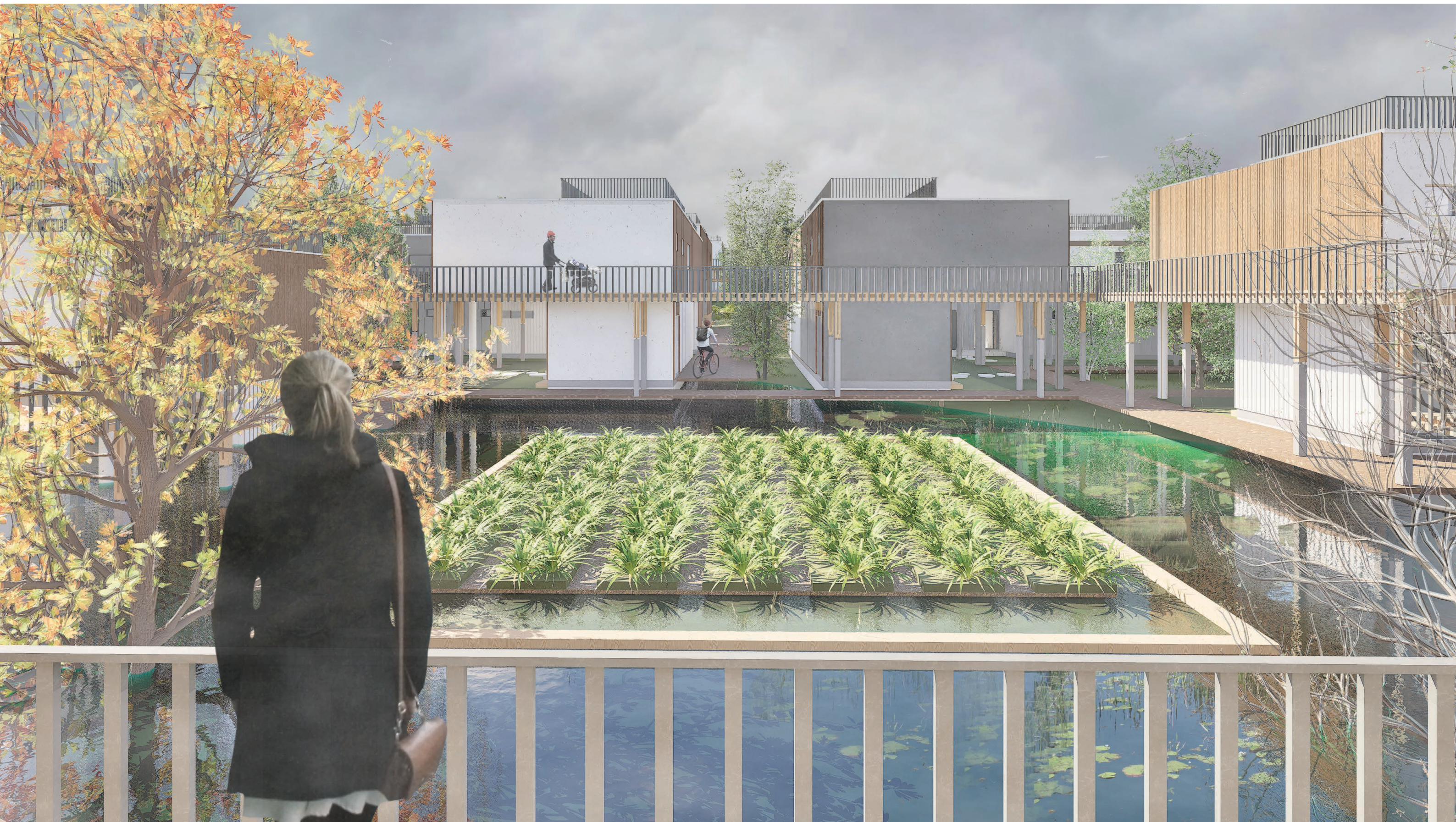
Floating gardens help clean flood water using a combination of natural processes like phytoremediation, biofiltration, and sediment trapping.
