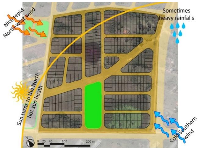
Fig. 5.5 climatically aspects that should be taken in account with a building design
