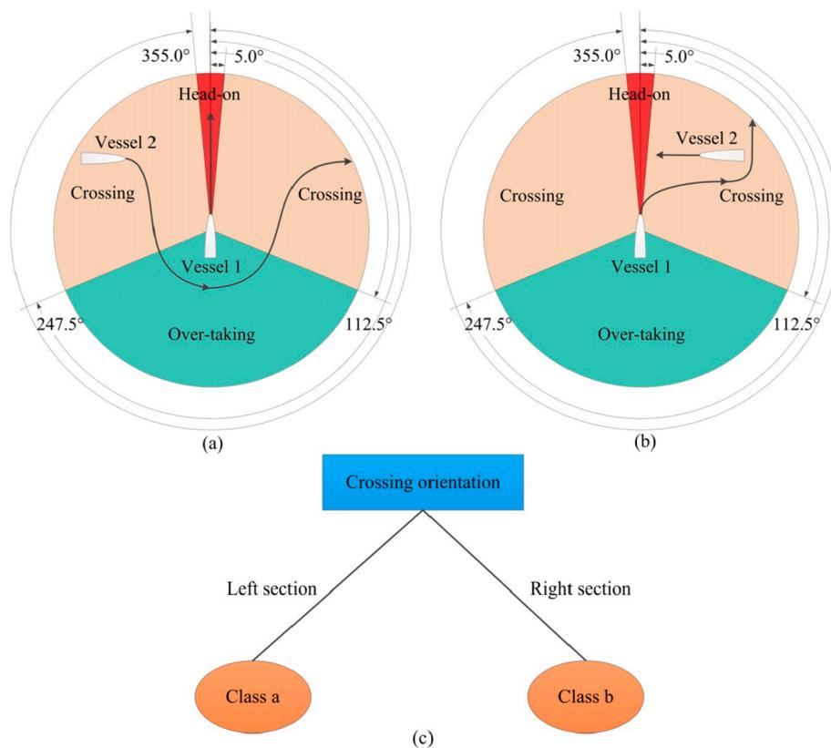
Fig. 1. The collision avoidance operation in the encounter scenario of different crossing situations and the decision tree generated from this case.
