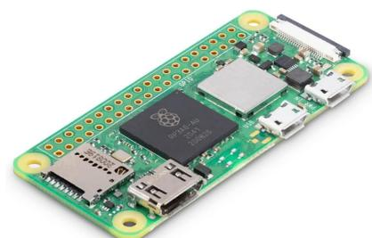
compared to the Odroid XU4 processor used on the 500-gram drone in this project. And an even bigger gap compared to the Jetson xavier nx processor used in the original EGO-planner paper [18]. Figure F.1 shows the Pi zero 2w.
