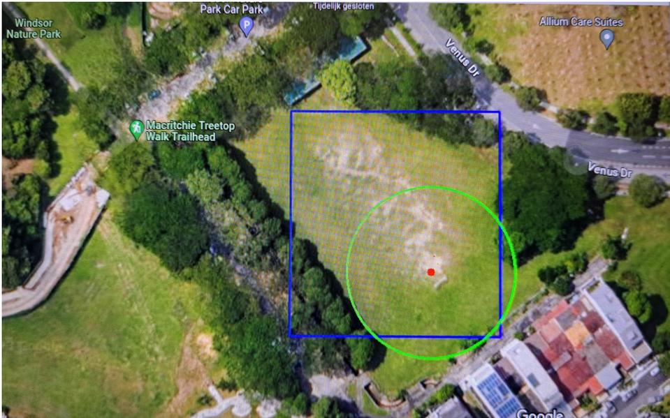
Figure B.8: Alternative created geofencing plotted on satellite image map
