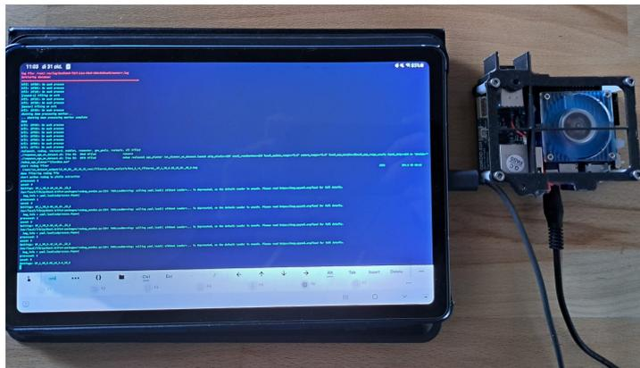
Figure 6.12: Example of running automated simulations on the drone's processor by a tablet with SSH terminal
