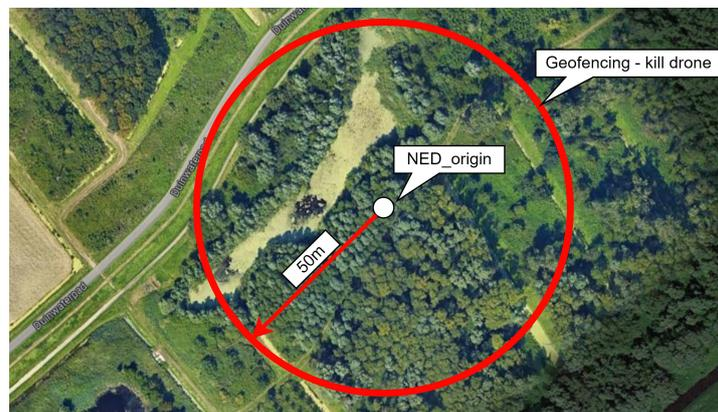
Figure 3.9: Geofencing kill function for redundancy. Example overlay on an image from Google Earth.
