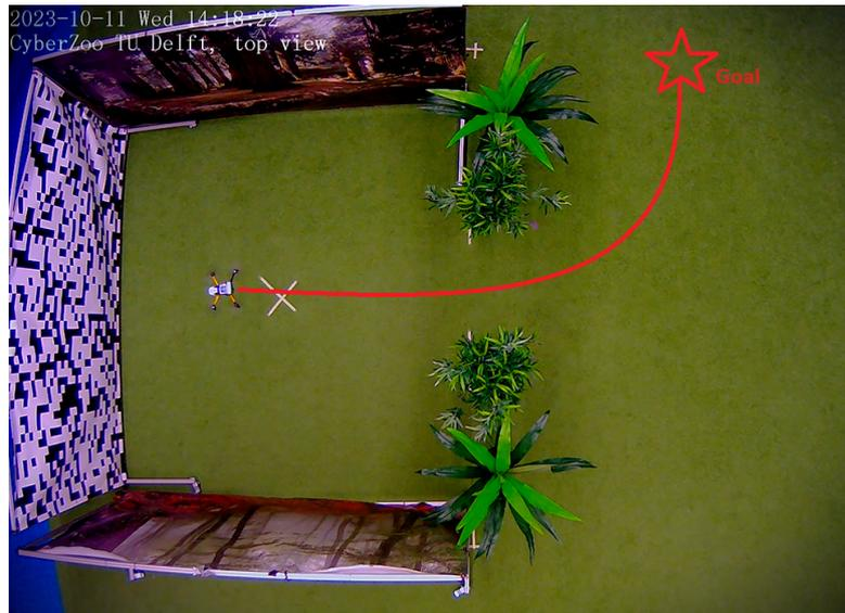
Figure C.1: Varying gap size test (60cm), top-view, in Cyberzoo for indoor dataset
