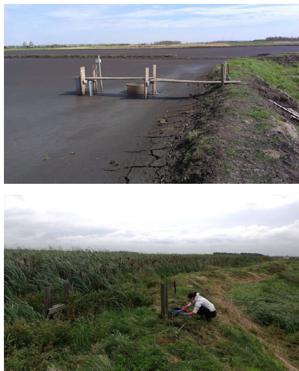
Fig. 2. Depot in June 2014 showing the sampling platform and level gauge (top) and in September 2015, illustrating to the rapid growth and potential dewatering effect of reed (bottom).
