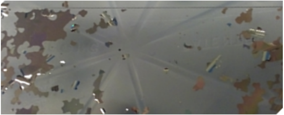
Figure 5.3: Delamination after attempting to dice the wafer into separate devices. Adhesion between glass and silver films is a difficult issue, and is solved by DC magnetron sputtering the silver.
