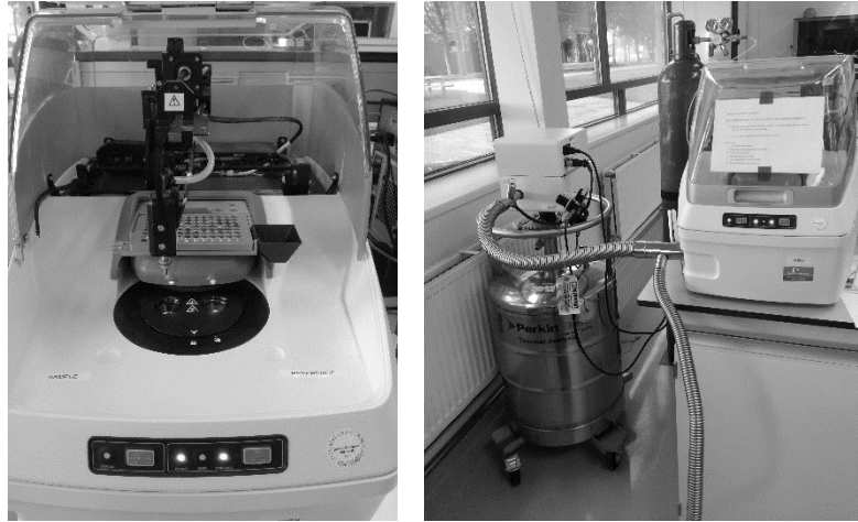
Figure 78: Differential scanning calorimetry auto-sampler (left) and liquid nitrogen cooler (right).
