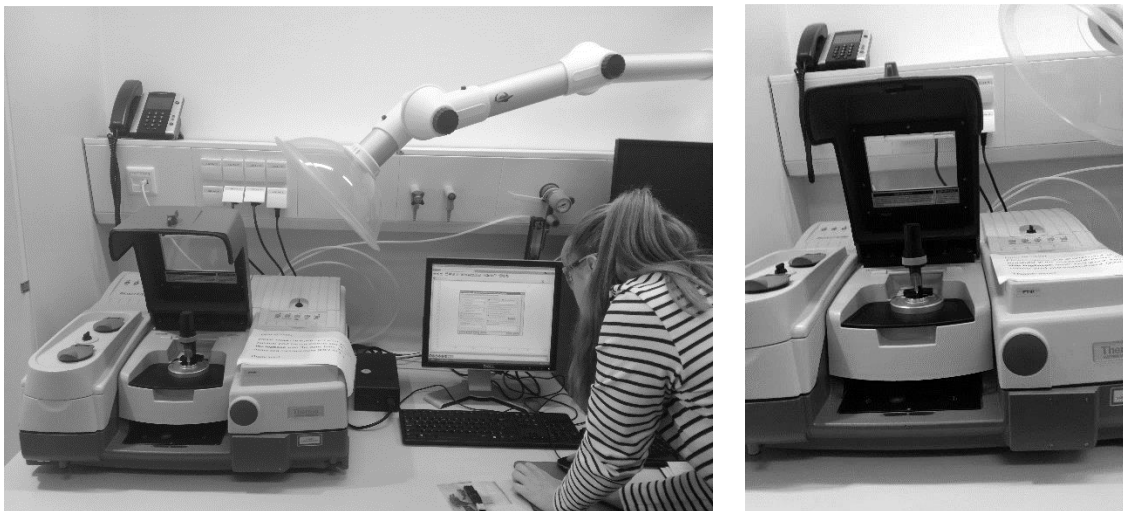
Figure 98: Fourier-transform infrared spectroscopy test setup.
