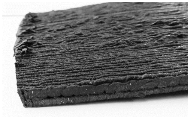
Figure 74: The bent extruded plate of the material PP.
