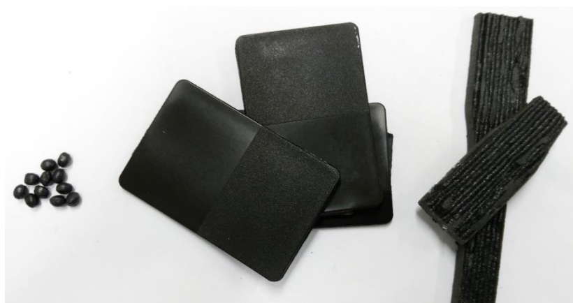
Figure 59: Picture of the raw (left), injection-moulded (middle) and 3D printed PP-based composite.
