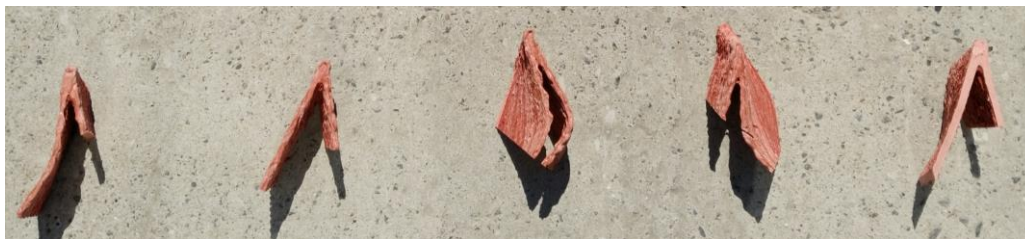
Figure 19: Thermal shock resistance test specimens.
