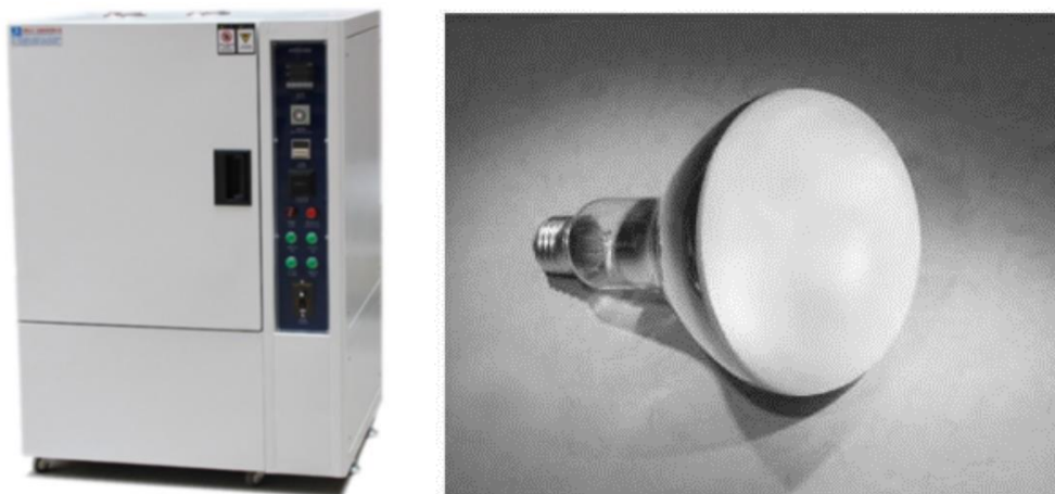
Figure 37: Ultraviolet test chamber (right) and Ultra-Vitalux lamp (left).
