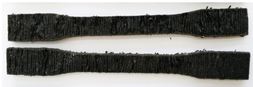
Figure 50: Degraded (upper) and unexposed (lower) tensile transverse sample (840 UV exposure hours).
