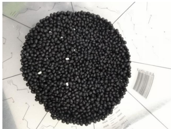
Figure 31: Raw material: PP-pellets (black) with 1% UV stabilisers (white).
