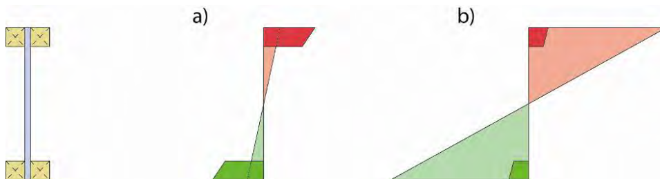
Figure 239: Flexural stress distribution: a) wood PMMA composite, b) wood glass composite
