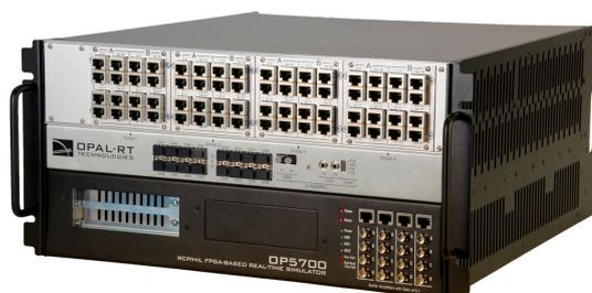
Figure 3.4: OPAL-RT OP5700 Real-Time Simulator [40]
