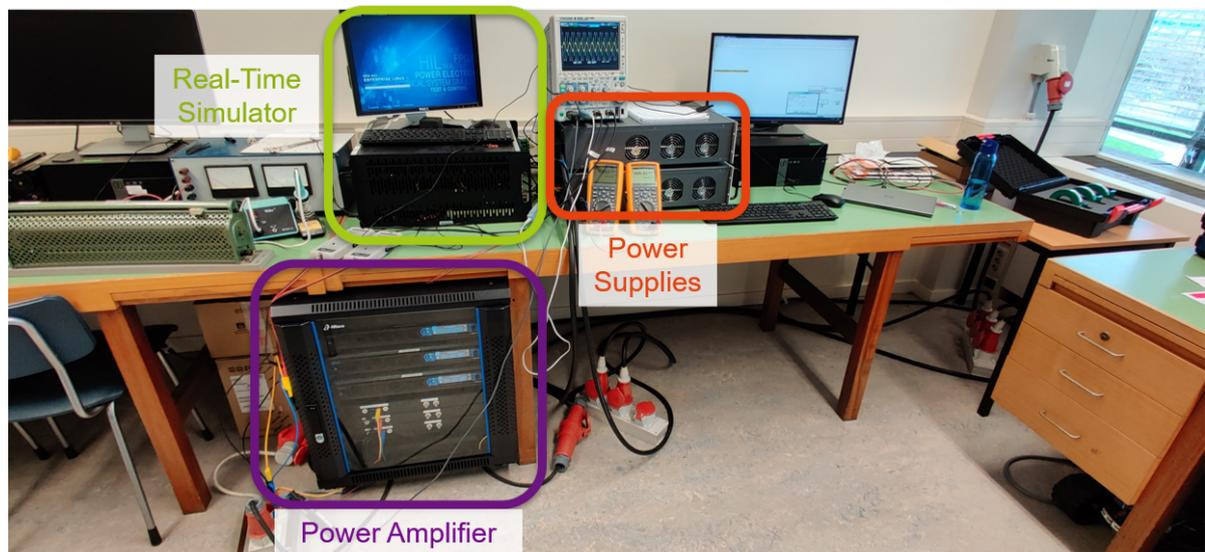
Figure 5.6: Annotated picture of experimental setup. The annotation colors used correspond to the colors of figure 3.2.
