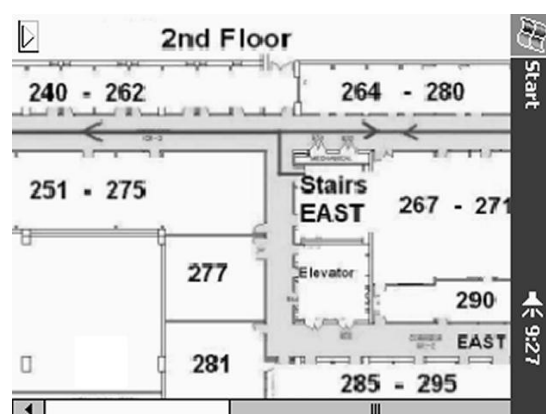
Figure 6-3. Floor overview on the PDA (rotated 90 degrees). The gray area represents a hallway, the dark gray line indicates the route.
