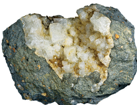
Figure 1.1: Natural zeolite Chabazite [55]. Zeolites have a crystal-like appearance on the inside. The size of the zeolite in the picture is 72x54x30 mm.
