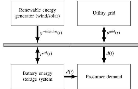
Figure 1: Power flow diagram by Norbu et al. (2021, p. 5) depicting the prosumer model.
