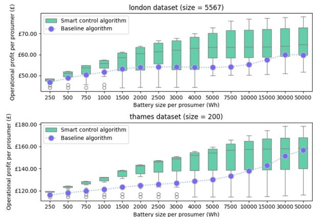
Figure 3: High-level comparison between operational profits of the baseline algorithm and smart algorithm for the average prosumer using various battery sizes and lookahead amounts represented in boxplots, following the experiment described in subsection 4.2.
