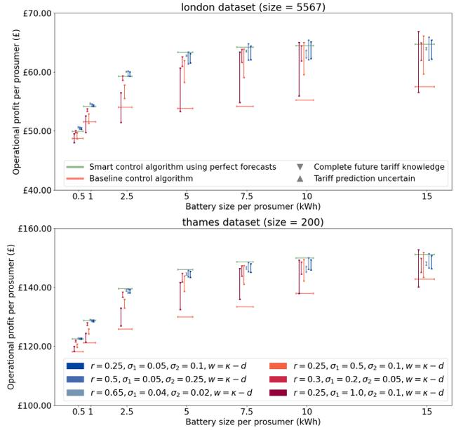
Figure 8: High-level comparison between operational profits of the baseline algorithm and smart algorithm for the average prosumer using various battery sizes and lookahead amounts with uncertain forecasts based on converging and diverging margins.
