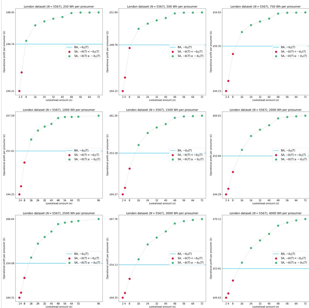
Figure 10: Overview of operational profits per prosumer for the baseline- and smart control algorithm using various sizes for the lookahead window ( $\kappa$ ) and various sizes for the battery per prosumer ( $\omega/N$ ) on original historical data of London (part 1).
