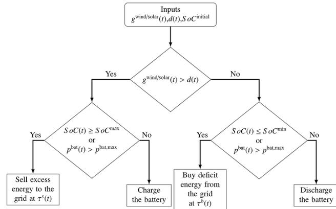
Figure 2: Flowchart of heuristic-based battery control algorithm strategy by Norbu et al. (2021, p. 7).
