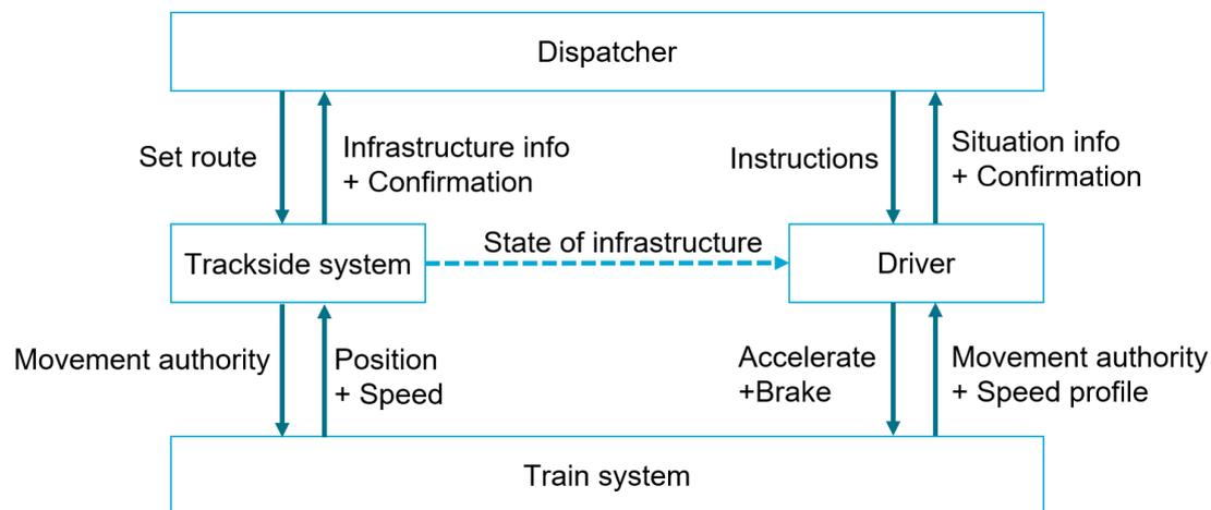
Figure 15: General control structure that can be used to base a specific user process control structure on
