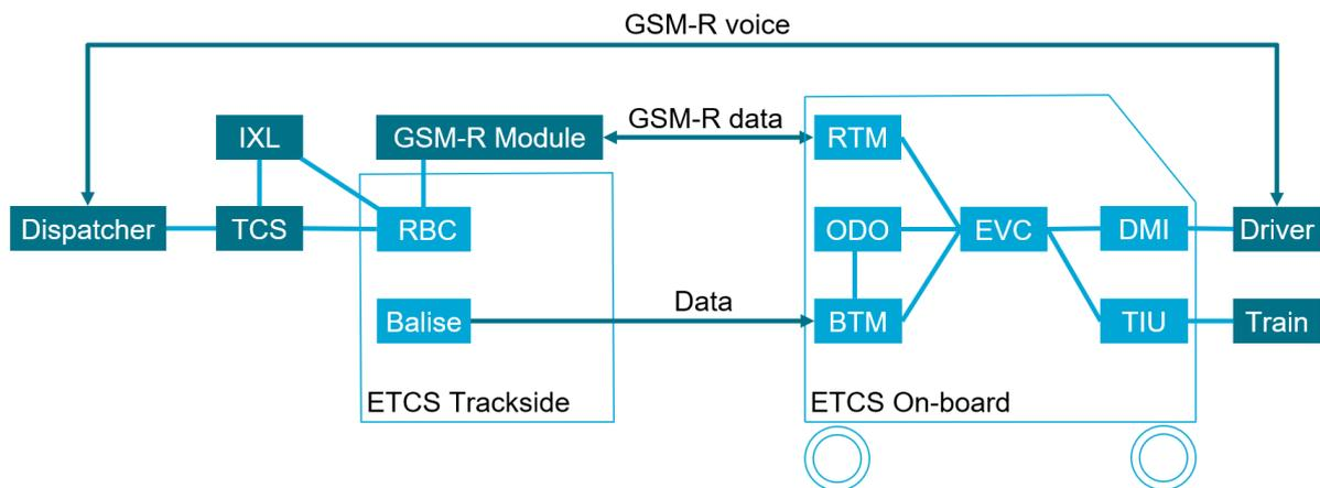
Figure 7: ERTMS/ETCS level 2 architecture model
