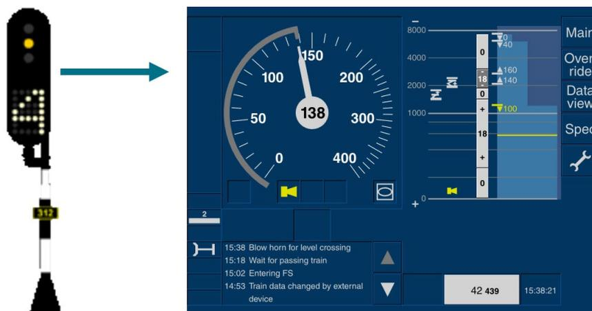
Figure 8: From light signalling along the track (left) to in-cab signalling with a driver machine interface (right) (de Vries, 2016).
