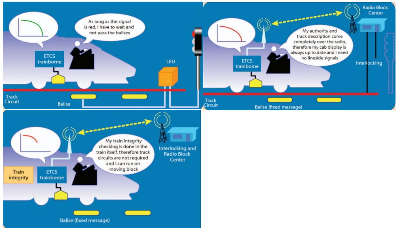
Figure 6: Level 1: left up. Level 2: Right up. Level 3: left down (Unife, 2021b)
