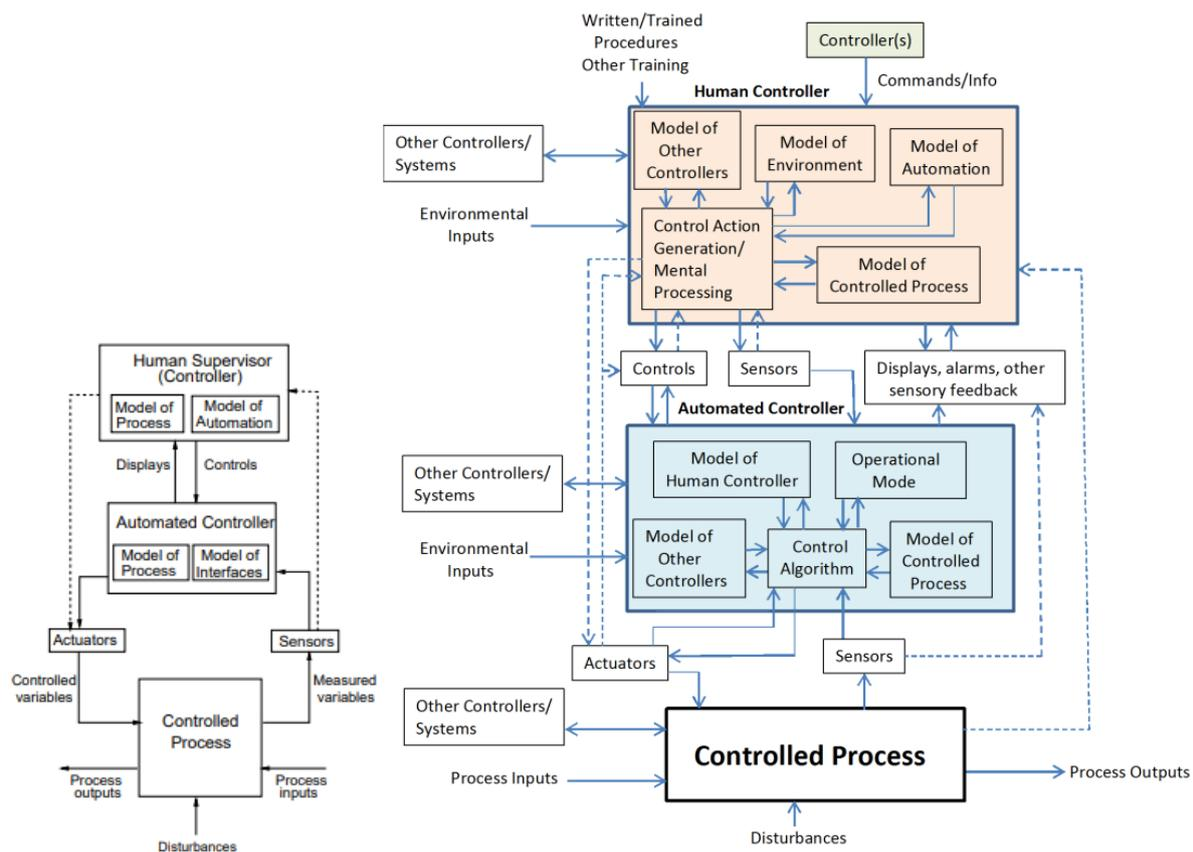
Figure 28: Two general control structures with human controller and automated controller. Left (Leveson 2004), Right (Leveson, 2018).
