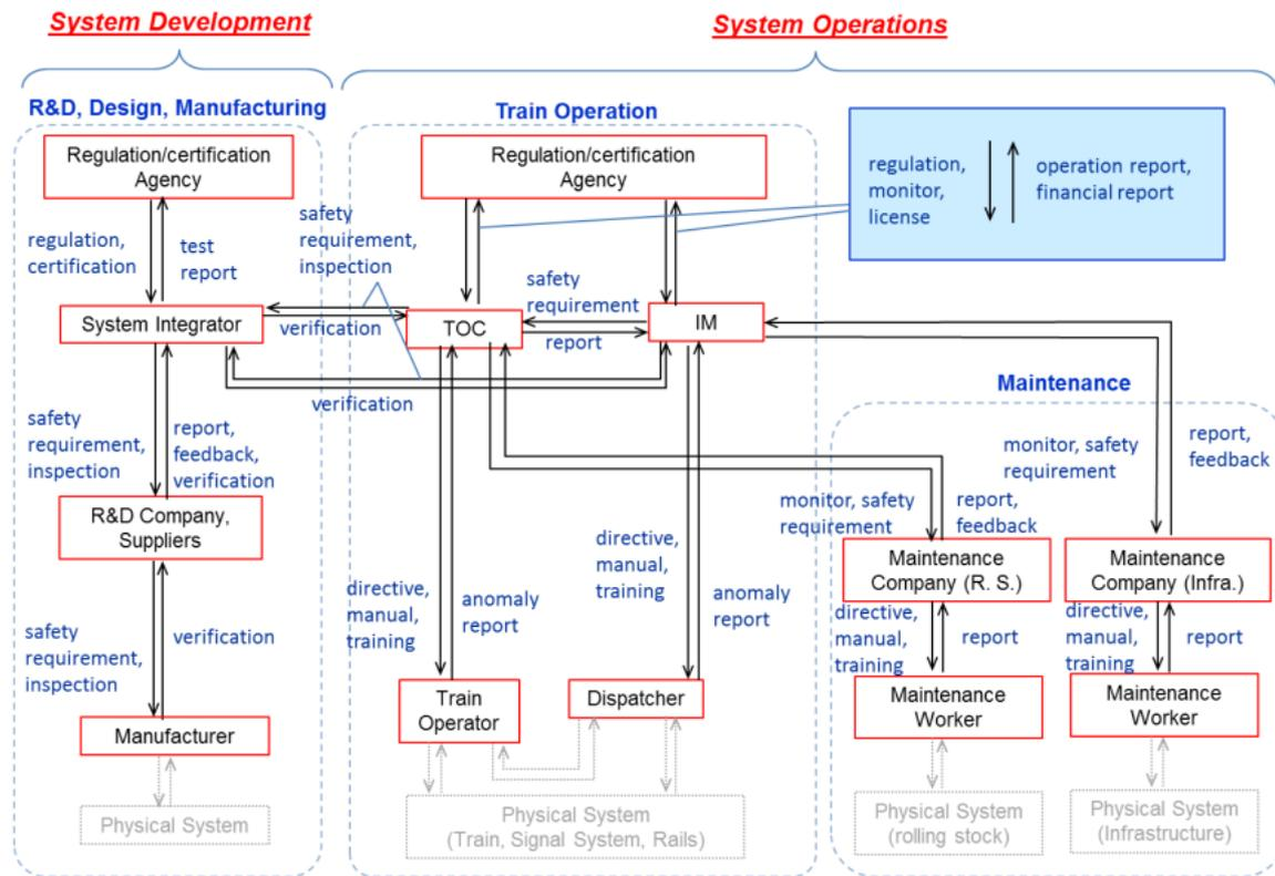
Figure 39: Safety control structure of a generic highspeed rail system (Kawakami, 2014).
