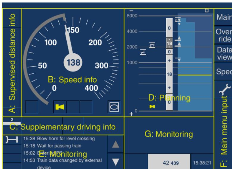
Figure 9: Example of a Driver Machine Interface with the different sections highlighted in yellow (de Vries, 2016).
