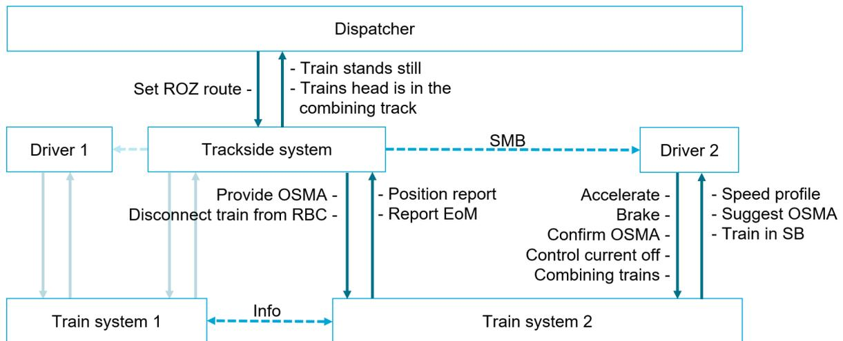
Figure 16: Control structure for user process 48
