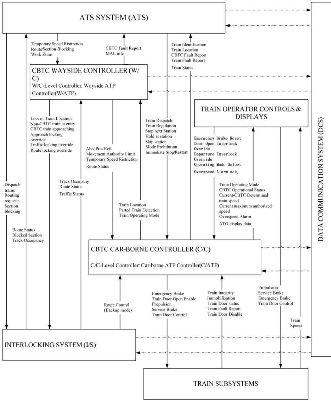
Figure 38: Control structure of a communication based train control system (Dong, 2012).
