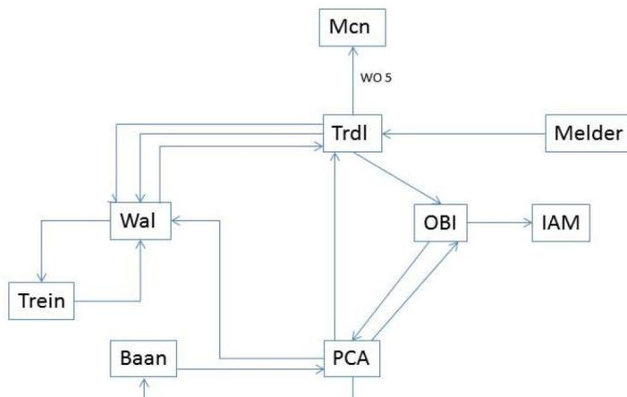
Figure 40: Control structure of user process 47: 'setting a temporary speed limit' (ProRail, 2022b).
