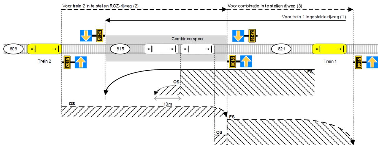
Figure 14: User process 48 example illustration: Combining two trains arriving from opposite directions with movement authority (ProRail, 2022c).
