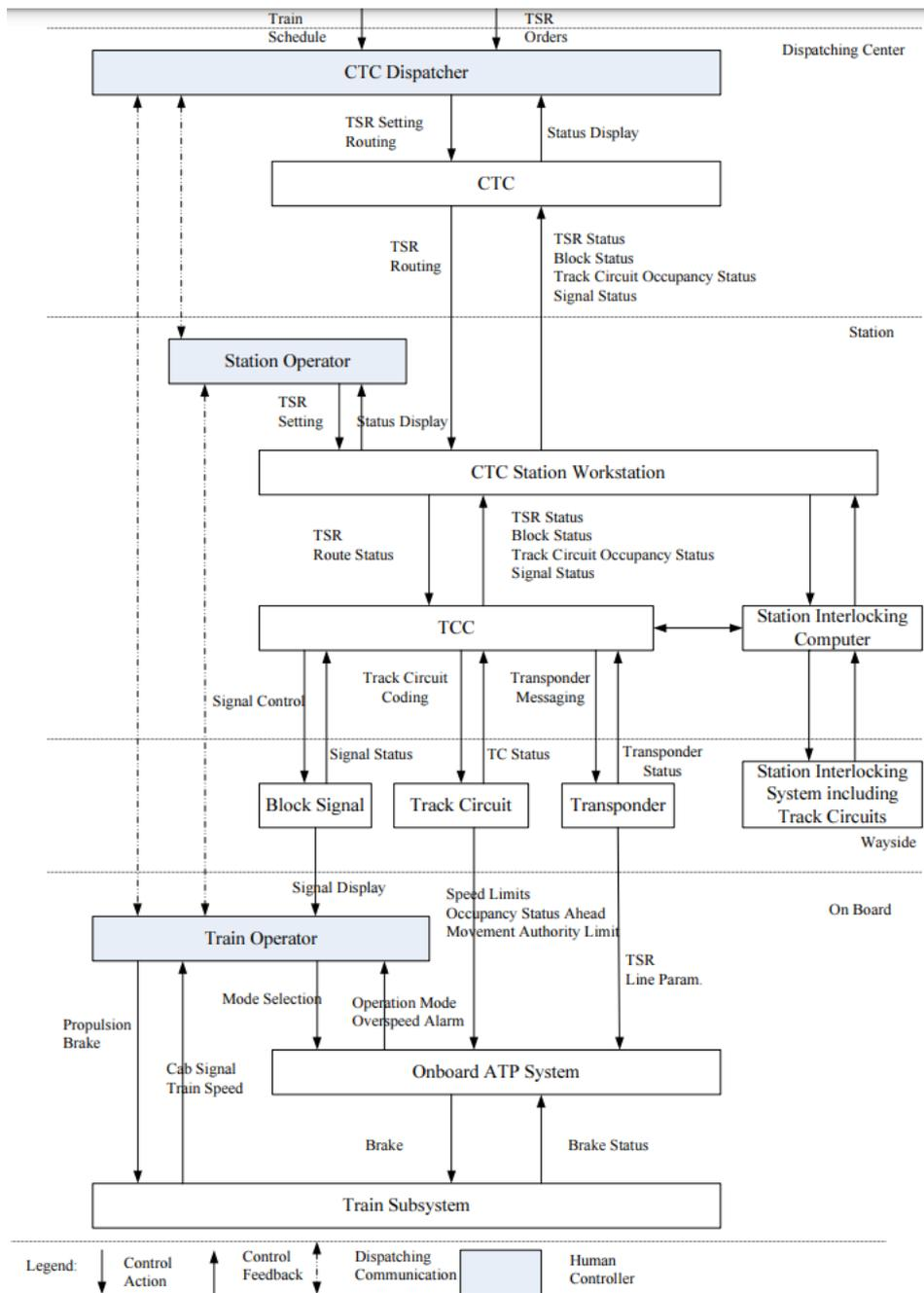
Figure 37: Control structure, to prevent collision between trains (Dong, 2012).
