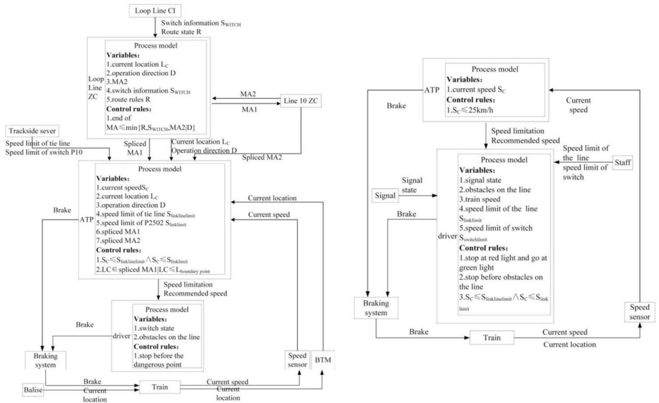
Figure 31: left: train control structure in communications-based train control mode. Right: train control structure in restriction mode. (Li et al., 2021)
