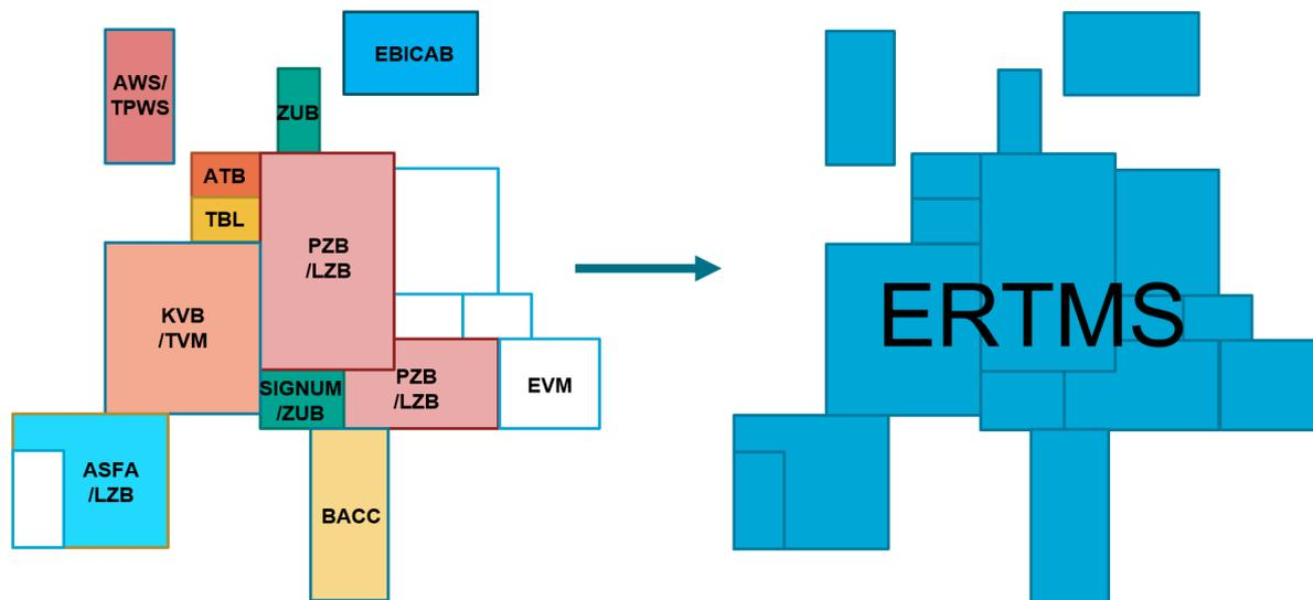
Figure 1: Simplified figure of the transition from the different national automatic train protection systems to a single European railway system (redrawn from ERA, 2017)
