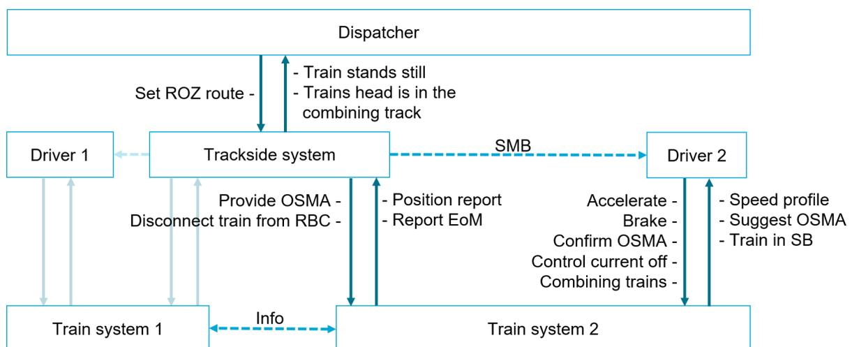
Figure: Control structure of the procedure for combining two train that arrive from opposite directions.
