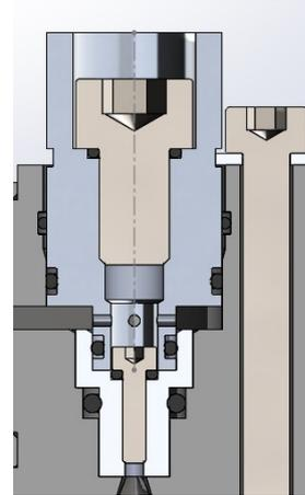
Fig. 55: Section view of the hydraulic valve
