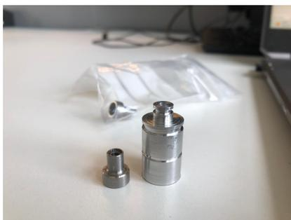
Fig. 39: Valve parts after manufacturing
