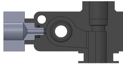
Fig. 47: Section view of the designed pressure sensor fit
