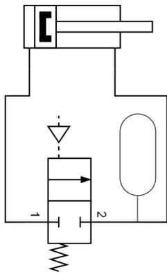
Fig. 54: Hydraulic circuit of the second concept with one 2/2 valve coupled to the cylinder head and the cylinder foot.
