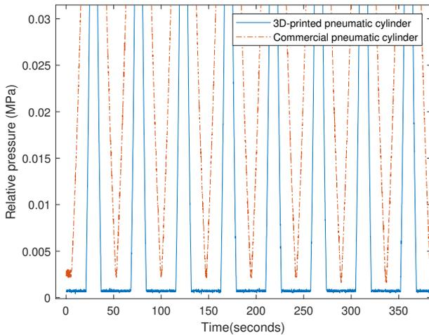
Fig. 49: Plot of the preliminary dynamic leakage test of the cylinder head with self generated pressure
