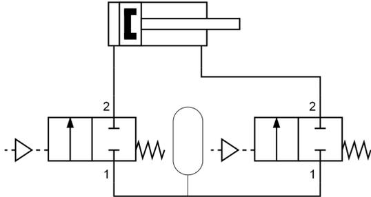
Fig. 53: Hydraulic circuit of the first concept with two 2/2 valves connected to the cylinder head and cylinder foot.
