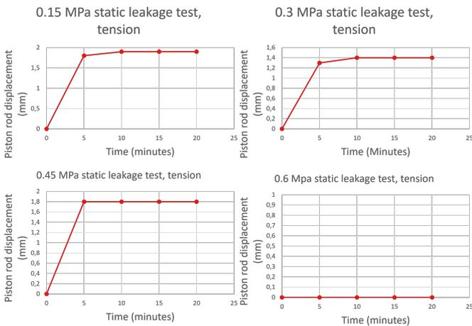
Fig. 46: Results of the weight test for tension at different weights
