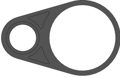
Fig. 8: Section view of hydraulic tube with accumulator tube and connecting triangular cavities
