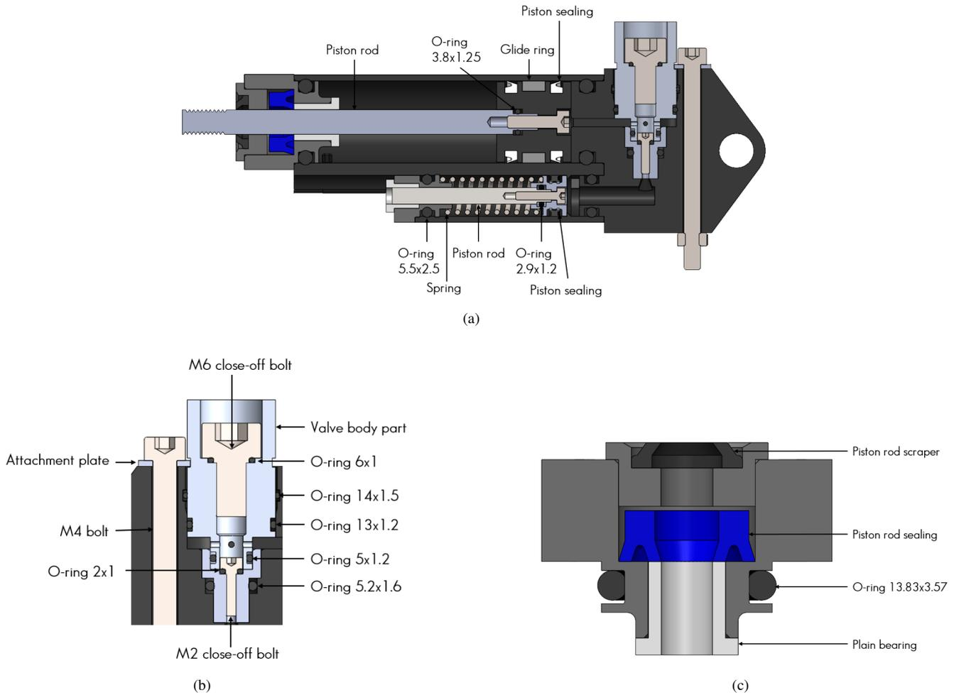
Fig. 7: (a) Section view of the 3D-printed hydraulic cylinder with annotations of the piston rod assembly and the accumulator assembly (b) Section view of the valve assembly with annotations of the different valve parts (c) Section view of the cylinder head assembly with annotations of the different seals and parts.
