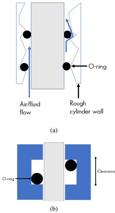
Fig. 18: (a) Explanation of the resettling of an O-ring encountering rough cylinder walls. As can be seen the O-ring settles differently at different rough point leaving passageways for the air. (b) Explanation of the resettling of an O-ring in a high clearance seating. The O-ring is able to move into a diagonal configuration leaving space between the part and the O-ring.
