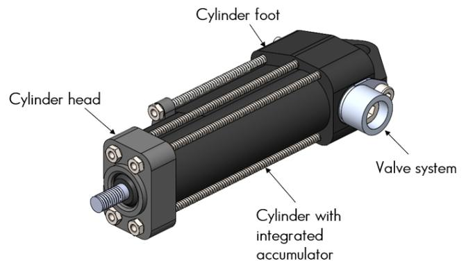
Fig. 6: CAD-model of the 3D-printed hydraulic cylinder with annotation of the main components.
