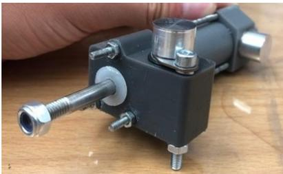
Fig. 42: Picture of the manufactured first iteration of the 3D-printed pneumatic cylinder
