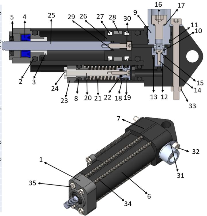
Fig. 58: Bill of materials with annotations of the parts in the section view and the isometric view.
