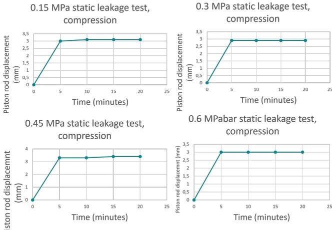
Fig. 45: Results of the weight test for compression at different weights
