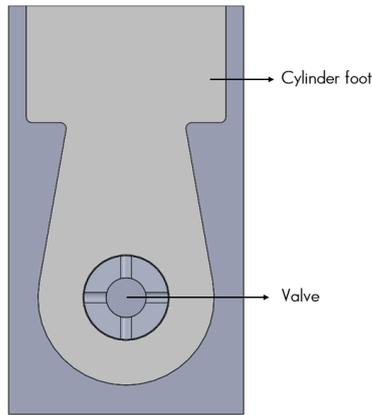
Fig. 30: Section view of the vertical orientation concept in the cylinder foot
