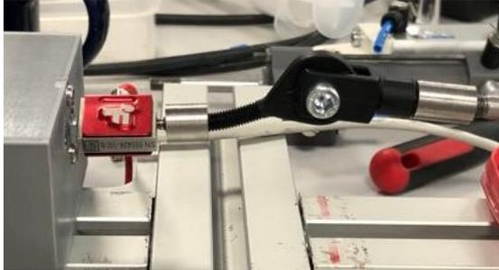
Fig. 20: An exaggerated view of the reaction moment that the force sensor coupling can exert on the force sensor
