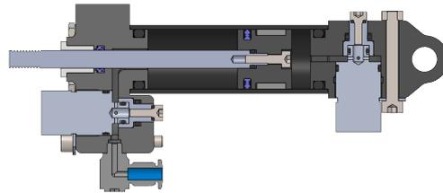
Fig. 52: Section view of the final design of the integrated pneumatic cylinder
