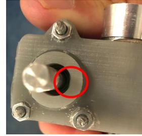
Fig. 51: Close up of the cylinder head, the red circle indicates the unroundness of the plain bearing seating and piston rod seal seating
