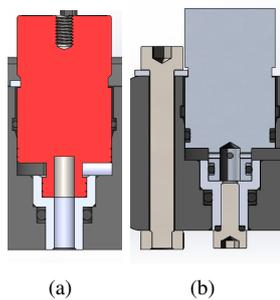
Fig. 38: (a) section view of the Parker-Hannifin valve (b) section view of the designed manual valve assembly
