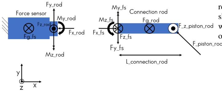
Fig. 22: Free body diagram of the coupling between force sensor and connection rod of the universal joint when there is misalignment. The end of the connection rod is coupled to a universal joint which is coupled to the piston rod. The FBD seen from a top view.
