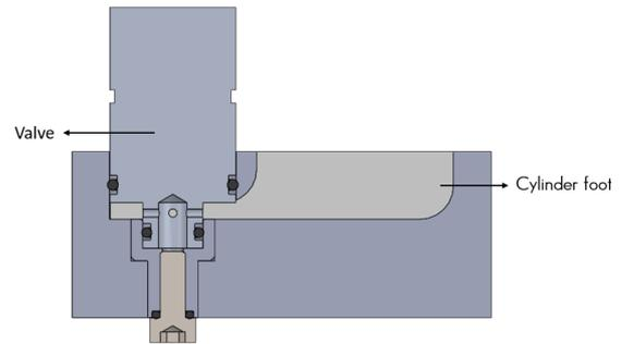
Fig. 33: Section view of the parallel horizontal orientation concept in the cylinder foot
