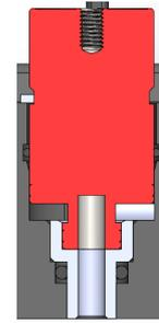
Fig. 37: Section view of the valve seating with commercial valve
