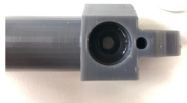
Fig. 40: Picture of one of the first printed parts with a lot of damages after support removal in the cavity
