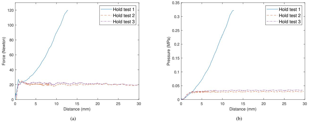
Fig. 17: (a) Three hold tests with distance and force measured until the holding point. (b) Three hold tests with distance and internal pressure generation measured.
