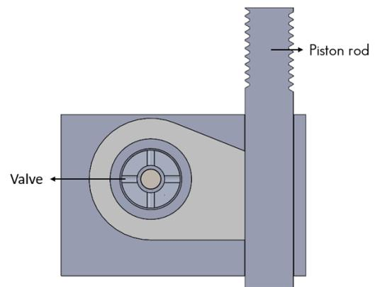
Fig. 34: Section view of the parallel vertical orientation concept in the cylinder head
