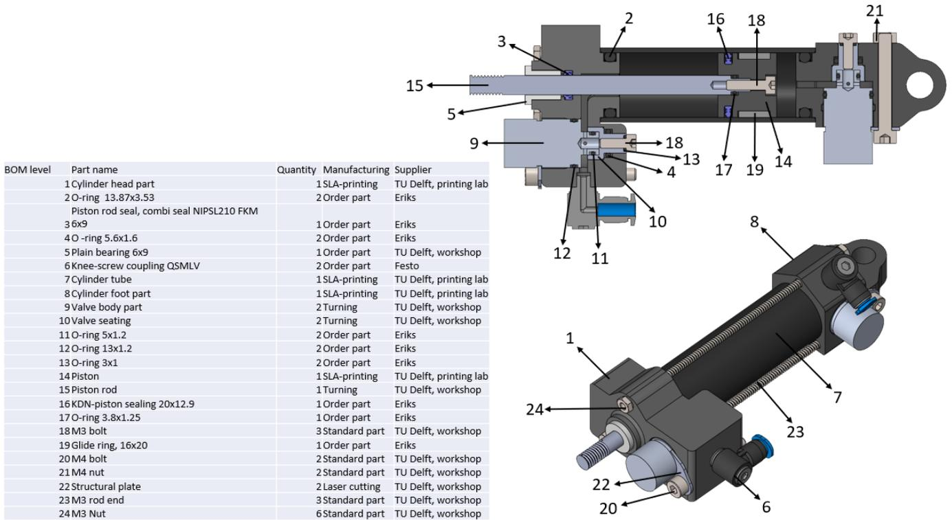
Fig. 57: Bill of materials with annotations of the parts in the section view and the isometric view.
