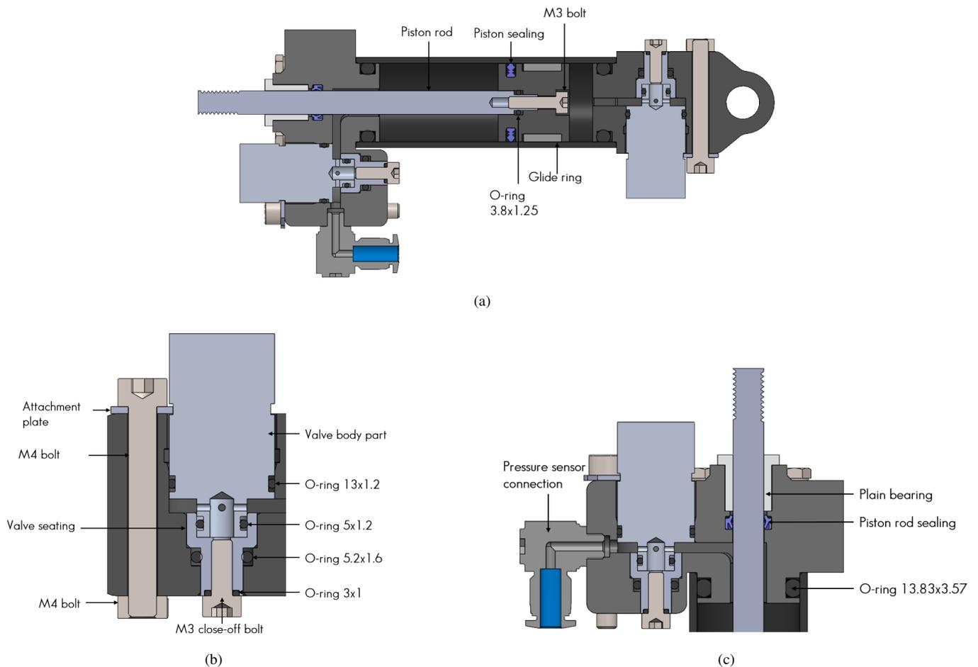
Fig. 3: (a) Section view of the 3D-printed pneumatic cylinder with annotations of the piston rod assembly. (b) Section view of the valve and valve seating assembly. (c) Section view of the cylinder head with annotation of functional parts
