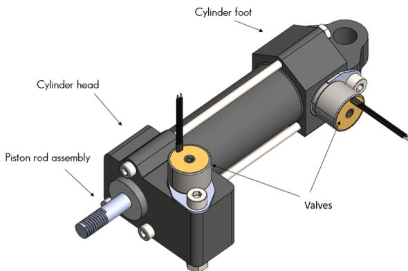
Fig. 36: Isometric view of the total assembly with annotation of the main components
