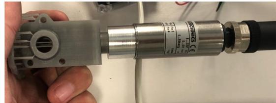
Fig. 48: The manufactured and assembled pressure sensor connection
