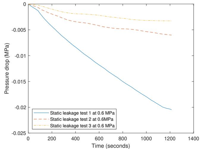
Fig. 19: Pressure drop diagram for three different static leakage tests in the cylinder head at  $0.6\ \text{MPa}$ .
