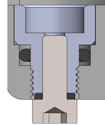
Fig. 23: Section view of the new design for the valve seating with outer thread connected in a tapped hole in the cylinder head or foot.
