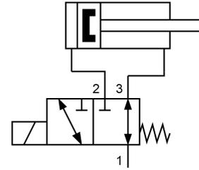
Fig. 25: Pneumatic circuit of the second concept, a 3/2 valve connected to the cylinder head and foot
