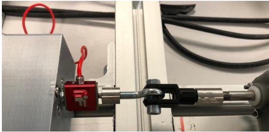
Fig. 50: Test rig set-up for the pulling test with a hook that can only pull and not push the cylinder
