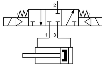
Fig. 26: Pneumatic circuit of the third concept, 3/3 valve connected to the cylinder head and foot.
