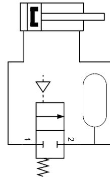
Fig. 5: Hydraulic circuit of the 3D-printed hydraulic cylinder. The two hydraulic chambers are connected by a 2/2 valve and accumulator
