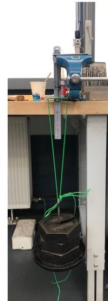
Fig. 44: Test set up for weight testing for the cylinder head
