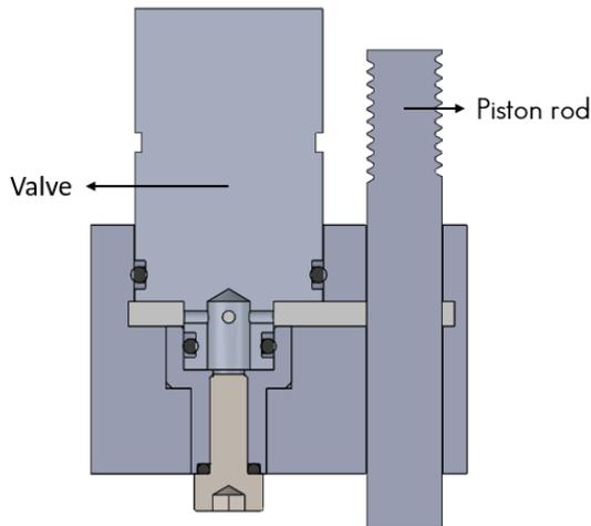
Fig. 35: Section view of the parallel horizontal orientation concept in the cylinder head
