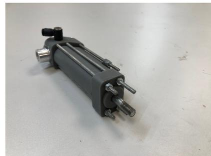
Fig. 9: The assembled 3D-printed hydraulic cylinder ready for testing
