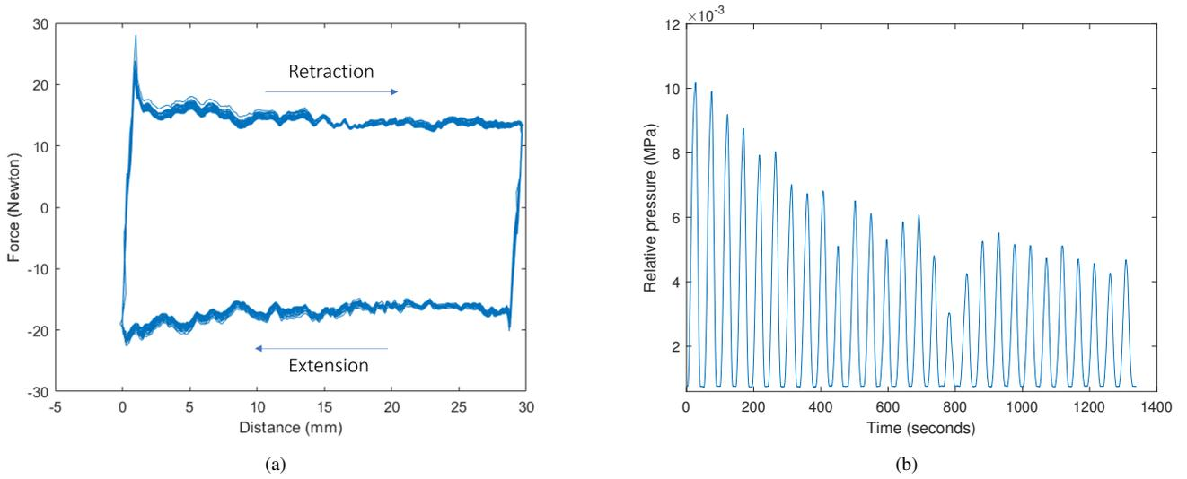
Fig. 16: (a) Hysteresis plot of the hydraulic cylinder in open valve mode, increasing distance corresponds with a retracting or inward movement. Decreasing distance corresponds with a extension or outward motion. (b) Internal leakage plot of the hydraulic cylinder measured for 20 minutes during a dynamic test.
