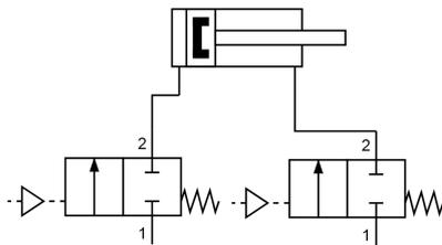
Fig. 24: Pneumatic circuit of the first concept, two 2/2 valves connected to the cylinder head and foot
