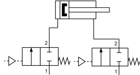
Fig. 1: Pneumatic circuit of the 3D-printed cylinder. To both cylinder ends a two way two-position valve is connected.
