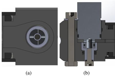
Fig. 28: (a) Top view of the droplet connection concept. (b) Side view of the droplet connection concept.
