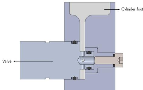
Fig. 31: Section view of the horizontal orientation concept in the cylinder foot
