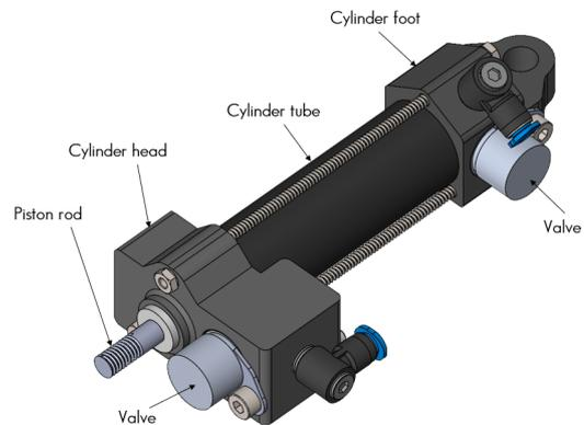
Fig. 2: CAD view of the designed 3D-printed pneumatic cylinder with annotation of the main components
