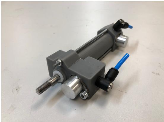
Fig. 4: Manufactured 3D-printed cylinder ready for testing.
