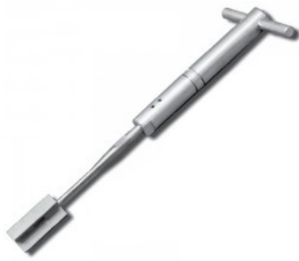
(a) Portable shear vane tester
