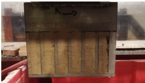
Figure 5.7: Side of the Alpha Plough after test
