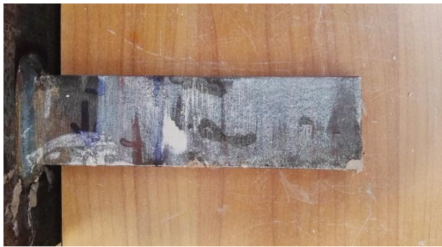
Left side of plough after trenching
