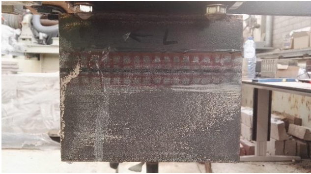
Left side of plough after trenching
