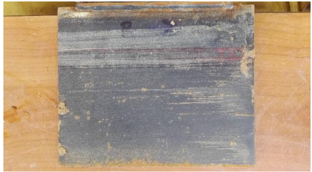
Right side of plough after trenching
