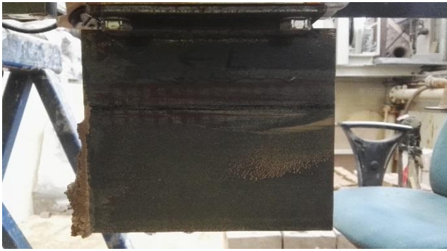
Left side of plough after trenching
