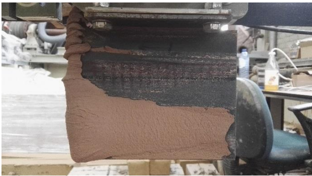
Left side of plough after trenching
