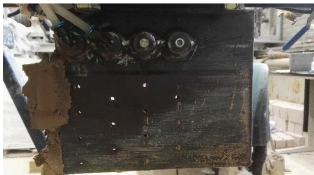
Left side of plough after trenching
