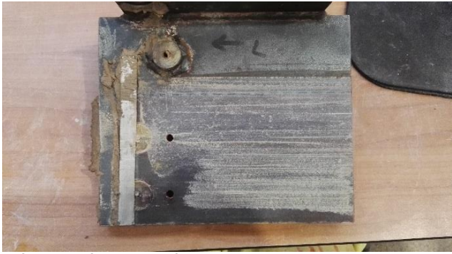
Left side of plough after trenching
