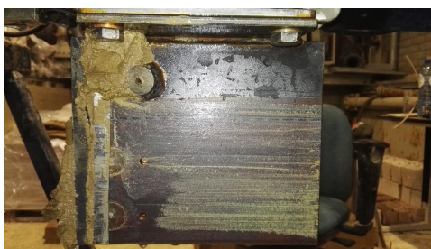
Figure 5.9: Side of the Bravo Plough with 2mm strips after test
