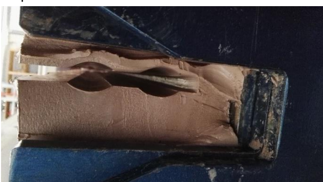
Cross section at the start of the clay container
