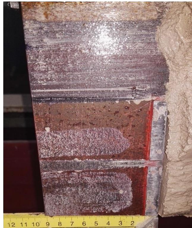
Left side of plough after trenching
