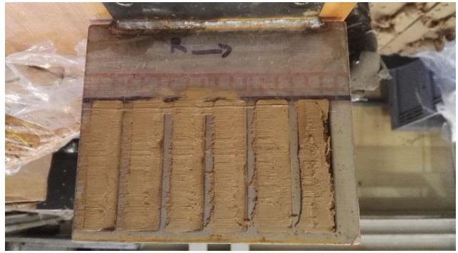
Right side of plough after trenching
