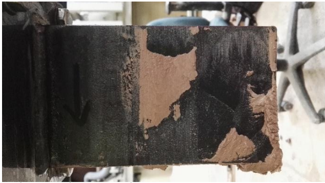
Left side of plough after trenching
