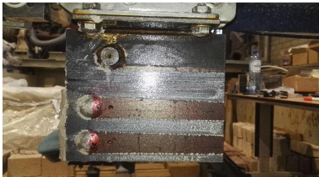
Left side of plough after trenching
