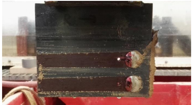
Right side of plough after trenching
