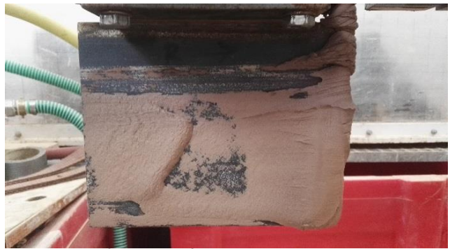
Right side of plough after trenching
