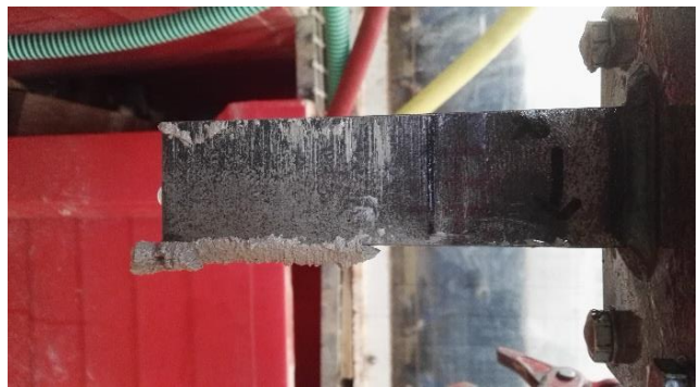
Right side of plough after trenching
