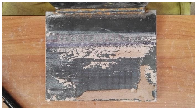
Right side of plough after trenching
