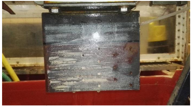
Right side of plough after trenching
